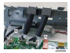
10. Connect the two modular harnesses [A] (TEL), [B] (LINE1) to the FCU.
