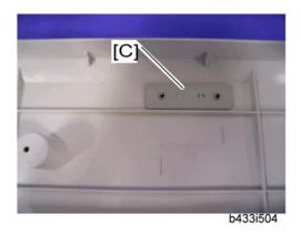
3. Attach the hand set support bracket [C] inside the scanner left cover.
