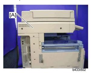
1. Remove the scanner left cover [A] ( \*\* x 2).
