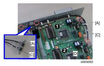
7. Attach the socket of harness [A] (LINE2) and the socket of harness [C] (LINE3) to the modular bracket for SG3.
