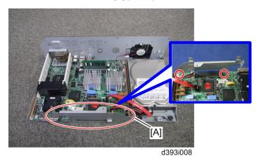
2. Attach the FCU I/F board bracket [A] to the controller board (  $\mbeta$  x 2).
