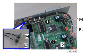
$7. \ \ \, \text{Attach the socket of harness [A] (LINE2) and the socket of harness [C] (LINE3) to the modular bracket}$
