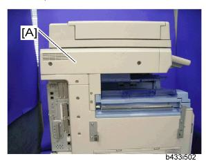
1. Remove the scanner left cover [A] (  $\mbox{\ensuremath{\beta}}\mbox{ x 2)}.$
