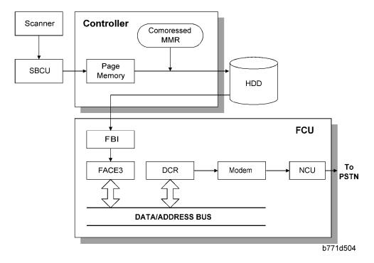
The base copier's scanner scans the original at the selected resolution. The IPU video processes the data and transfers it to the controller board.
