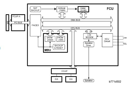
The FCU (Facsimile Control Unit) controls fax communications, the video interface to the base copier's engine, and all the fax options.
