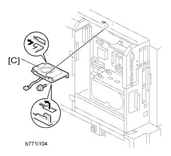
3. Install the speaker [C] to the controller box ( $\mathcal{F}$ x 1).
