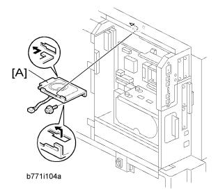
1. Install the speaker [A] on the controller box if the fax unit has not been installed ( $\mathscr{F} \times 1$ ).
