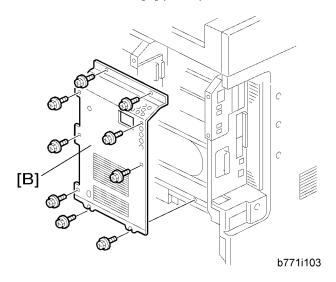
2. Remove the controller box cover [B] (  $\widehat{\mathscr{E}}$  x 9).
