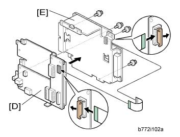
3. Attach the SG3 interface unit [D] to the rear side of the fax unit [E] (  $\mbox{\ensuremath{\beta}}$  x 4).
