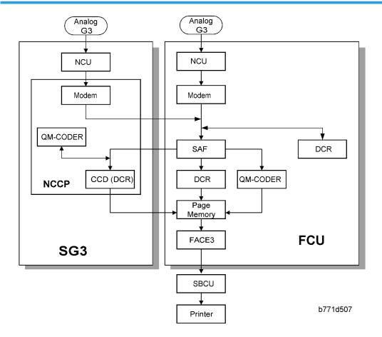
First, the FCU stores the incoming data from either an analog line to the SAF memory. (The data goes to the FACE3 at the same time, and is checked for error lines/frames.)
