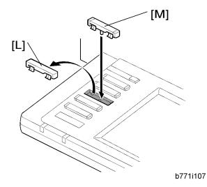
15. Replace the third key-slot cover [L] with the fax key [M].
