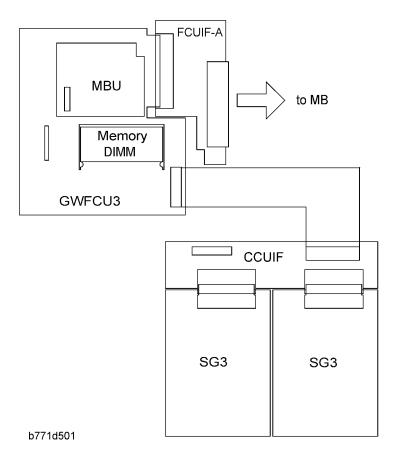
The basic fax unit consists of two PCBs: an FCU and an MBU.
