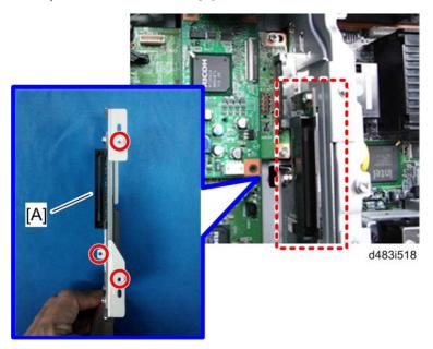
6. Attach the relay board [A] ( x 3).
