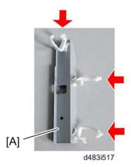
8. Attach the three clamps to the bracket [A].
