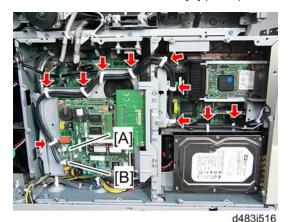
12. Connect the two modular harnesses [A] [B] to the FCU ( $\frak{\Box} x$  12).
