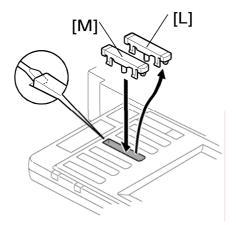
19. Replace the third key-slot cover [L] with the fax key [M].
