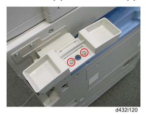
8. Attach the cradle to the handset bracket (  $\nearrow$  x 2: M3x8).
