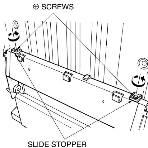
Figure 6-24. Removal of the Paper Exit Stopper Plate
