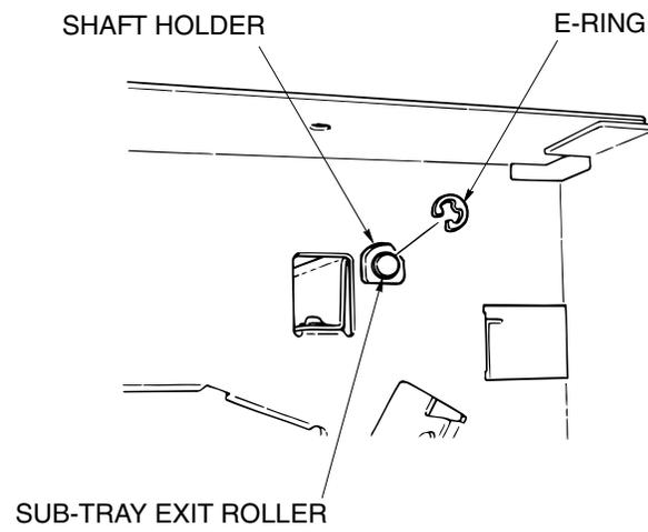
*Figure 6-10. Removal of the Sub-tray Paper Exit Roller*
