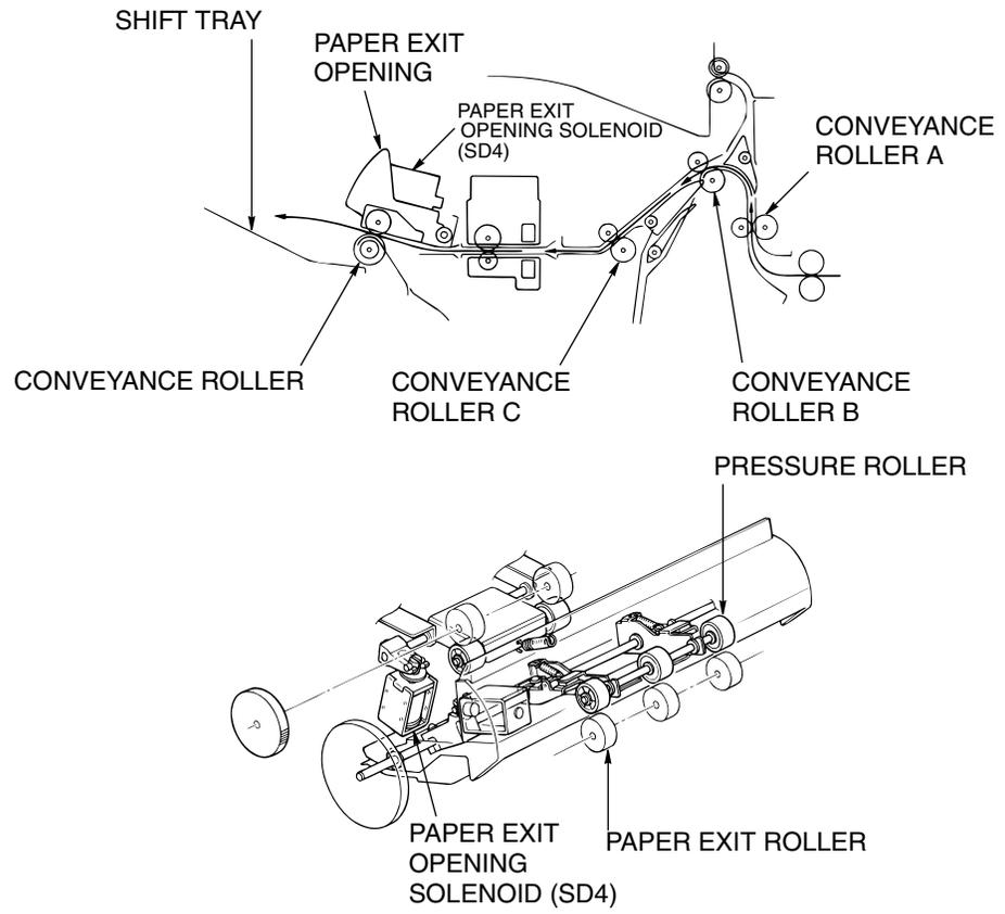
Figure 7-19. View of the Paper Exit Opening Unit
