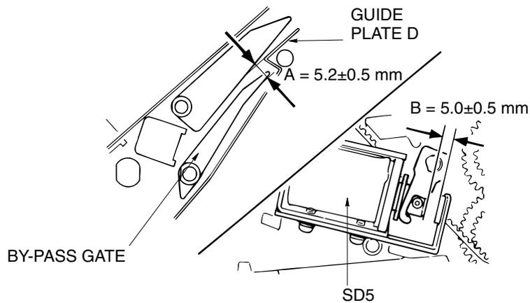
Figure 6-55. Adjustment of the By-Pass Gate
