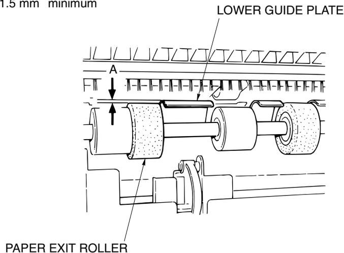
Figure 6-64. Adjustment of the Paper Exit Opening Lower Guide Plate
