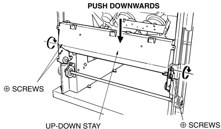
Figure 6-28. Removal of the Up-down Stay
