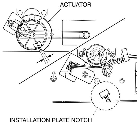
Figure 6-57. Adjustment of the Shift Position
