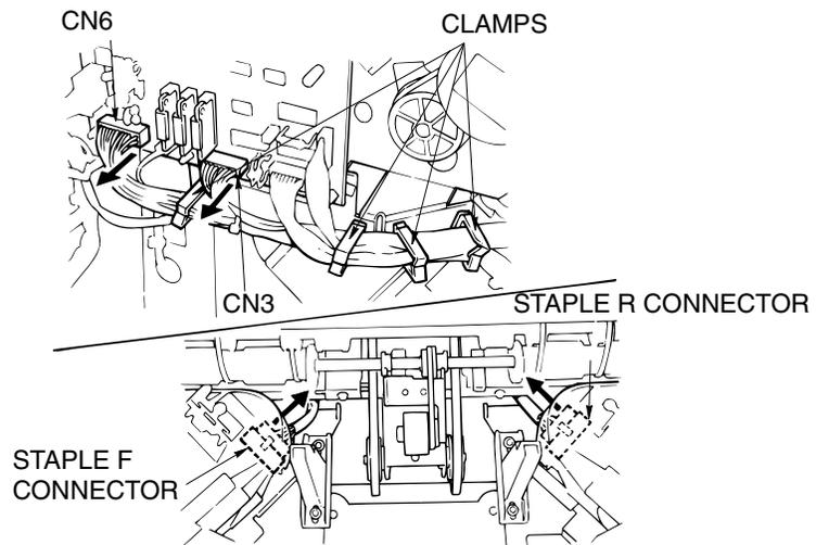
Figure 6-41. Removal of the Stacker Unit
