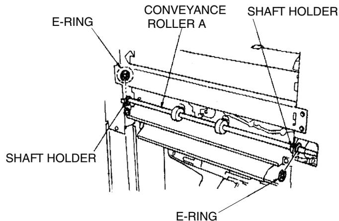
Figure 4-13. -2 Removal of the Conveyance Roller A and Pulley/F
