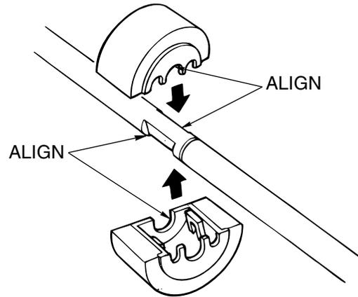
*Figure 4-7. Assembling of the Paper Exit Roller*
