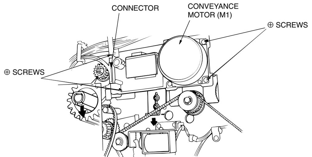
Figure 4-14. Removal of the Conveyance Motor (M1)
