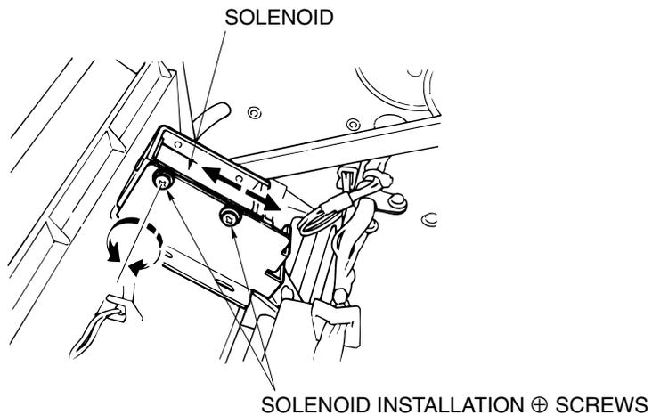
*Figure 6-63. Adjustment of the Paper Exit Opening Solenoid*
