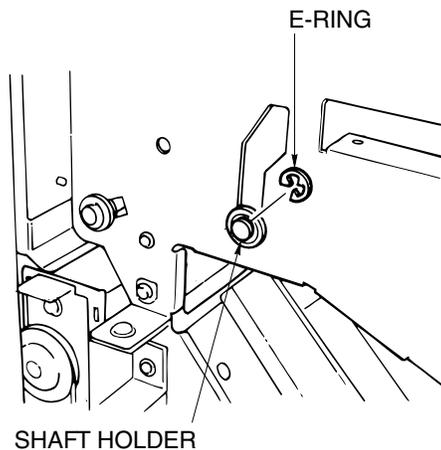
Figure 6-18. Removal of the Paper Exit Opening Unit
