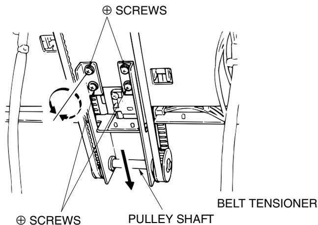
Figure 6-66. Adjustment of the Stacker paper Exit Belt Tension
