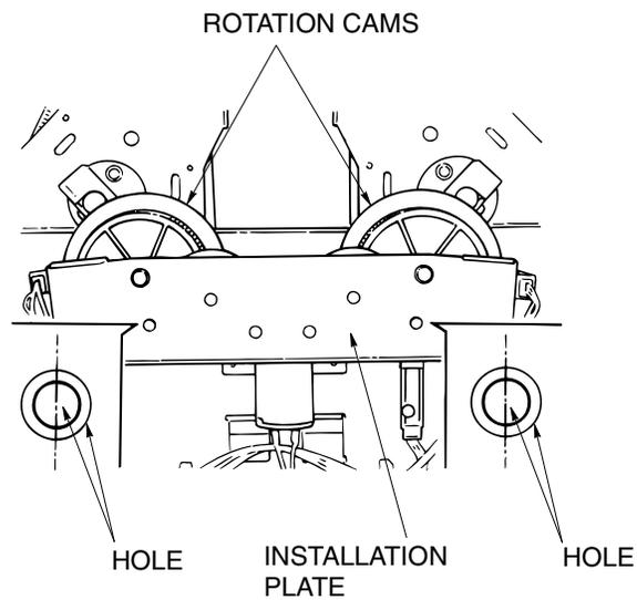
Figure 6-70. Adjustment of the Stapler Rotation Drive Section Installation
