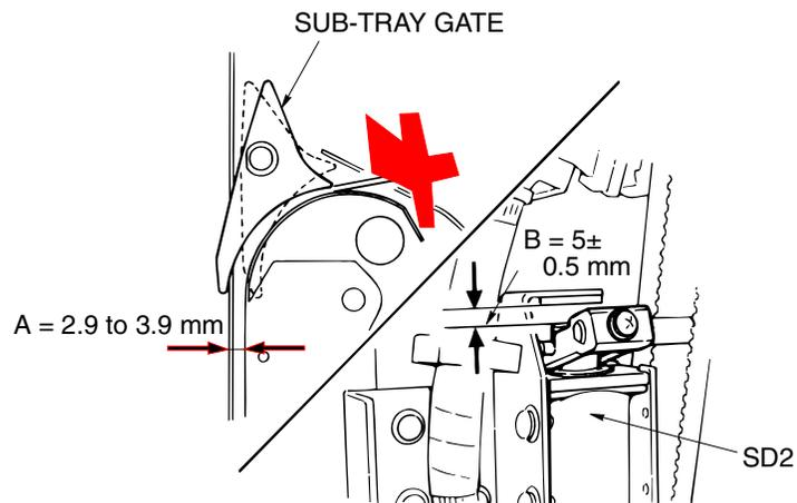
Figure 6-50. Adjustment of the Sub-tray Gate
