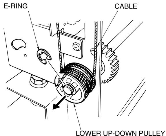
Figure 6-30. Removal of the Up-down Cable
