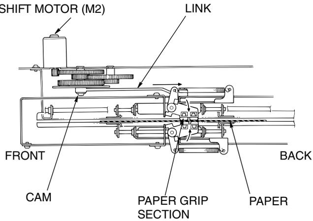
Figure 7-14. View of the Offset Operation
