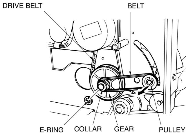
Figure 6-14. Removal of the Paper Exit Opening Unit
