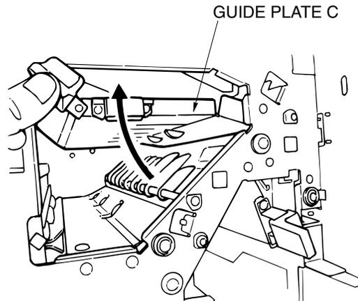
Figure 6-54. Adjustment of the By-Pass Gate
