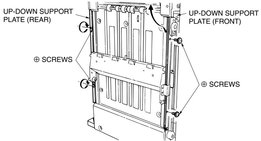
Figure 6-25. Removal of the Paper Exit Stopper Plate
