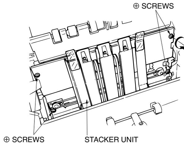
Figure 6-42. Removal of the Stacker Unit
