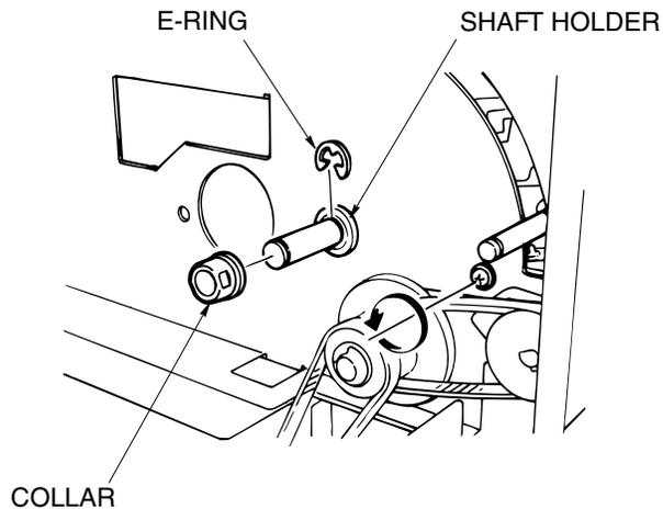
Figure 6-15. Removal of the Paper Exit Opening Unit
