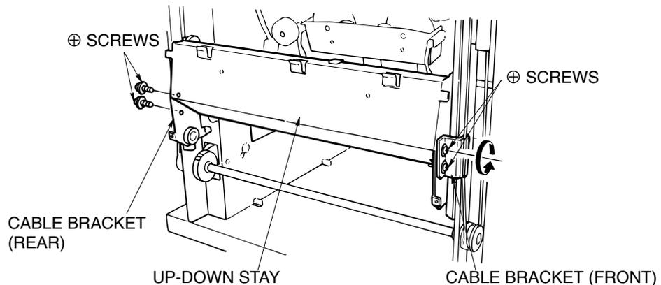
Figure 6-27. Removal of the Up-down Stay
