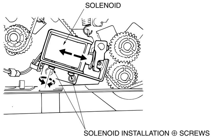
*Figure 6-56. Adjustment of the By-Pass Gate*
