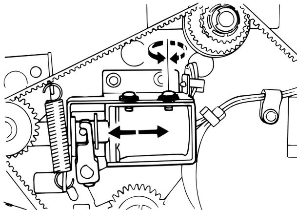
Figure 6-7. Removal of the Shift Unit
