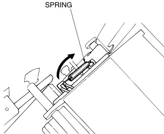
Figure 6-19. Removal of the Paper Exit Opening Unit
