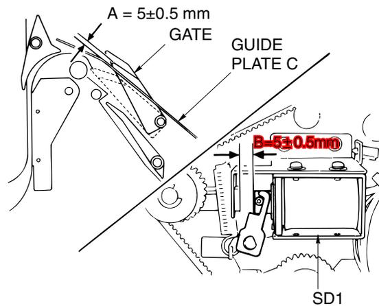
Figure 6-52. Adjustment of the Paper Route Switching Gate
