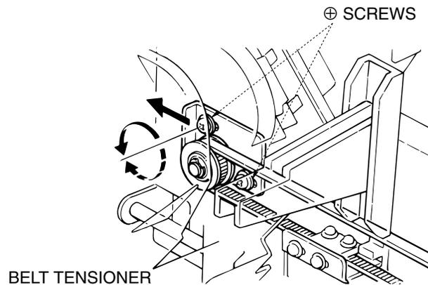
Figure 6-74. Adjustment of the Tension of the Stapler Move Timing Belt
