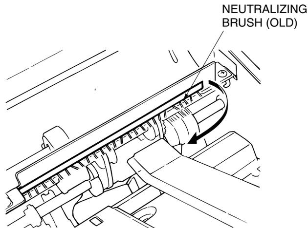
Figure 6-44. Removal of the Neutralizing Brush
