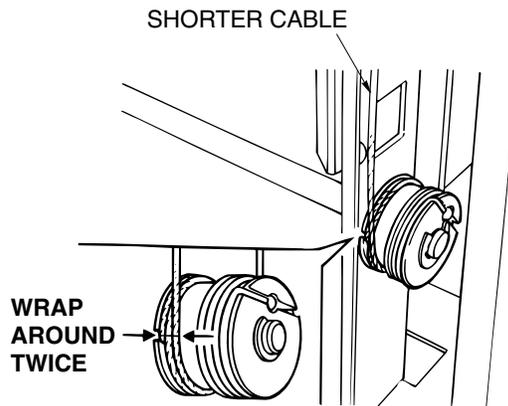
Figure 6-31. Removal of the Up-down Cable
