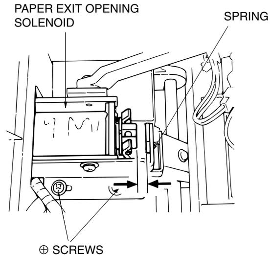
Figure 4-16. Removal of the Paper Exit Opening Solenoid
