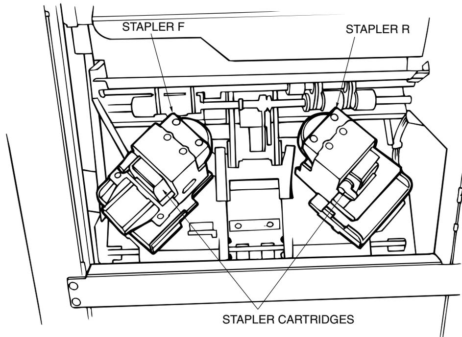
Figure 7-20. Construction of the Stapler Unit
