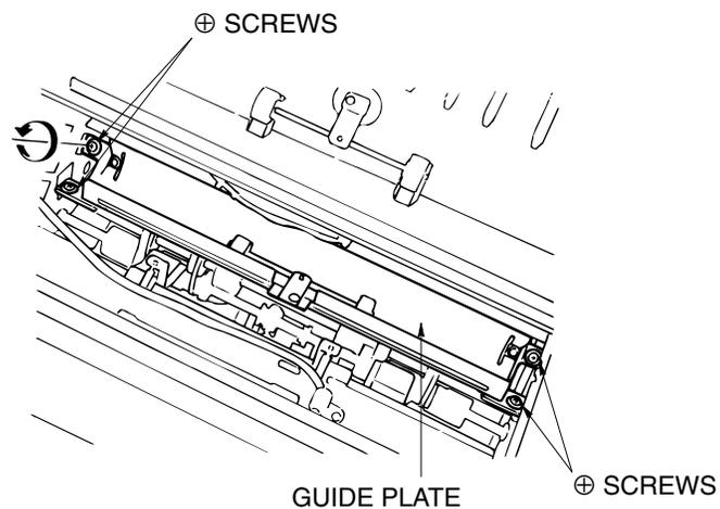
Figure 6-11. Removal of the Stacker Entrance Roller
