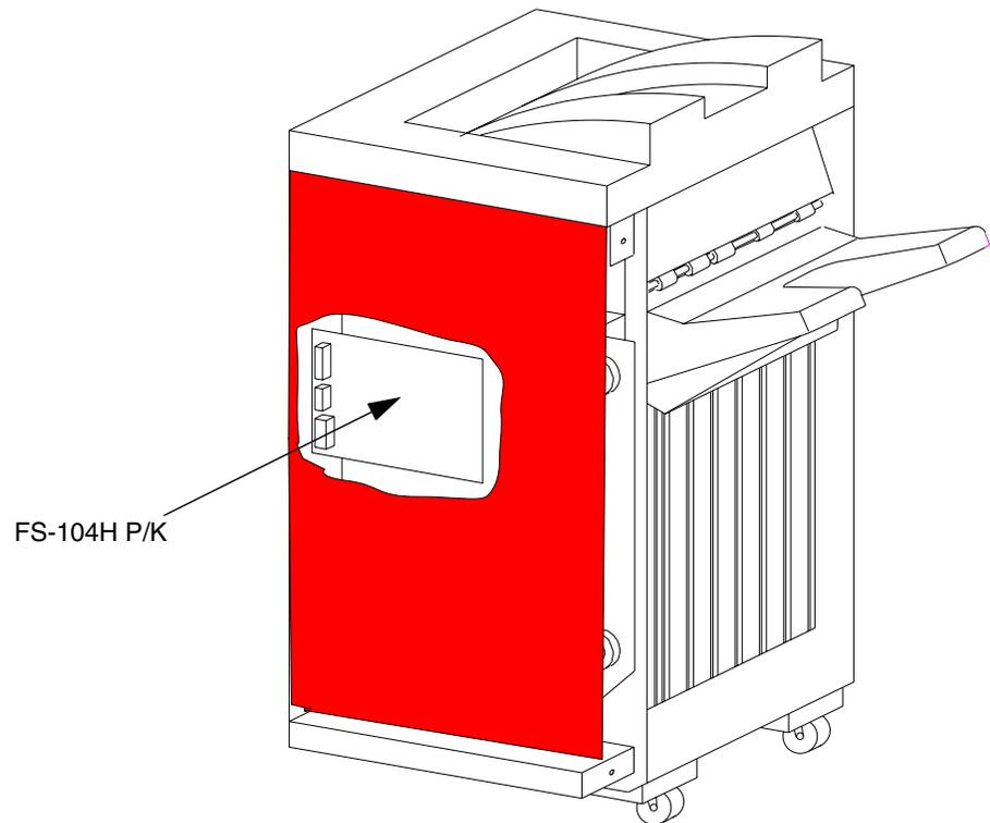
Figure 4-17. Removal of the FS-104H P/K
