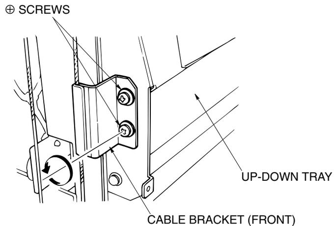
Figure 6-29. Removal of the Up-down Cable
