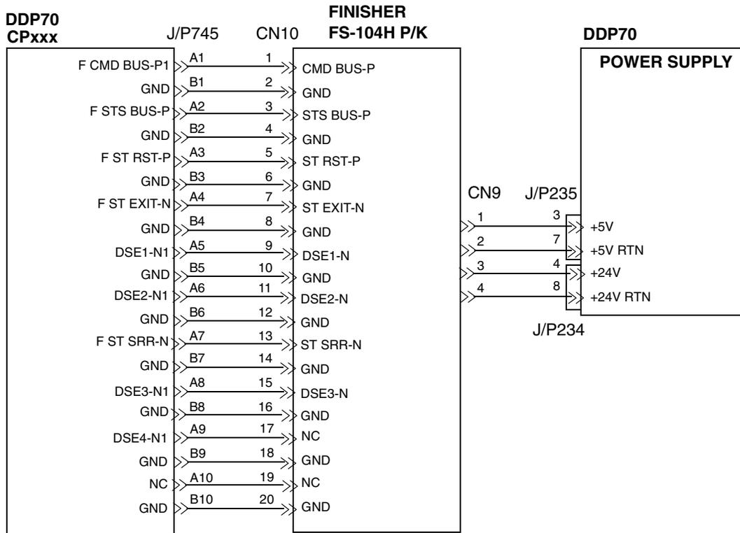
Figure 3-1. Finisher Circuit Diagram
