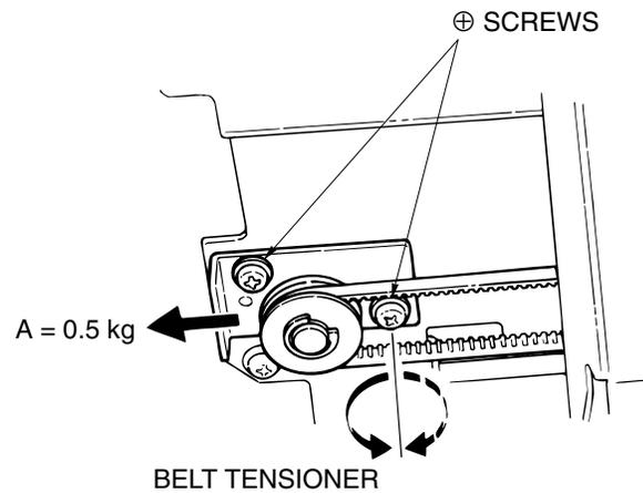
Figure 6-69. Adjustment of the Alignment Drive Timing Belt Tension
