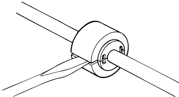
Figure 4-6. -2 Removal of the Paper Exit Roller
