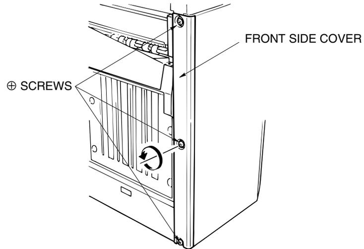
*Figure 6-4. Removal of the Front Side Cover*
