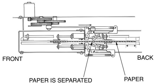
Figure 7-15. View of the Offset Operation
