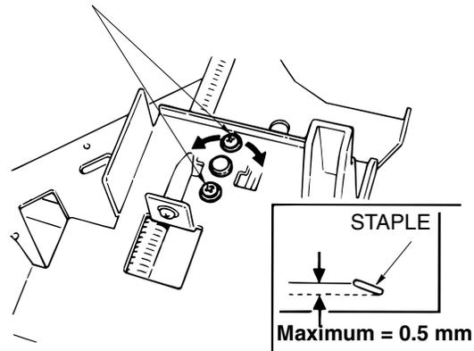
Figure 6-72. Adjustment of the Stapler 2 Position Mechanism
