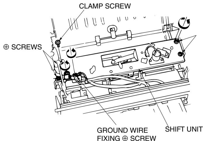
Figure 6-6. Removal of the Shift Unit
