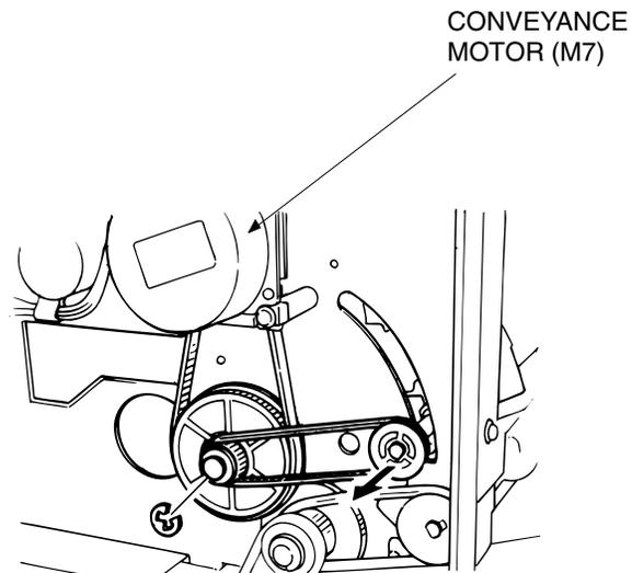
Figure 4-15. Removal of the Conveyance Motor (M7)
