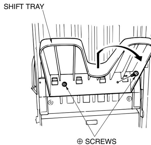
Figure 6-22. Removal of the Shift Tray
