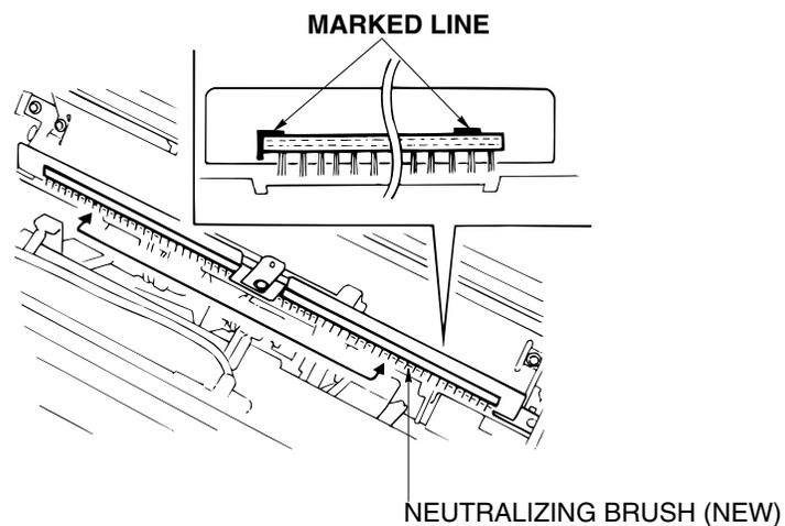
Figure 6-45. Removal of the Neutralizing Brush
