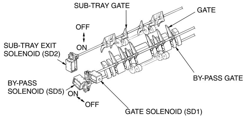
Figure 7-10. View of the Paper Path Switching
