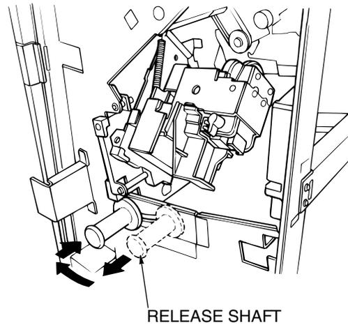
Figure 4-8. -1 Removal of the Stapler
