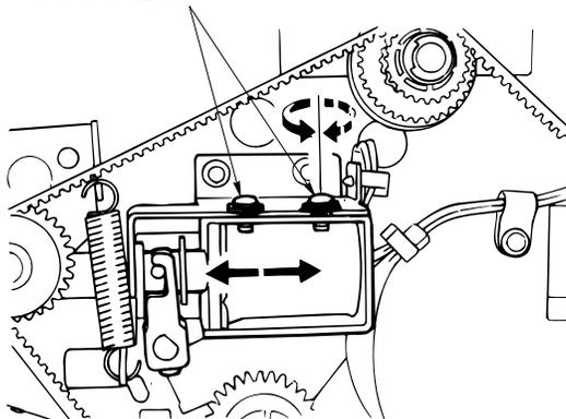
Figure 6-53. Adjustment of the Paper Route Switching Gate
