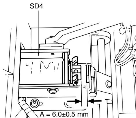
Figure 6-61. Adjustment of the Paper Exit Opening Solenoid
