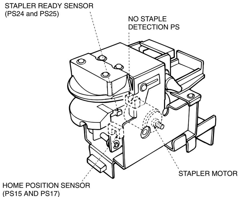
Figure 7-23. View of the mechanism for stapling in one place
