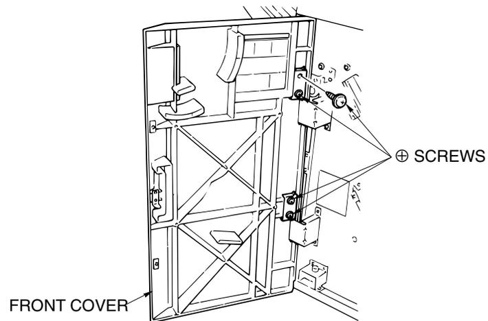
*Figure 6-3. Removal of the Front Cover*
