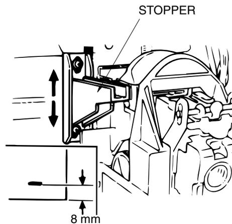
Figure 6-71. Adjustment of the Stapler 2 Position Staple Position
