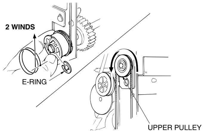
Figure 6-32. Removal of the Up-down Cable
