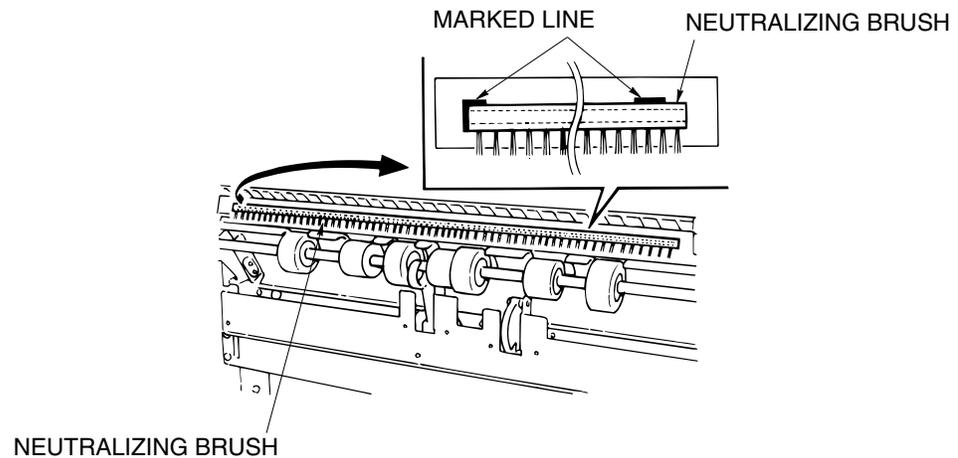
Figure 6-21. Removal of the Neutralizing Brush
