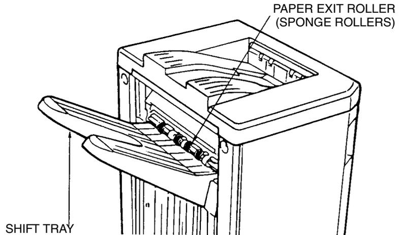
Figure 4-5. -1 Removal of the Paper Exit Roller
