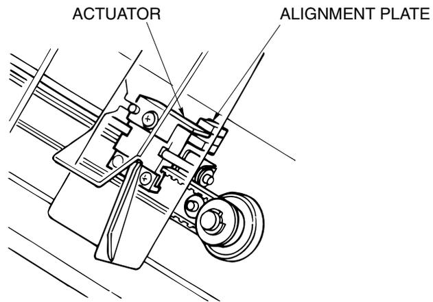
Figure 6-67. Adjustment of the Paper Exit Opening Lower Guide Plate
