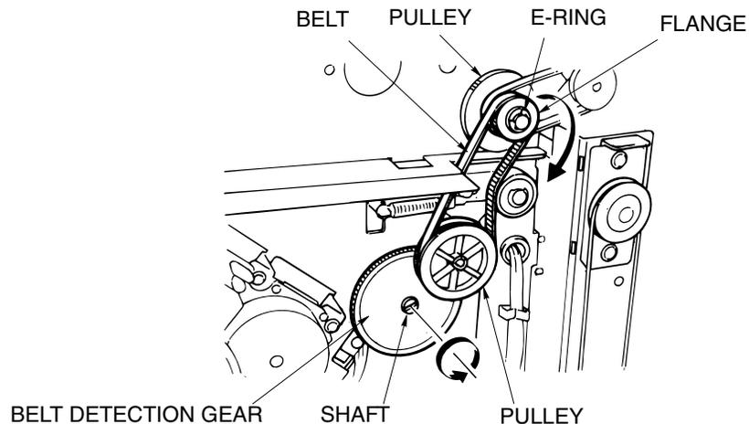
Figure 6-35. Removal of the Stacker Unit
