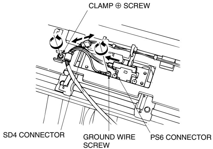
Figure 6-16. Removal of the Paper Exit Opening Unit
