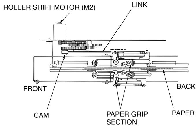
Figure 7-13. View of the Offset Operation
