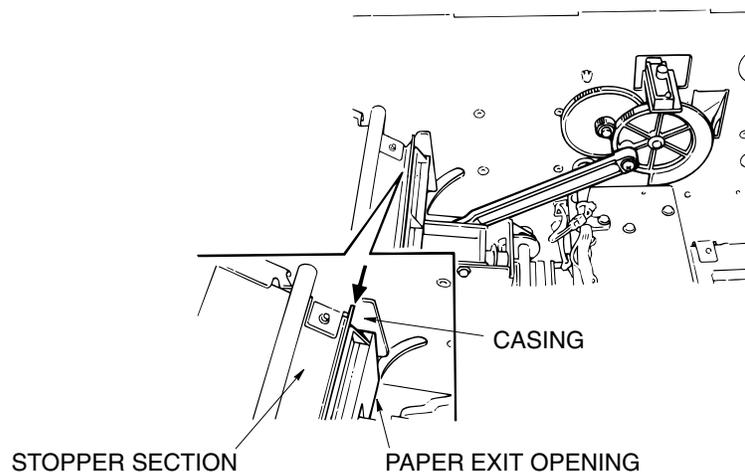
Figure 6-59. Adjustment of the Paper Exit Opening
