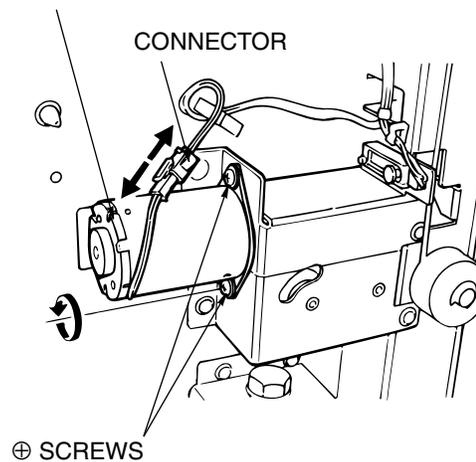
Figure 4-11. Removal of the Tray Up-down Motor
