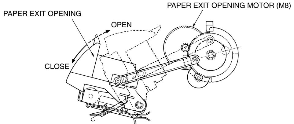
Figure 7-18. View of the Paper Exit Opening Unit
