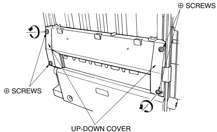
Figure 6-23. Removal of the Paper Exit Stopper Plate
