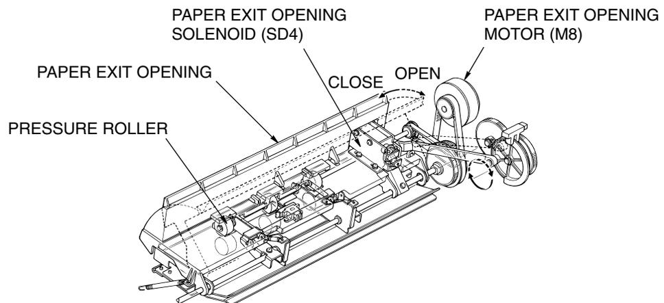
Figure 7-17. View of the Paper Exit Opening Unit
