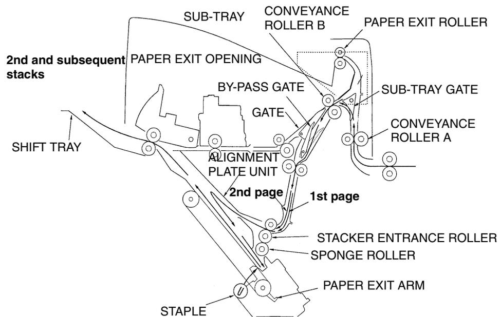
Figure 7-8. View of the second and subsequent stack
