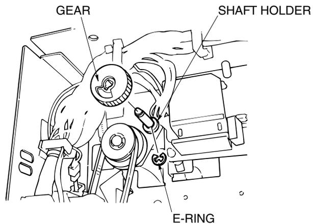
Figure 6-9. Removal of the Sub-tray Paper Exit Roller
