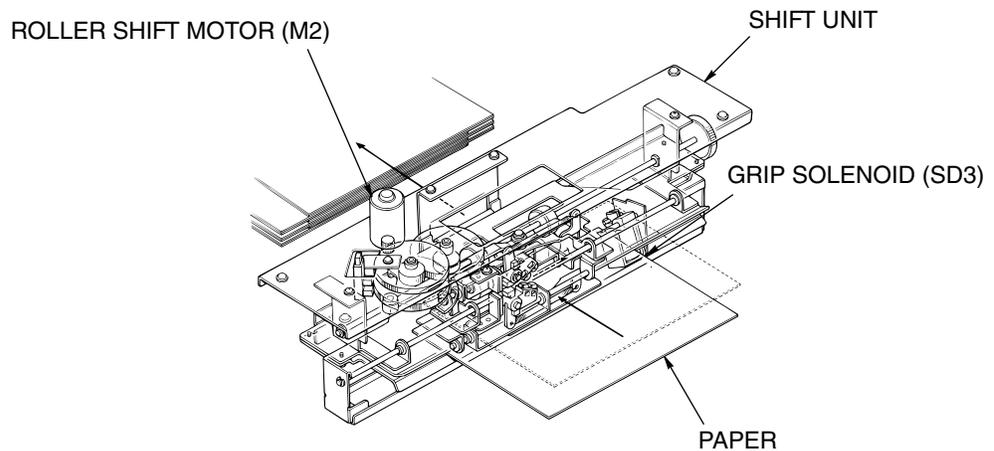
Figure 7-11. View of the Offset Operation
