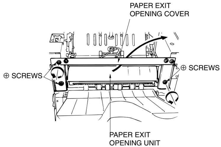
Figure 6-20. Removal of the Paper Exit Opening Unit
