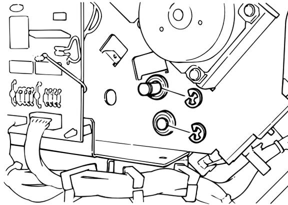
*Figure 6-13. Removal of the Stacker Entrance Roller*
