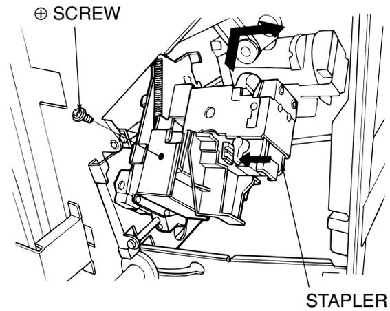
Figure 4-10. -3 Removal of the Stapler
