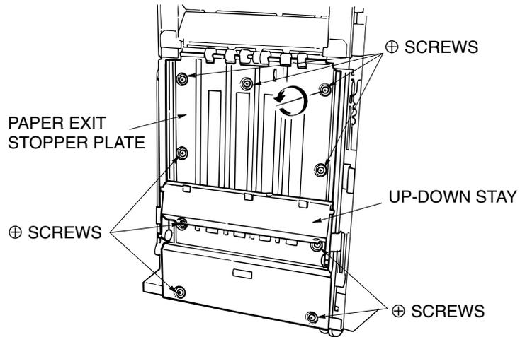
Figure 6-26. Removal of the Paper Exit Stopper Plate
