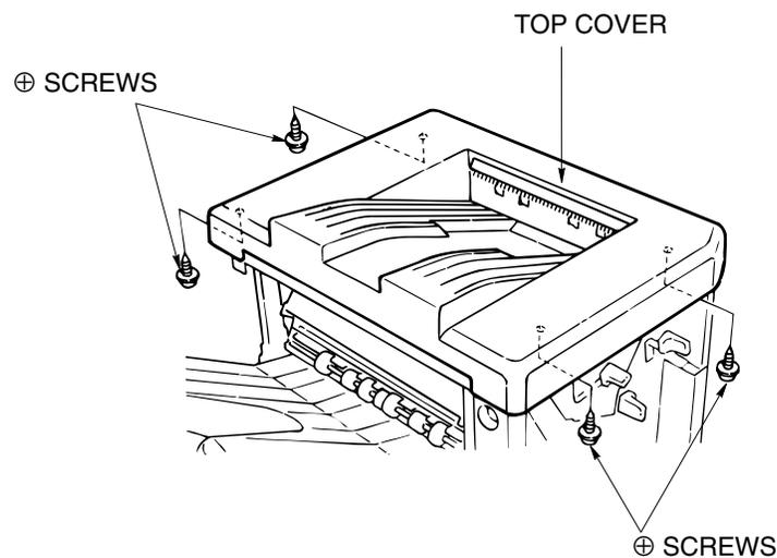
Figure 6-2. Removal of the Top Cover
