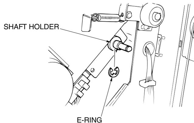
Figure 6-36. Removal of the Stacker Unit
