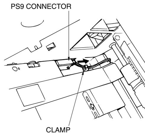
Figure 6-38. Removal of the Stacker Unit
