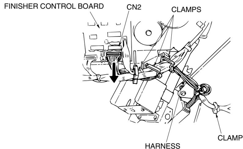
Figure 6-46. Removal of the Stapler Unit
