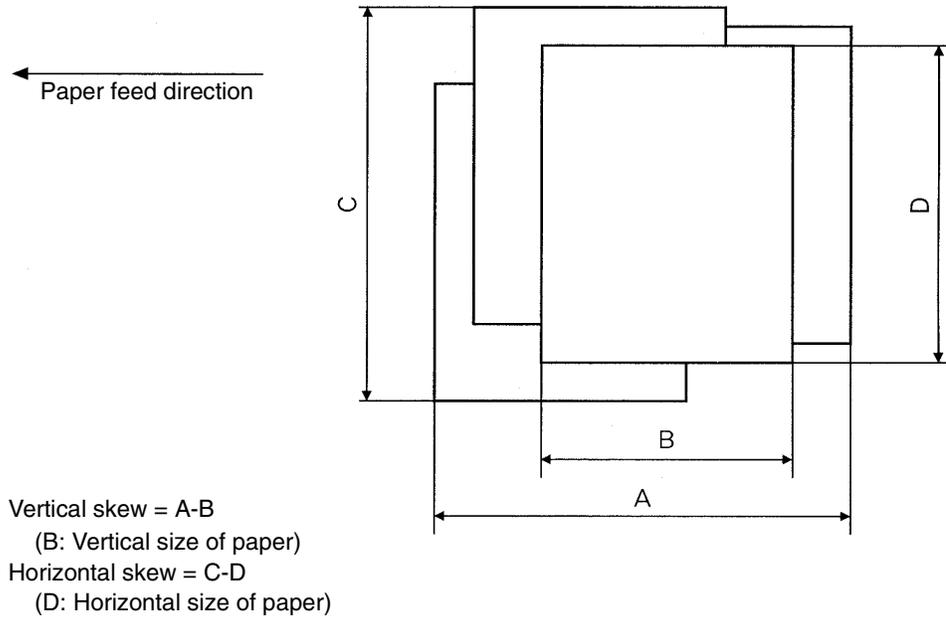
Figure 5-1. Vertical/Horizontal sizes of paper
