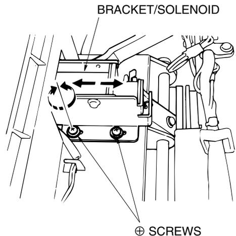
Figure 6-65. Adjustment of the Paper Exit Opening Lower Guide Plate
