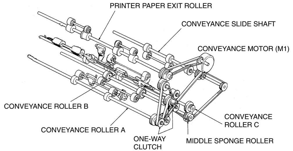
Figure 7-2. View of the Paper Conveyance Drive
