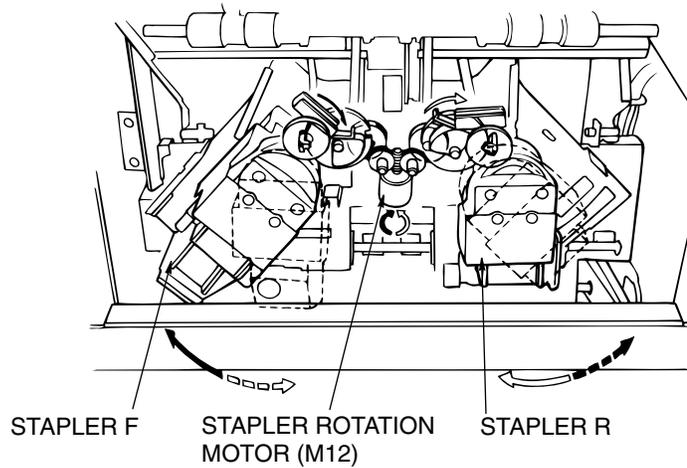
Figure 7-22. View of the mechanism for stapling in two places
