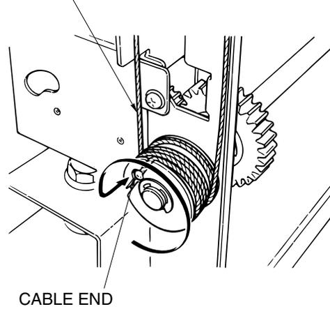
Figure 6-33. Removal of the Up-down Cable
