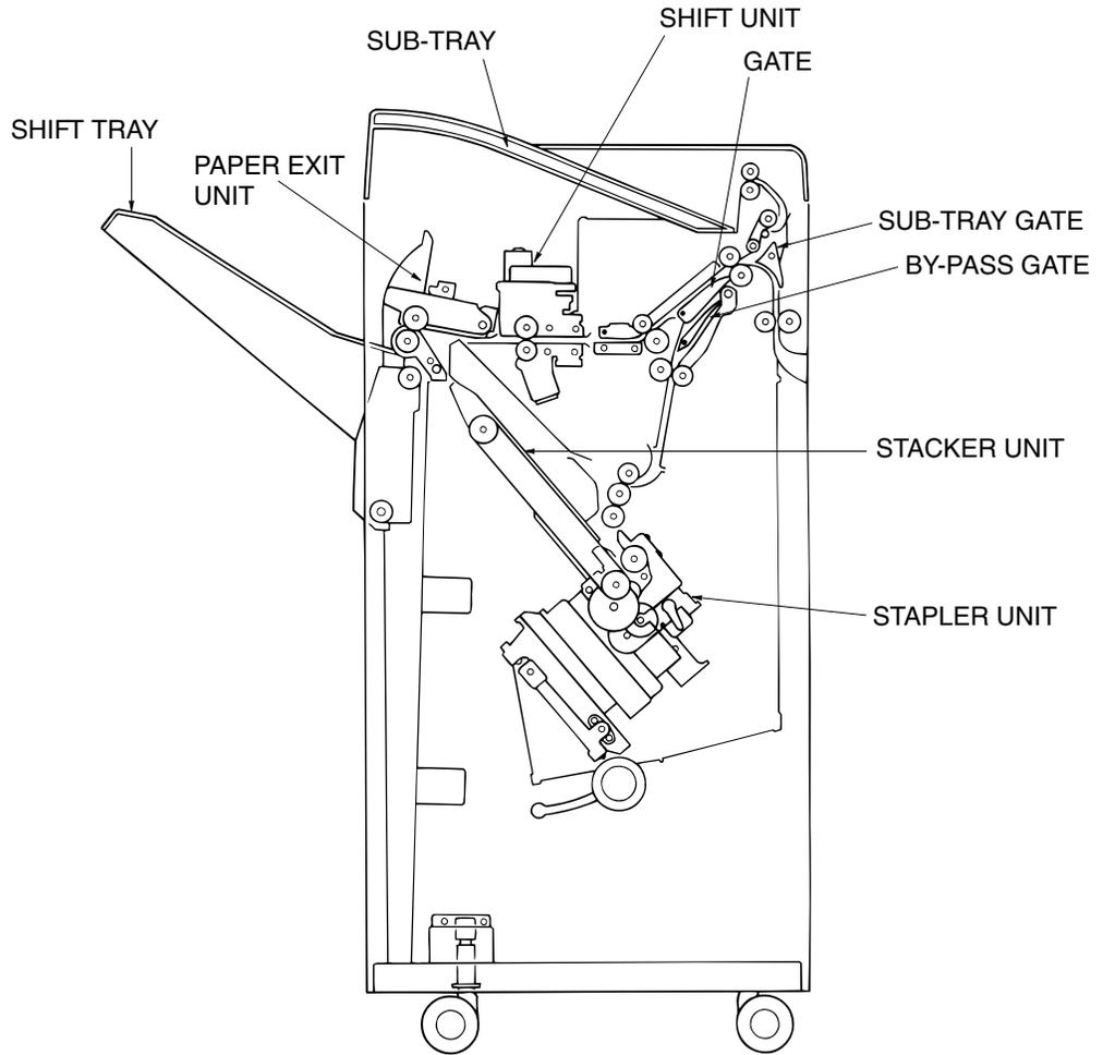
Figure 7-1. View of the Center Cross Section of the Finisher
