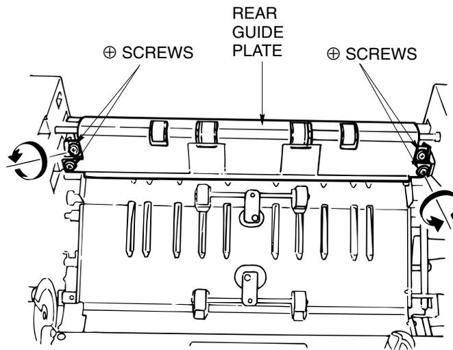
Figure 6-8. Removal of the Sub-tray Paper Exit Roller
