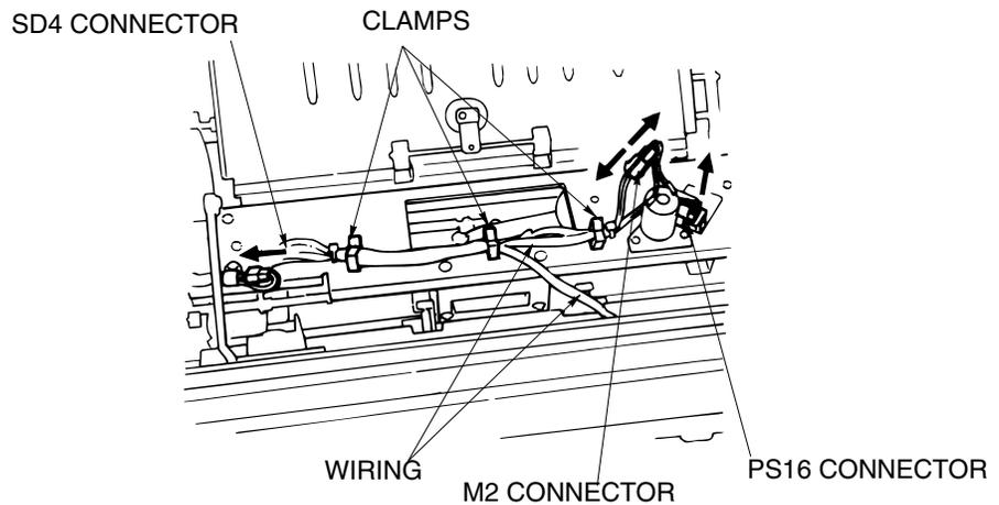
Figure 6-5. Removal of the Shift Unit
