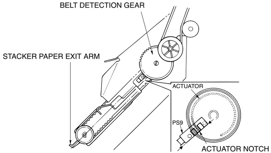
Figure 6-43. Removal of the Stacker Unit
