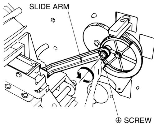
Figure 6-17. Removal of the Paper Exit Opening Unit
