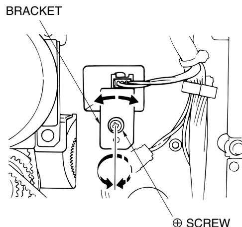
Figure 6-60. Adjustment of the Paper Exit Opening
