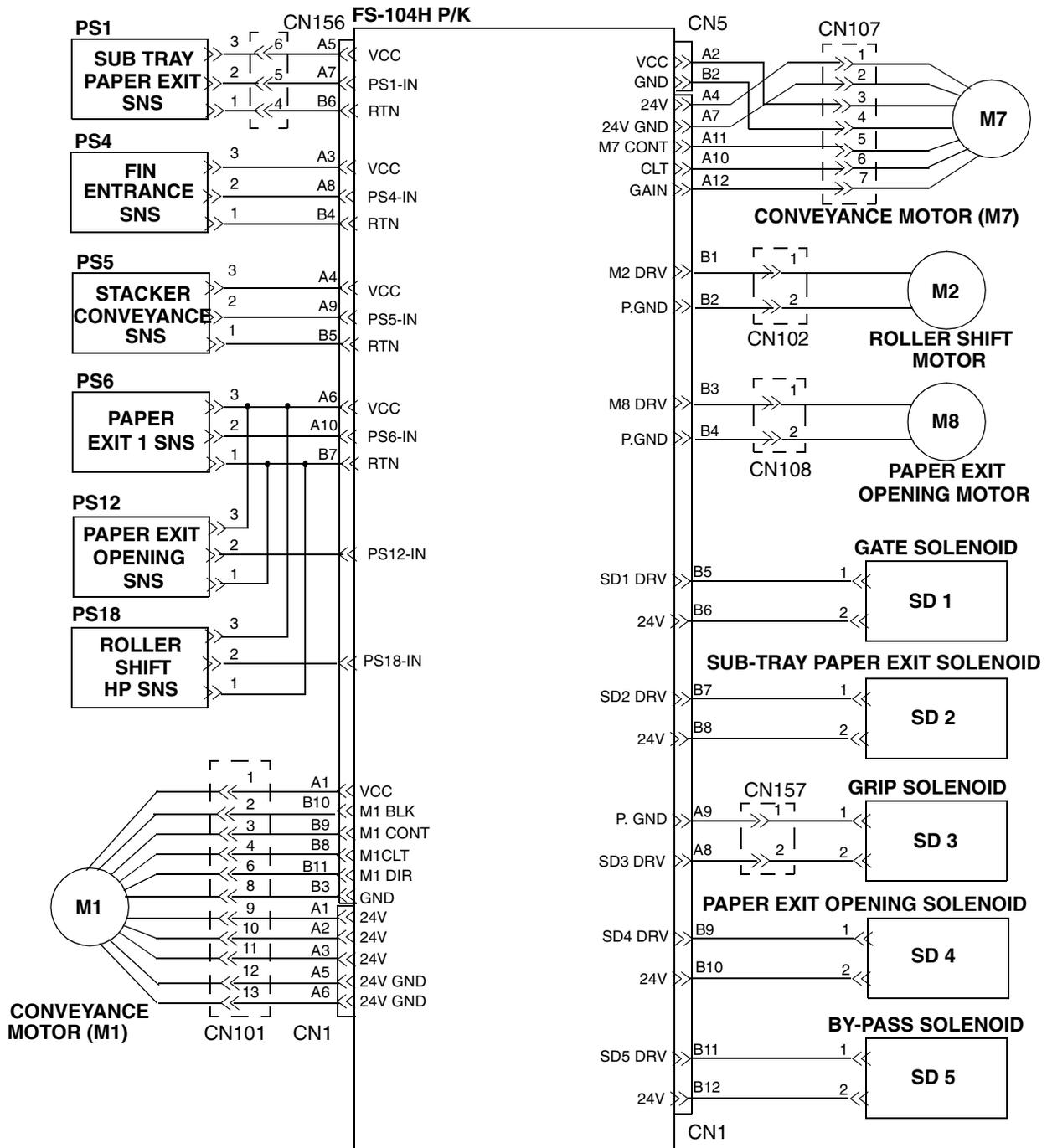
Figure 3-3. Finisher Circuit Diagram
