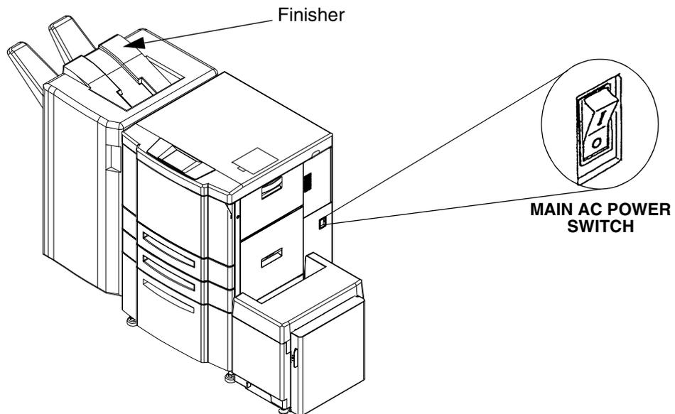
Figure 3-1. Location of the Main AC Power Switch
