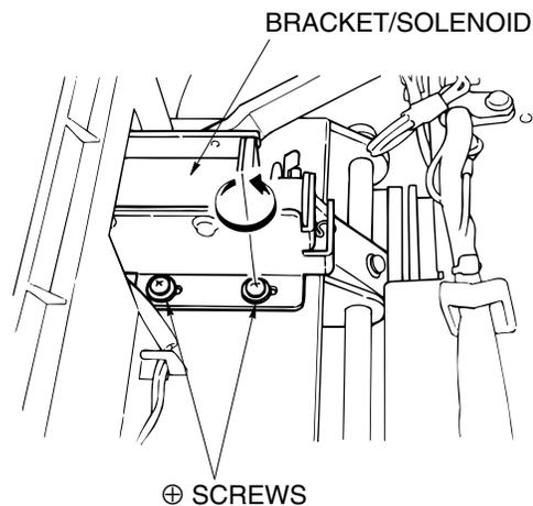
Figure 6-62. Adjustment of the Paper Exit Opening Solenoid
