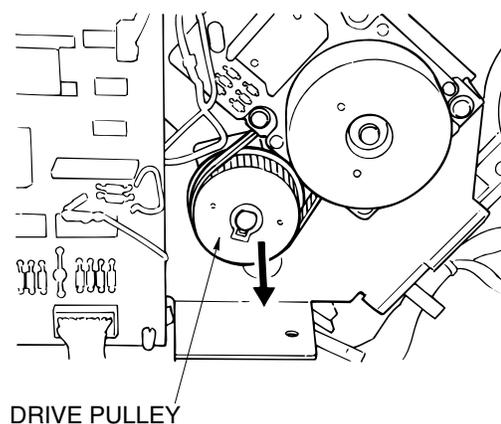
Figure 6-12. Removal of the Stacker Entrance Roller
