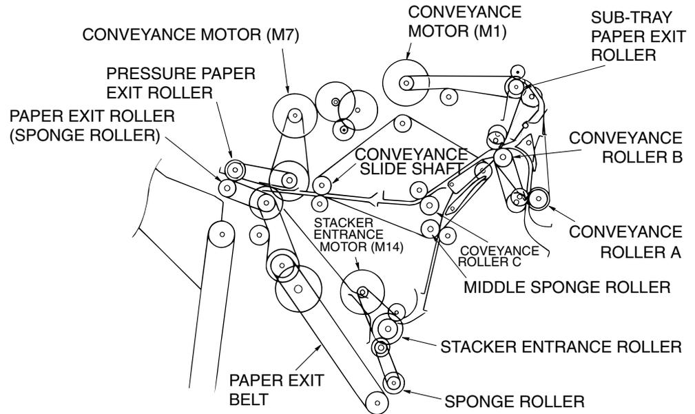
Figure 7-9. Construction of the Conveyance Section
