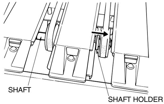
Figure 6-37. Removal of the Stacker Unit
