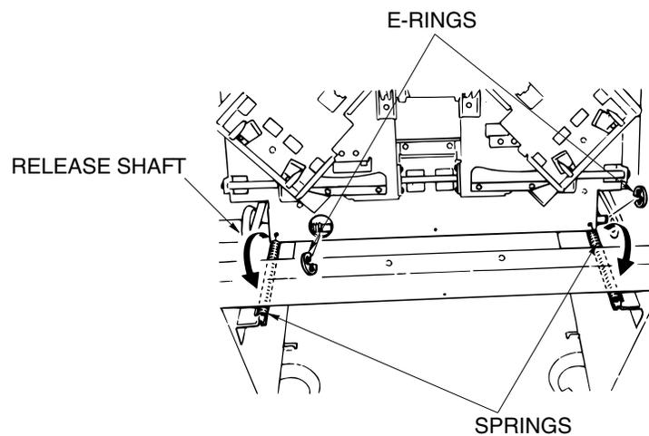
Figure 6-47. Removal of the Stapler Unit
