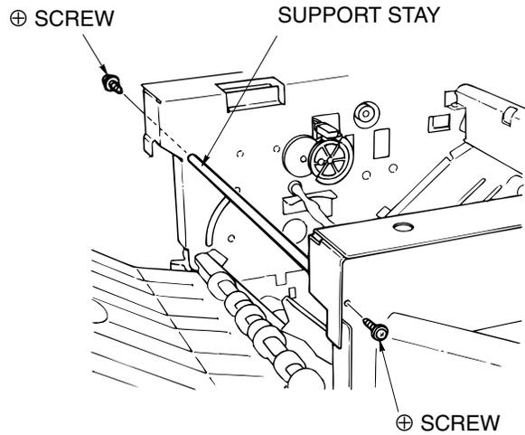
Figure 6-40. Removal of the Stacker Unit
