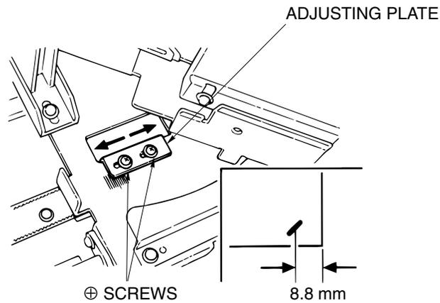
Figure 6-73. Adjustment of the Stapling Position for 1 Position Stapling
