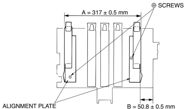
Figure 6-68. Adjustment of the Alignment Plate Installation Position
