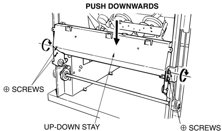
Figure 6-34. Removal of the Up-down Cable
