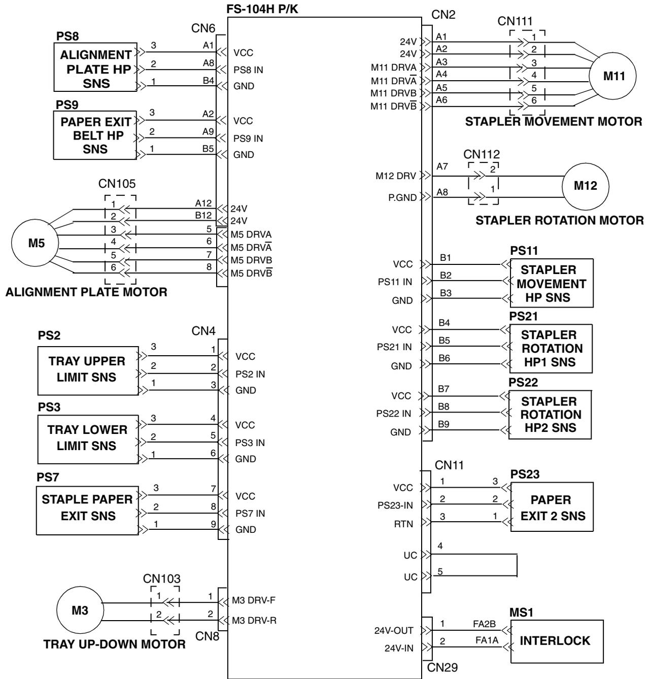
Figure 3-4. Finisher Circuit Diagram
