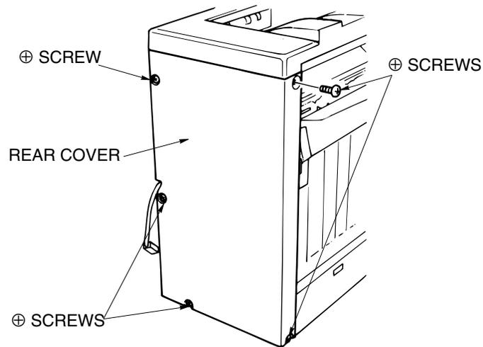
Figure 6-1. Removal of the Rear Cover
