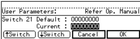
Each digit in the display is referred to in the Operator's Manual by a number from 0 to 7, starting from the *right*.
