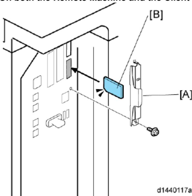
1. Remove the SD-card slot cover [A] from the SD card slots (x 1)
