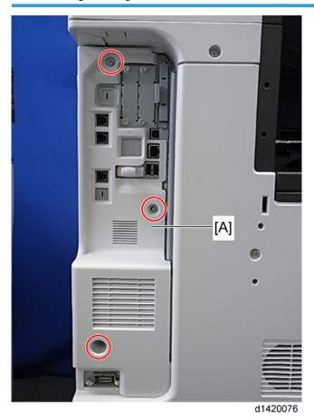
1. Remove the controller box cover [A] (  $\mathscr{F}$  x 3).
