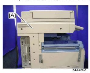
1. Remove the scanner left cover [A] (  $\widehat{\!\!\textit{F}}\!\!\!/ \times 2$  ).
