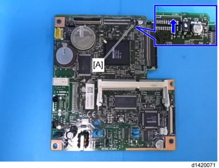
12. Move the Dip Switch [A] of the old FCU board from "OFF" to "ON".
