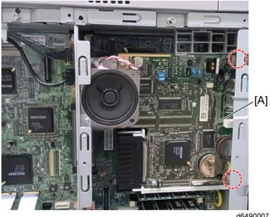
8. Secure the FCU [A] with two screws included in the kit (M3x6:  $\mathcal{F}$  x 2).
