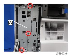
8. Remove the cover (LINE 2) [B] and cover (LINE3) on the controller cover [A].
