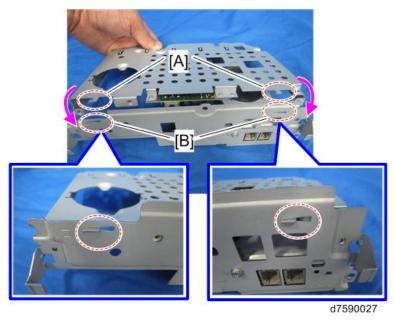
5. Fasten the SG3 interface unit [A] and the fax unit. [B] ( $\mathcal{F}$ x2).
