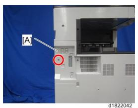
2. With its label turned away toward the front of the machine, insert **Fax Connection Unit** into SD card slot 2 (lower slot) [A]. Push it in until you hear it click and lock in place.
