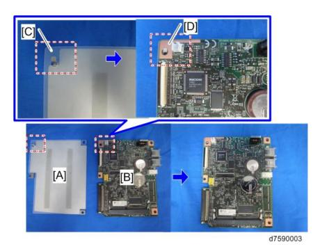
8. Attach the FCU panel [A] to the new FCU [B] (Left:  $\Re x2$  (M3x4), Right:  $\Re x1$  (3x6)).
