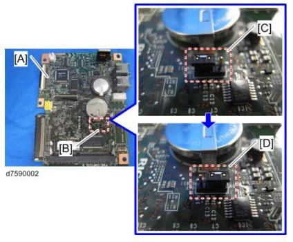
$5. \ \, \text{Attach the shield plate [A] to the FCU [B]. (Fit the hook [C] into the hole [D] in the FCU.)}$
