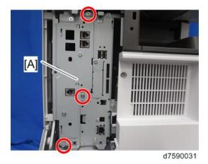
11. Remove the cover (LINE 2) [B] on the controller cover [A].
