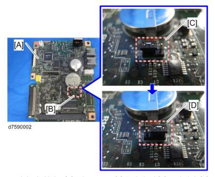
7. Attach the shield plate [A] to the new FCU [B]. (Fit the hook [C] into the hole [D] in the FCU.)
