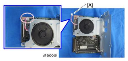
8. Put the FCU [B] in the groove [A] and insert it.
