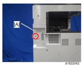
2. Remove the fixing screws of the scanner front cover [A] (Px2).
