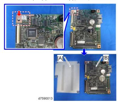
6. Switch the battery jumper switch [A] to the "ON" position on the new FCU.
