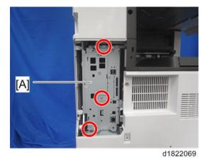
3. Remove the SG3 board [A] (Fx6).
