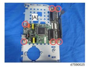
6. Connect the flat cable [B] to the fax unit [A].
