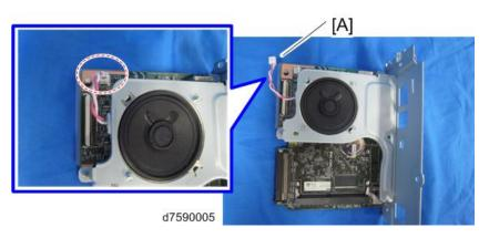
10. Connect the flat flexible cable [A] to the new FCU [B]. This flexible cable is shipped with the new FCU.
