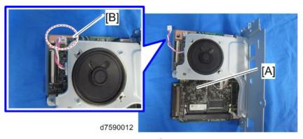
4. Remove the FCU [A] with the shield plate (Fx3).
