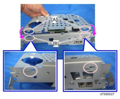
8. Fasten the SG3 interface unit [A] and the fax unit. [B] (  $\not\!\!\!P x2$  ).
