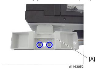
12. Make two loops with the telephone cord, and then attach the ferrite core [A] to the cable.
