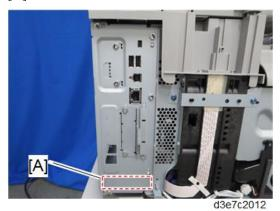
**13.** Open the line and telephone connector covers [A] with a flat-head screw driver.
