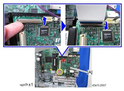
**<u>9.</u>** Attach the battery jumper switch [A] on the removed FCU board to switch to the Restore mode. This jumper switch is provided with the new FCU board.
