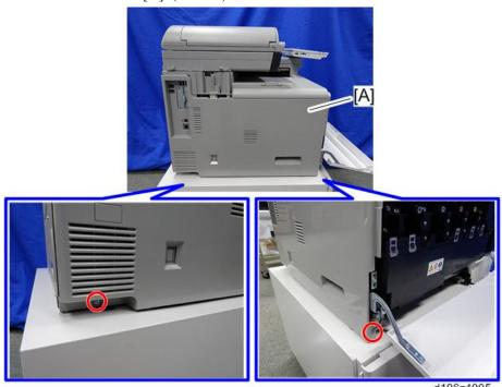
5. Remove the controller cover [A] with the HDD [B].
