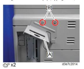
5. Attach the cradle [A] to the bracket. (flat head screw)
