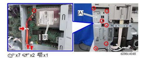
**<u>6.</u>** Attach the speaker bracket [B] while sliding the tabs into the cutouts [A] in the controller box. (hook x 2)
