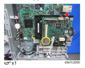
**<u>6.</u>** Switch the battery jumper switch [A] of the new FCU to the "ON" position before installing.
