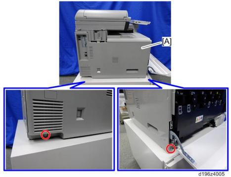
**<u>4.</u>** Remove the controller cover [A] with the HDD [B].
