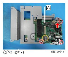
**9.** Switch the battery jumper switch [A] of the FCU board to the "ON" position before installing the fax unit on the controller board.
