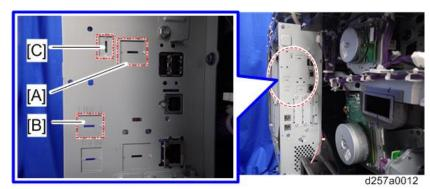
**<u>8.</u>** Install the G3 interface unit [A] on the controller board.
