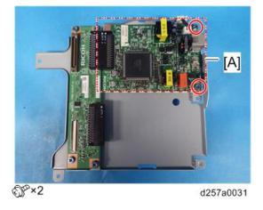
3. Install the G3 board [A] removed from the second G3 interface unit on the first G3 interface unit.
