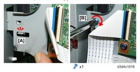
13. Make sure that the connectors fit correctly into the holes on the controller box faceplate.
