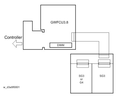
The FCU, which is composed of one PCB, controls all the fax communications and fax features, in cooperation with the controller board.
