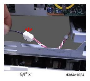
7. Remove fax unit bracket [A] with FCU attached.
