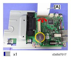
11. Move the jumper on the new FCU from the OFF [A] to ON [B] to switch the onboard battery on.
