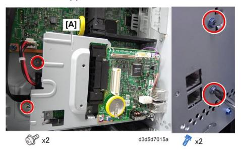
8. Remove the old FCU from the bracket, and then mount the new one on the bracket.
