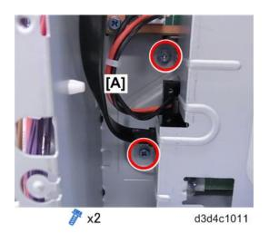
15. Fasten the small bracket [A] (provided accessory) to the center stay of the controller box.
