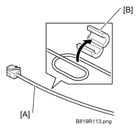
1. Loop one end of the telephone cable [A] once, then clamp it with the ferrite core (K3 NF-75(N)BK0) [B] as shown.
