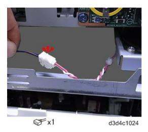
10. Below the FCU, set the clamps [A], and then fasten the clamps on the harness [B].
