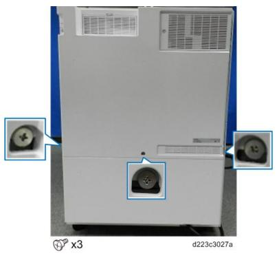
$2. \ \ \text{Remove the upper screws of the rear upper cover}.$
