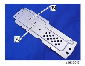
4. Switch the battery jumper switch [A] to the "ON" position.
