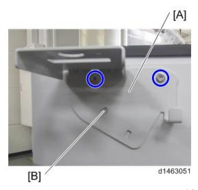
7. Attach the cradle [A] to the handset bracket ( x 2).
