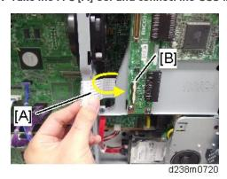
8. Secure the FFC [B] with the supplied clamp [A].
