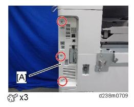
2. Remove the interface slot cover [A] ( x 2).
