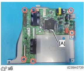
6. Remove the SG3 board [A] from one of the CCU I/F and SG3 board assemblies removed in step 5.
