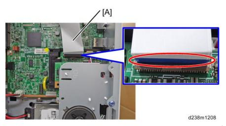
11. Attach the removed FCU board [A] to the center frame of the controller box ( x 1). Then attach the flat cable to CN603 of the removed FCU board.
