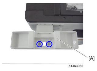
8. Make two loops with the telephone cord, and then attach the ferrite core [A] to the cable.
