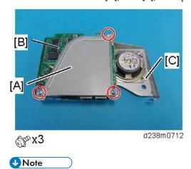
• Make sure that the clamp [B] is pressing the memory unit [A] and holding it in place.
