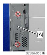
3. Pull out the FCU [A] from the interface slot.
