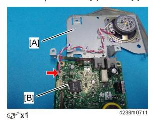
6. Attach the shield [A] to the FCU [B] and speaker bracket [C].
