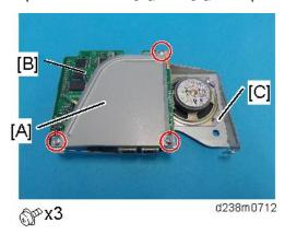
3. Attach the supplied clamp [B] to the speaker bracket [A].
