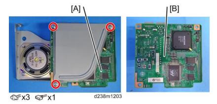
6. Change the orientation of the battery jumper switch [A] on the removed FCU board, and then attach the battery jumper switch [B] on the FCU board to switch to the Restore mode.
