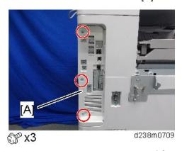
2. Remove the interface slot cover [A] ( $\Im x$  2).
