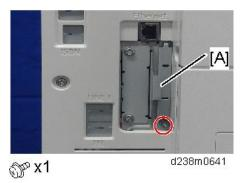
2. Insert the Fax Connection Unit SD card into SD card slot 1 [A: Upper Slot].
