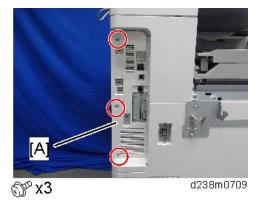
2. Remove the interface slot cover [A] ( $\Im^{*}x$  2).
