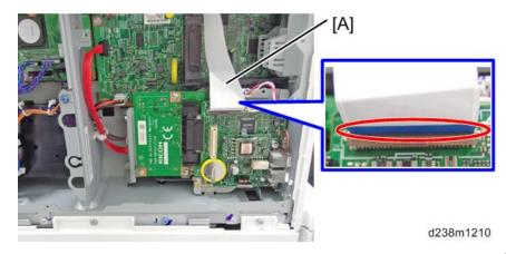
10. Attach the removed FCU board [A] to the center frame of the controller box (<sup>(3)</sup> x 1). Then attach the flat cable to CN603 of the removed FCU board.
