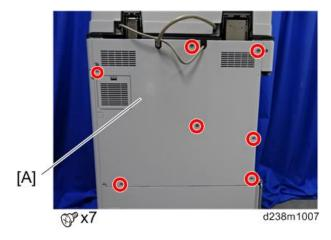
3. Remove the controller box cover [A].
