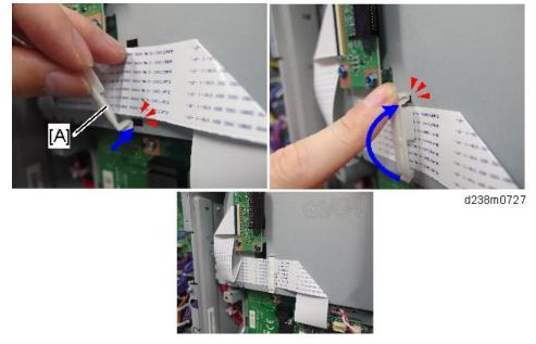
8. Attach the FFC Holder [A] to secure the FFC.
