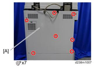
3. Remove the controller box cover [A].
