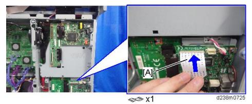
• Release the connector lock [B] and connect the FFC, and then lock the FFC.
