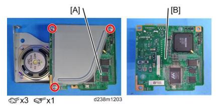
6. Change the orientation of the battery jumper switch [A] on the removed FCU board, and then attach the battery jumper switch [B] on the FCU board to switch to the Restore mode. The battery jumper switch [B] is supplied with the new FCU board.
