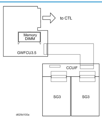
Together with the controller board, the FCU controls all the fax communications and fax features. The FCU also contains the ROM, SRAM and NCU circuits.
