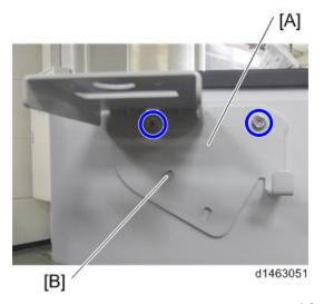
11. Attach the cradle [A] to the handset bracket ( $\Im$  x 2).
