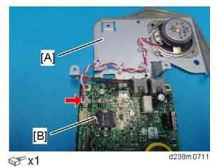
6. Attach the shield [A], FCU [B], and speaker bracket [C] together.
