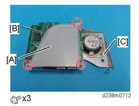
7. Insert the FCU [A] completely into the interface slot.
