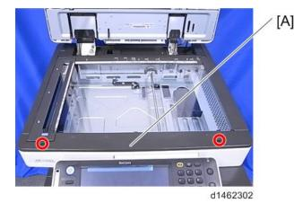
6. Remove the scanner left cover [A] ( x 3).
