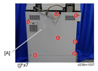
4. Remove the controller box cover [A].
