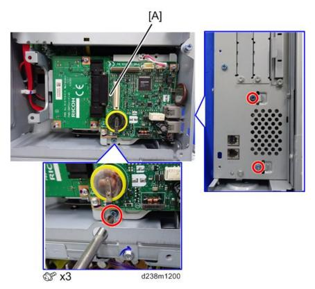
6. Change the orientation of the battery jumper switch [A] on the removed FCU board, and then attach the battery jumper switch [B] on the FCU board to switch to the Restore mode.
