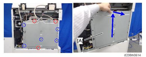
4. Remove the "LINE2" [A] cover using a screwdriver.
