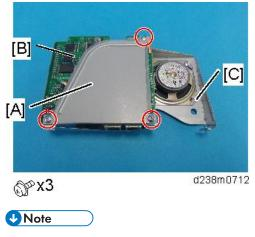
• Make sure that the clamp [B] is pressing the memory unit [A] and holding it in place.
