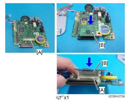
4. Attach the memory unit [B] to the FCU connector [A]
