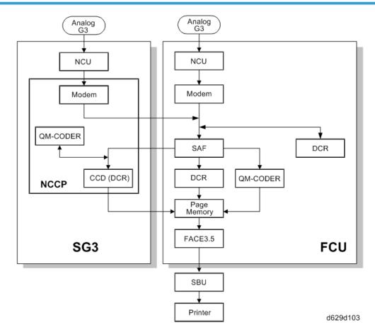
First, the FCU stores the incoming data from either an analog line to the SAF memory. (The data goes to the FACE3 at the same time, and is checked for error lines/frames.)
