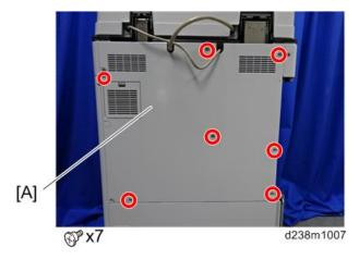
3. Remove the controller box cover [A].
