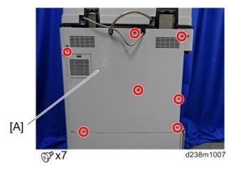
3. Remove the controller box cover [A].
