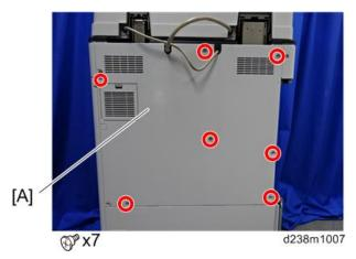
3. Remove the controller box cover [A].
