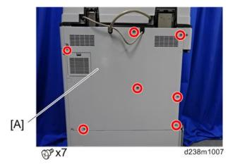
9. Remove the controller box cover [A]. Red circle: remove Blue circle: loosen
