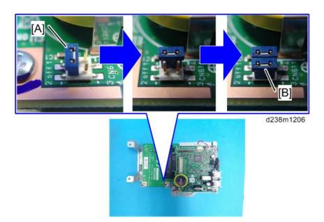
7. Switch the battery jumper switch [A] of the new fax unit to the "ON" position before installing.
