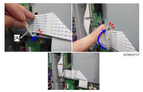
12. Attach the FFC Holder [A] to secure the FFC.
