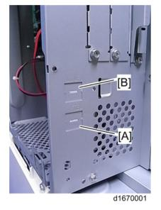
5. Switch the battery jumper switch [A] to the "ON" position.
