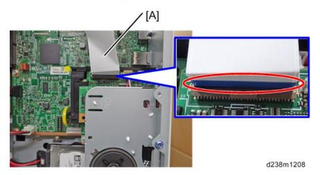
11. Attach the removed FCU board [A] to the center frame of the controller box (<sup>(W)</sup>x 1). Then attach the flat cable to CN603 of the removed FCU board.
