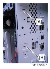
5. Remove the CCU I/F board and SG3 board [A] from the SG3 interface unit. Repeat the same procedure for the second SG3 interface unit.
