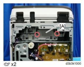
6. Attach the bracket [A] to the Fax Unit.
