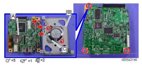
7. Connect the flat flexible cable (a service part) to the old FCU board.
