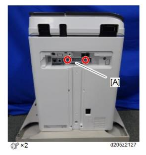
Insert the SD card (Fax Connection Unit Type M15) in SD slot 1 [A] if SD slot 1 is vacant. If slot 1 is not vacant, follow "Moving a Fax Communication application into an SD card in SD slot 1" shown below.
