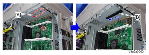
7. Slide the FCU [B] into the slot along the guide rails [A].
