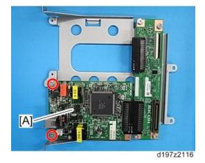
6. Attach the SG3 board [A] removed in step 5 to the CCU I/F of the other SG3 interface unit [B] (@ x 2).
