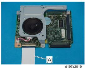
5. Switch the battery jumper switch [A] to the "ON" position.
