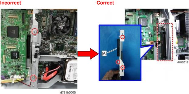
10. Fasten the relay board [A] (Px2). 3
