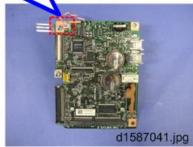
5. Grounding plate (2-tip) [A] on the back of the FCU (  $\ensuremath{\widehat{\mathcal{F}}}$  x 1).
