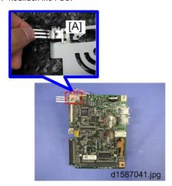
5. Attach the grounding plate (2-tip) [A] on the back of the FCU ( $\mathscr{F}$  x1).
