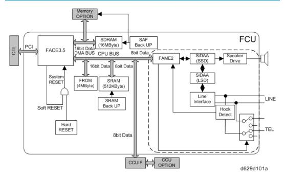
The FCU (Facsimile Control Unit) controls fax communications, the video interface to the base copier's engine, and all the fax options.
