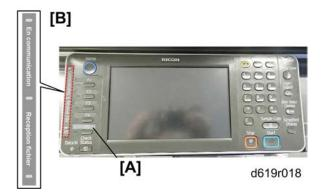
1. Attach the fax function decal [A] to F5.
