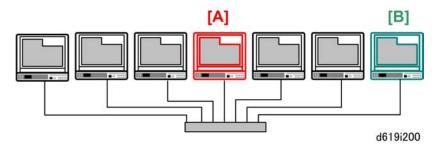
The machines must be on the same network. In the drawing above, [A] has the FCU (Fax Option Type 9002 (D619)) and at least one G3 interface board installed (G3 Interface Unit Type 9002 (D619)). Another machine [B] without the fax hardware (in the same network) can be connected to the master machine to make it capable of functioning as a fax.
