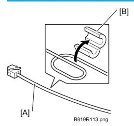
1. Loop one end of the telephone cable [A] once, then enclose it with the ferrite core (K3 NF-75(N)BK0) [B] as shown.
