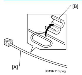
1. Loop one end of the telephone cable [A] once, then clamp it with the ferrite core (K3 NF-75(N)BK0) [B] as shown.
