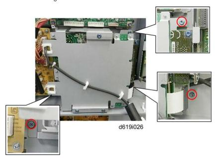
21. Fasten the FCU to the back of the machine ( $\nearrow x3$ ).
