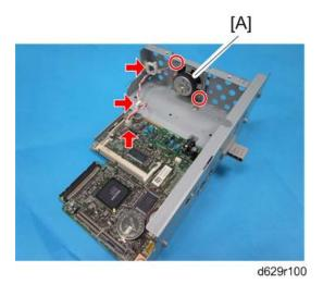
5. Remove the speaker [A] from the fax unit (  $\Re x$  2,  $\Re x$  2,  $\Re x$  1).
