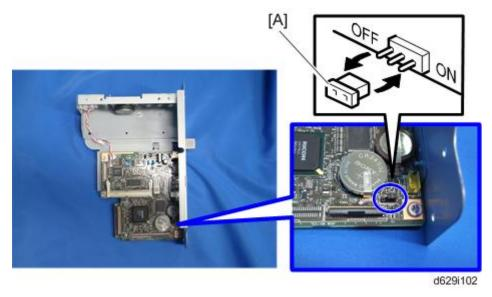
4. Move the jumper switch [A] of the new FCU board from "OFF" to "ON".
