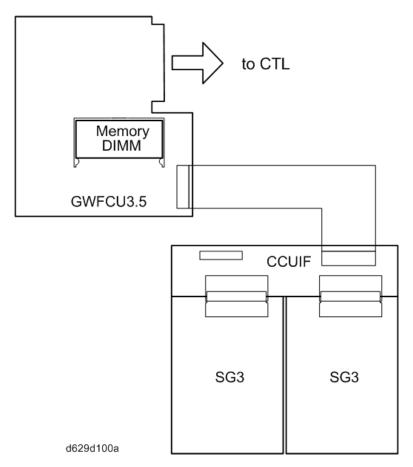
The FCU controls all the fax communications and fax features, in cooperation with the controller board. Also, the FCU contains the ROM, SRAM and NCU circuit.
