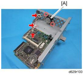
18. Install the speaker [A] in the fax unit as shown above (  $\Re x$  2,  $\Re x$  2,  $\Re x$  1).
