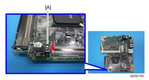
10. Move the Dip Switch [A] of the old FCU board from "OFF" to "ON".
