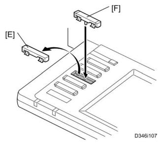
9. Remove dummy keytop [E] and replace it with the Fax keytop [F].
