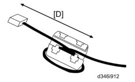
For EU models, attach the ferrite core to the telephone cord. The end of the ferrite core must be about 5 cm (2.1") [D] from the end of the cable. 8. Connect the telephone cord to the "LINE 1" jack.
