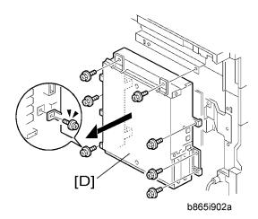
4. Remove the GDI controller box [D] if it has been installed (  $\hat{\mathscr{F}}$  x 7 ).
