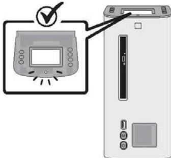
The power supply automatically senses the correct voltage. Allow startup to proceed without interruption. Do not press any buttons on the Control Panel while the system is starting.
