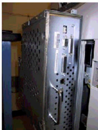
Figure 1 Front view – not fully seated
