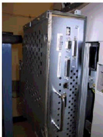
Figure 1 Front view – not fully seated
