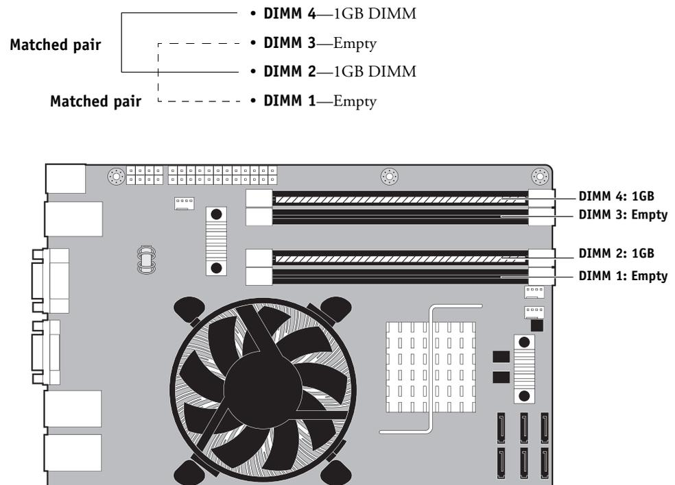
**FIGURE 23:** Motherboard DIMM sockets
