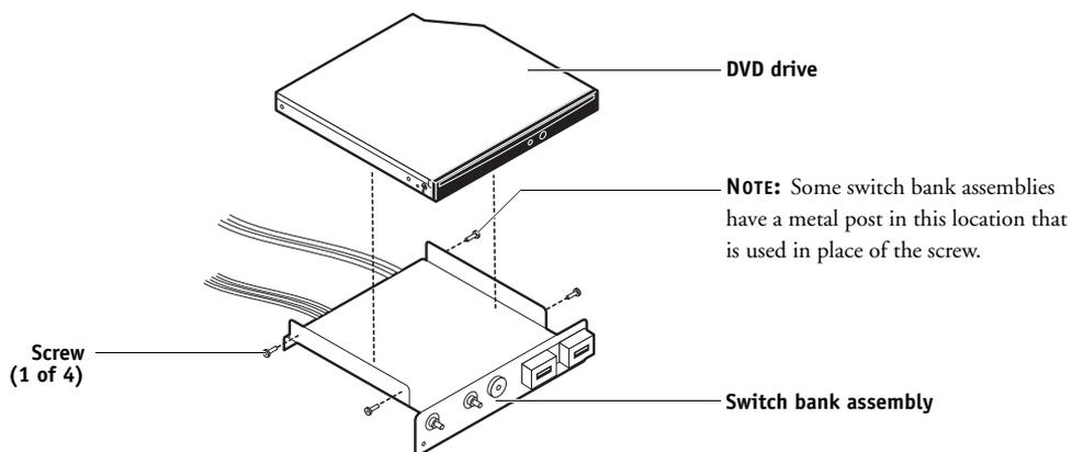
**FIGURE 38:** Removing/replacing the DVD drive
