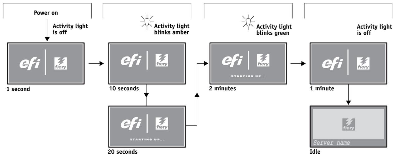
FIGURE 41: Normal startup sequence
