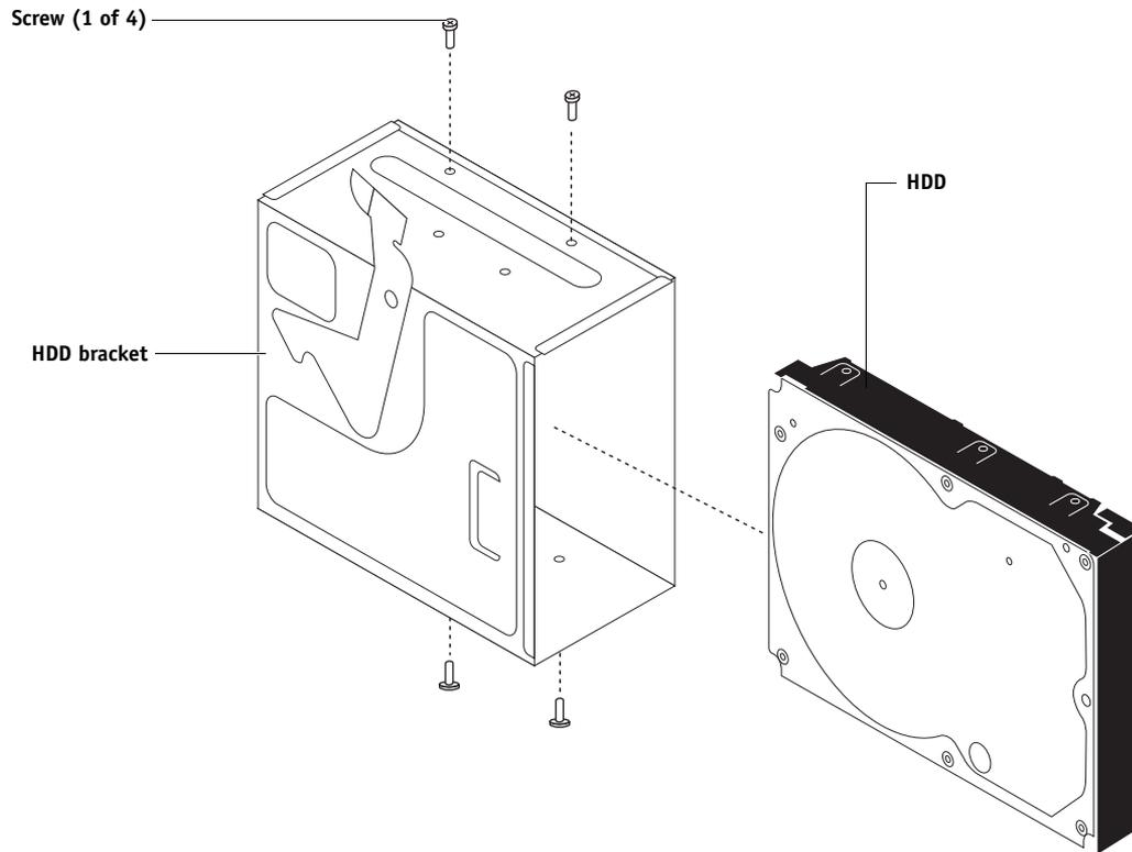
**FIGURE 33:** Removing/replacing the HDD from/in the HDD bracket
