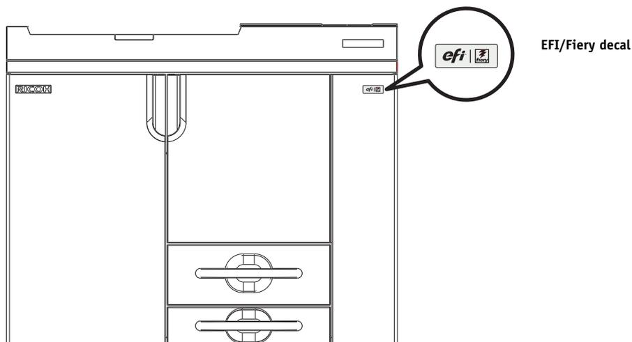
**FIGURE 5:** Affixing the decal to the copier/printer
