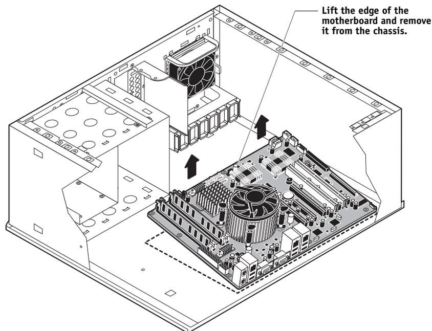
**FIGURE 21:** Removing the motherboard
