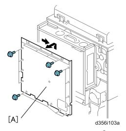
3. Remove the controller box cover [A] (earrow x 16).
