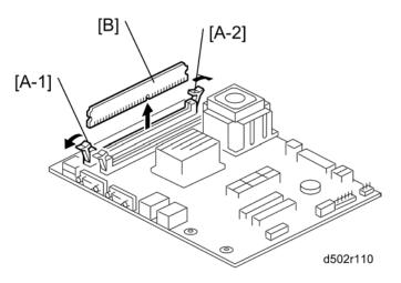
1. Push outward on the levers [A-1], [A-2] on each side of the DIMM.
