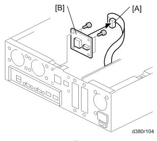
[A]: 16-pin DIAG cable (⊯ x 1) [B]: DIAG board (∦ x 4)
