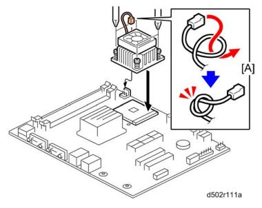
Make a loose knot [A] in the cable of the cooling assembly before connecting the cable to the motherboard.
