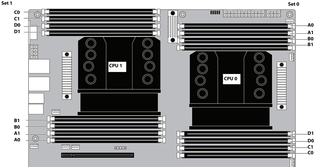
The E-85A standard configuration provides four 4GB DIMMs, for a total of 16GB of memory (Socket A0 for both Set 0 and Set 1, and Socket B0 for both Set 0 and Set 1).
