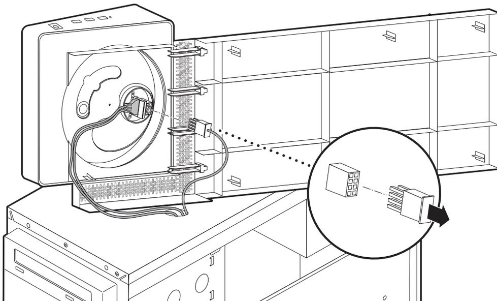
**b** Remove the two screws from the USB connector and then unplug the connector.
