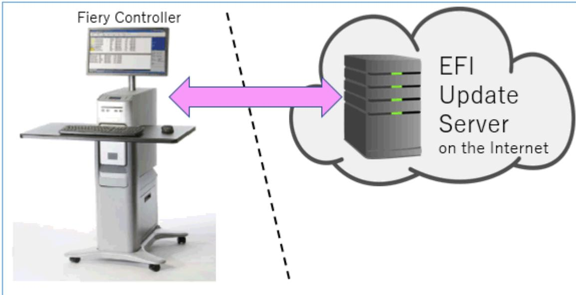
[Fiery controller (Windows or Linux model)] --(local LAN)-- [Command WorkStation on Client PC] --- (Internet) -- [EFI Update Server]
