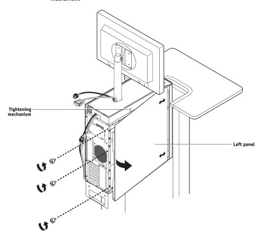
FIGURE 4: Removing the left panel
