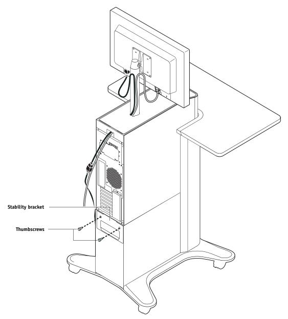
FIGURE 3: Loosening the stability bracket
