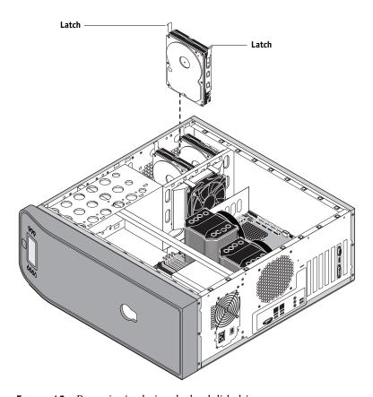
FIGURE 49: Removing/replacing the hard disk drive
