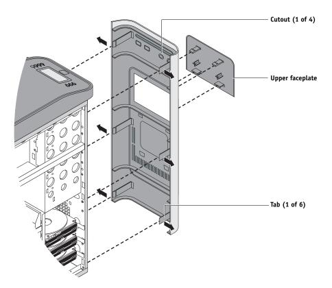
FIGURE 25: Removing/replacing the front panel
