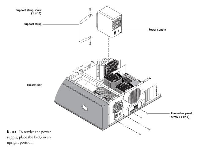
**FIGURE 47:** Removing/replacing the power supply
