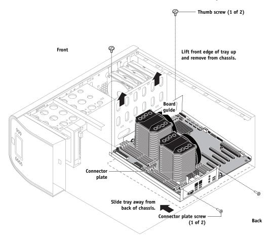
**FIGURE 34:** Removing the motherboard tray
