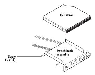
**FIGURE 53:** Removing/replacing the DVD drive
