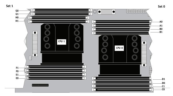
FIGURE 38: Motherboard DIMM sockets
