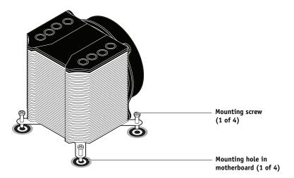
FIGURE 41: Removing/replacing the CPU cooling assembly
