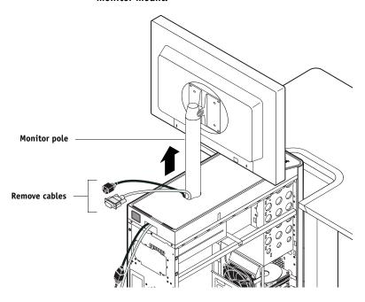
**FIGURE 6:** Removing the monitor pole assembly
