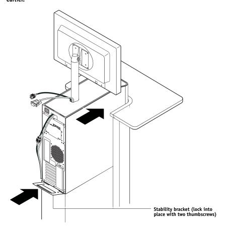
FIGURE 10: Locking the stability bracket
