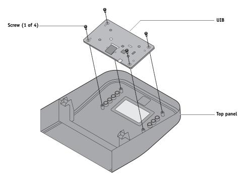
FIGURE 31: Removing/replacing the user interface board
