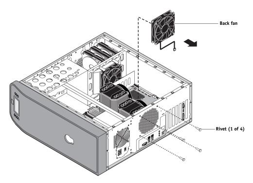
FIGURE 45: Removing/replacing the back fan
