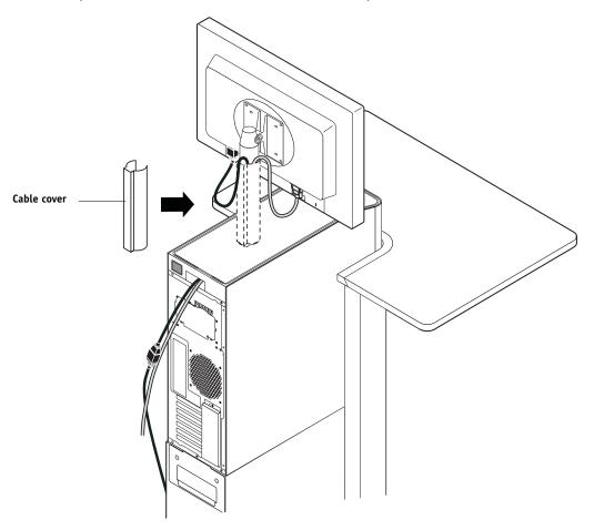
FIGURE 11: Installing the cable cover
