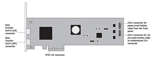
**FIGURE 27:** Printer interface board (component side)
