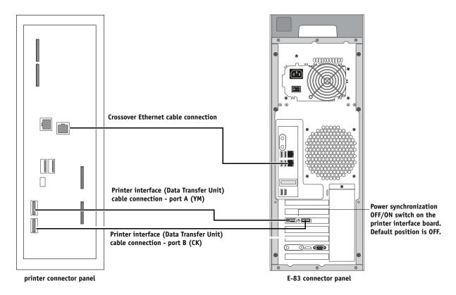
FIGURE 5: Printer and E-83 cable connection
