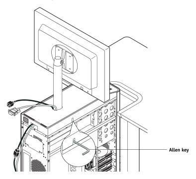
FIGURE 5: Loosening the monitor pole
