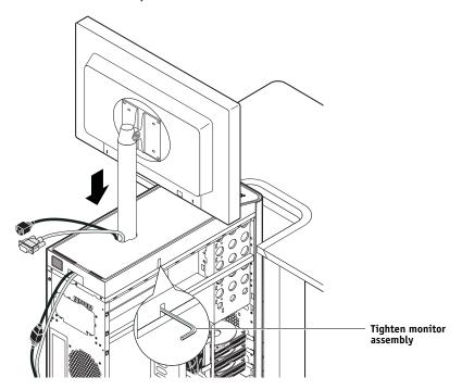
FIGURE 8: Tightening the monitor pole assembly
