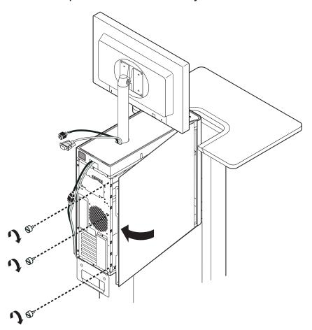
FIGURE 9: Installing the left panel
