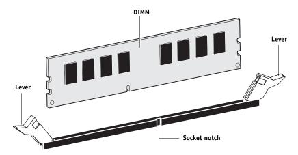
FIGURE 39: Releasing a DIMM
