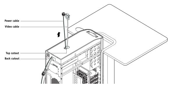
FIGURE 7: Routing the cables through the access cutout
