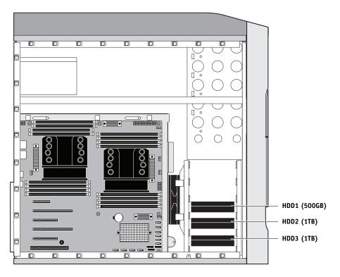
FIGURE 48: E-83 hard disk drives (HDDs)
