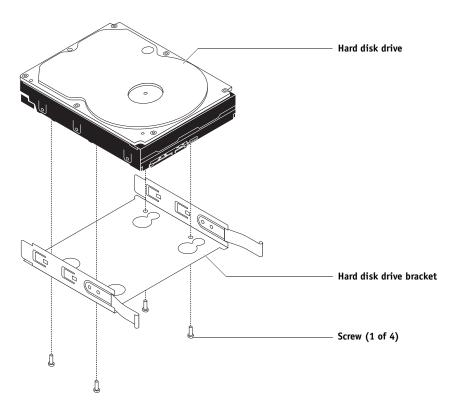
FIGURE 50: Removing/replacing the hard disk drive bracket
