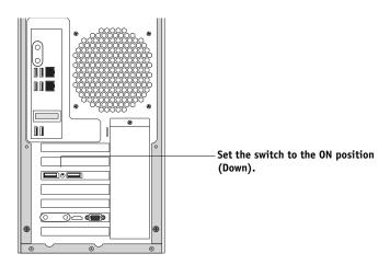
FIGURE 16: Power synchronization switch
