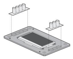
**FIGURE 32:** Removing/replacing the UIB buttons
