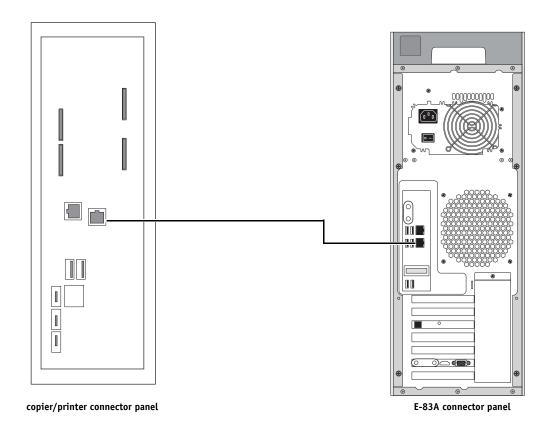
**FIGURE 5:** Copier/printer and E-83A cable connection
