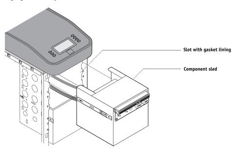
FIGURE 51: Removing/replacing the component sled
