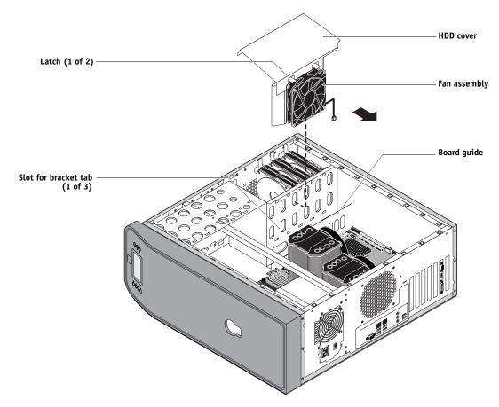
FIGURE 43: Removing/replacing the front fan assembly
