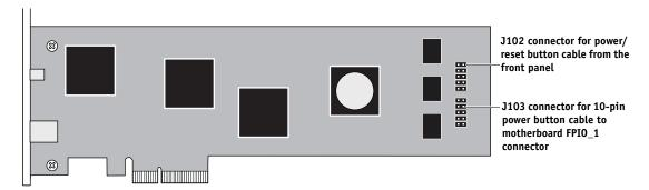
FIGURE 27: Printer interface board (component side)
