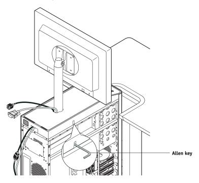
FIGURE 5: Loosening the monitor pole
