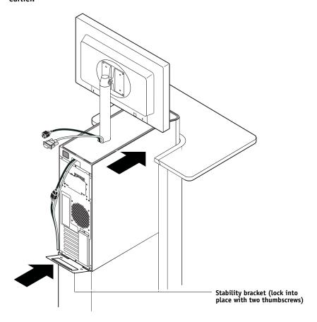
FIGURE 10: Locking the stability bracket
