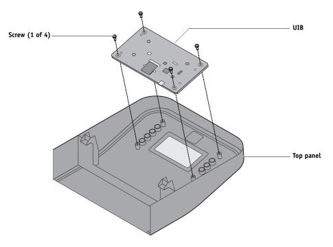
FIGURE 31: Removing/replacing the user interface board
