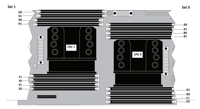
FIGURE 38: Motherboard DIMM sockets
