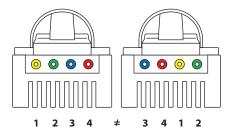
Crossover cable: wire arrangements are different (The wire arrangement shown here is an example; actual arrangements may vary.)
