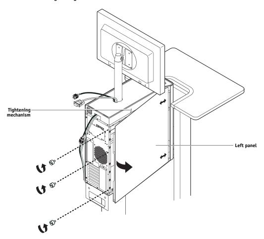
FIGURE 4: Removing the left panel
