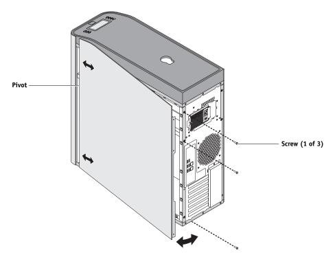
FIGURE 23: Removing/replacing the right panel
