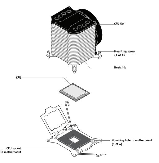
FIGURE 40: CPU, socket, and cooling assembly
