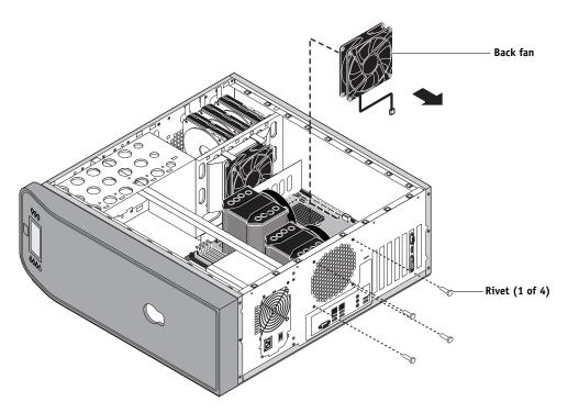
FIGURE 45: Removing/replacing the back fan
