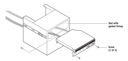
FIGURE 52: Removing/replacing the switch bank assembly
