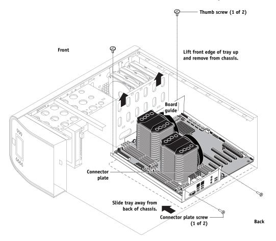
**FIGURE 34:** Removing the motherboard tray
