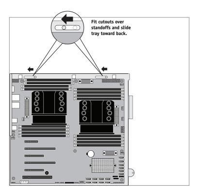
FIGURE 36: Installing the motherboard tray
