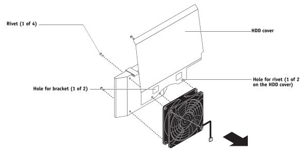
FIGURE 44: Removing/replacing the front fan and HDD cover from the bracket
