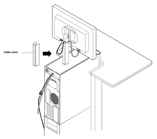
FIGURE 11: Installing the cable cover
