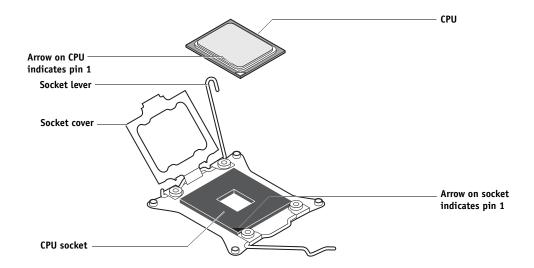
FIGURE 42: Replacing a CPU
