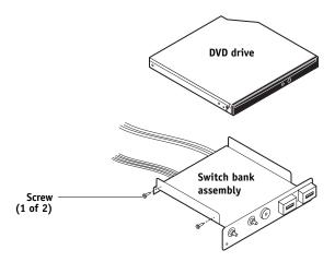
**FIGURE 53:** Removing/replacing the DVD drive
