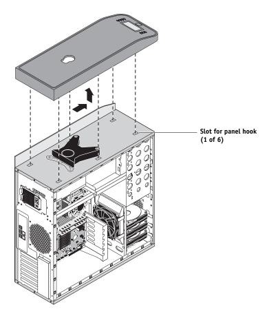
FIGURE 26: Removing/replacing the top panel
