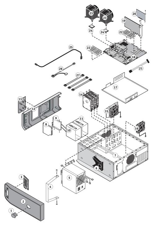
FIGURE 20: Exploded view of the E-83A
