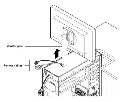
**FIGURE 6:** Removing the monitor pole assembly
