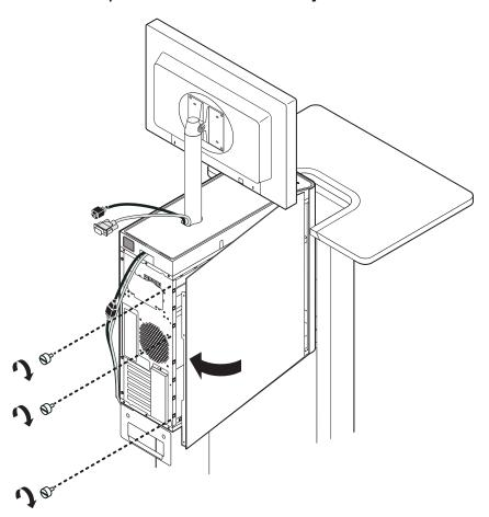
**FIGURE 9:** Installing the left panel
