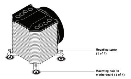
FIGURE 41: Removing/replacing the CPU cooling assembly
