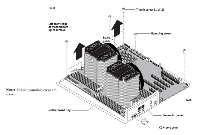
FIGURE 35: Removing the motherboard from the tray
