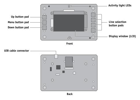
**FIGURE 30:** Diagram of the user interface board (front and back)
