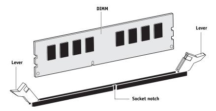
FIGURE 39: Releasing a DIMM
