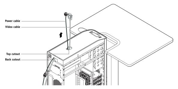
FIGURE 7: Routing the cables through the access cutout
