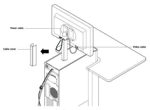
**FIGURE 2:** Removing the cable cover and monitor cables
