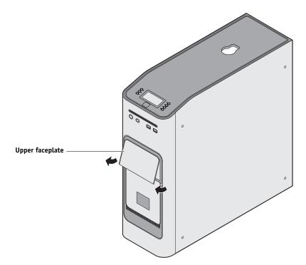
FIGURE 24: Removing the upper faceplate
