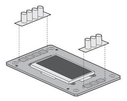
**FIGURE 32:** Removing/replacing the UIB buttons
