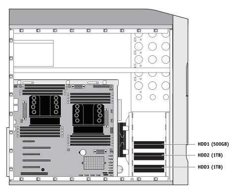
FIGURE 48: E-83A hard disk drives (HDDs)
