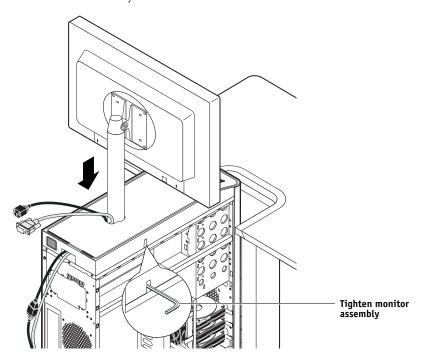
FIGURE 8: Tightening the monitor pole assembly
