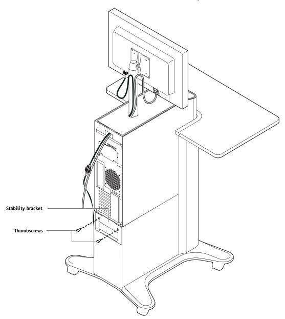
FIGURE 3: Loosening the stability bracket
