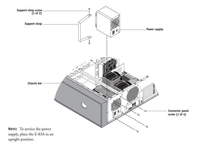
**FIGURE 47:** Removing/replacing the power supply
