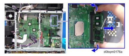
4. Insert the 4GB DIMM into SDRAM socket.
