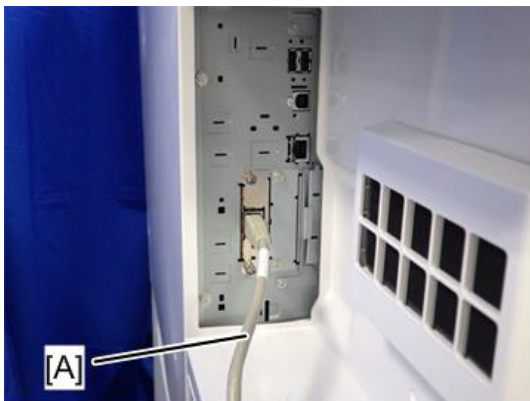
Figure 41: Connecting the interface cable to the printer.
