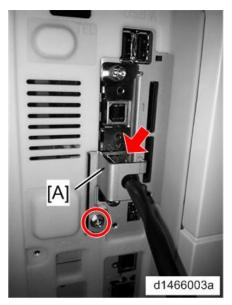
2. Remove the Gigabit Ethernet controller [A] (knob-screw x 2).
