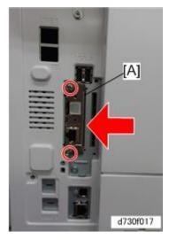
Connect the interface cable to the copier Gigabit Ethernet connector and then fix it with the protection plate [A] (\$\$\vert\$x 1).
