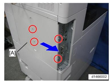
5. Remove the Gigabit Ethernet controller [A] as shown. (🕮 x 1, 🌮 x 2).
