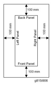
Place the machine near the power source, providing clearance as shown.
