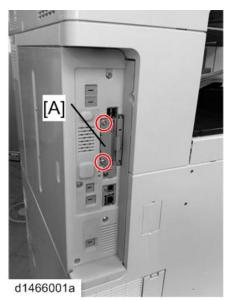
3. Insert the Gigabit Ethernet controller [A] and fasten it (knob-screw x 2).
