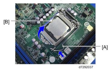
2. Grasp the CPU [A] by its edges and gently lift it from the socket.
