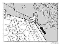
Fasten the duplex feed unit using a short screw and the provided screwdriver.
