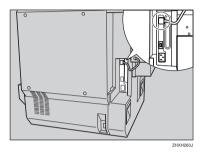
This completes installation of the duplex reversal unit. Install the duplex feed unit after the external tray.
