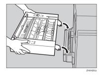
The hooks of the duplex reversal unit clip around the bar inside the groove of the stand.
