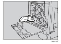
Holding the duplex feed unit using both hands, place it on the vertical rail, and then slide it slowly in until it stops.
