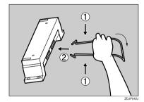
Insert the claws of the stand into the holes on the left side of the printer  $(\widehat{1})$ , and then push down  $(\widehat{2})$ .
