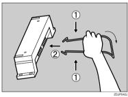
Insert the claws of the stand into the holes on the left side of the printer (1), and push down (2).
