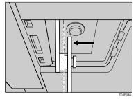
In step **5**, move the auxiliary bar to the position shown with a perforated line in the illustration.
