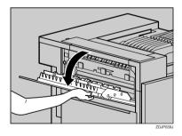
2 Pinch the two small covers and pull in the direction of the arrow to remove them.
