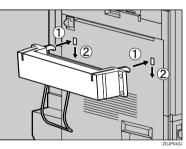
Open the front cover slowly by pulling the two points on the left and right.
