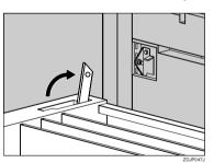
Hook the hole of the auxiliary bar on the mounting bracket of the printer.
