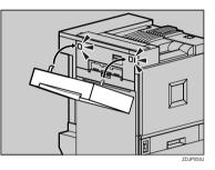
Remove the adhesive tape which hold the cable, and then connect the cable of the Duplex Reversal Unit to the upper connector on the back of the printer.
