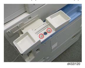
8. Attach the cradle to the handset bracket (  $\mbox{\ensuremath{\beta}}\mbox{\ensuremath{x}} \times 2 \colon \mbox{\ensuremath{M3}}\mbox{\ensuremath{x8}}\mbox{\ensuremath{)}}.$
