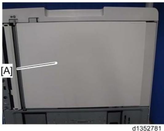
2. Put the white guide [A] in the correct position on the exposure glass, aligning it with the glass cover
