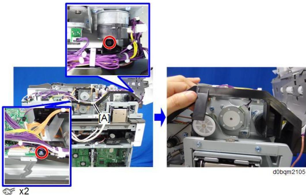
3. Remove the timing belt, and then remove the ADF pick-up roller lift motor (M1) [A].
