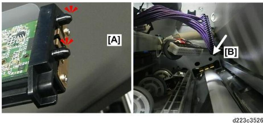
**3.** To re-install the CIS, set the CIS in its channel so it is perfectly flat.
