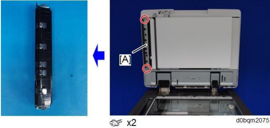
2. Remove the scanning guide plate [A].
