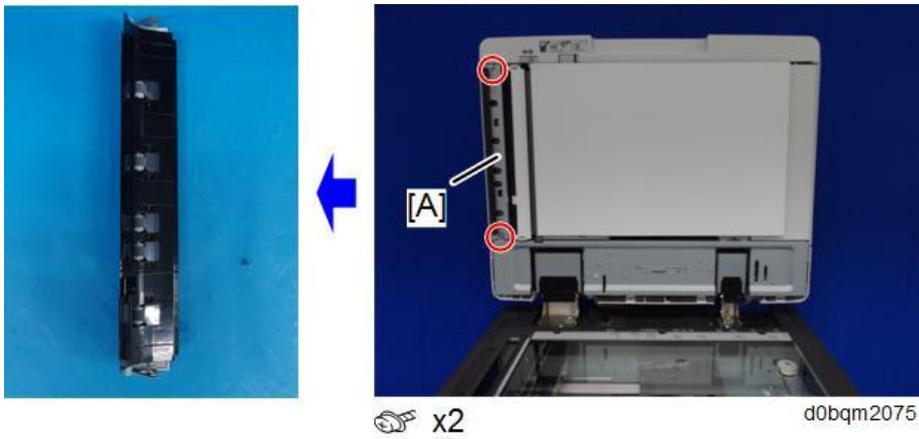
2. Remove the scanning guide plate [A].
