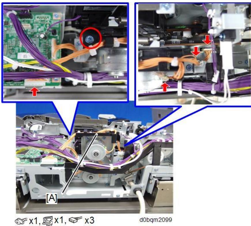
3. Remove the timing Belt, and then remove the pull-out motor (M4) [A] along with the bracket.
