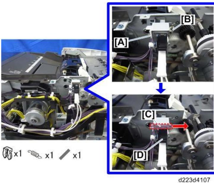
4. Remove the ADF feed cover interlock switch (SW1) [A].
