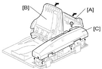
2. Remove the front cover [A] (screw x1).
