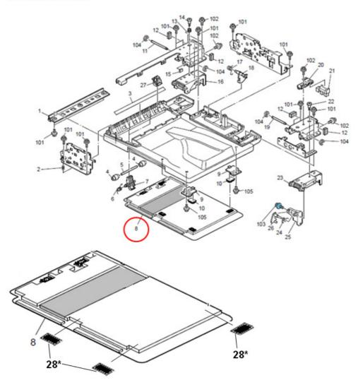
**Note:** Index 8 (PRESSURE PLATE ASS'Y) does not include index 28\* (TAPE - PLATEN SHEET).
