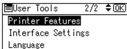
**3** Select the desired item using the [▲] or [▼] key, press the [OK] key, and then change its settings.
