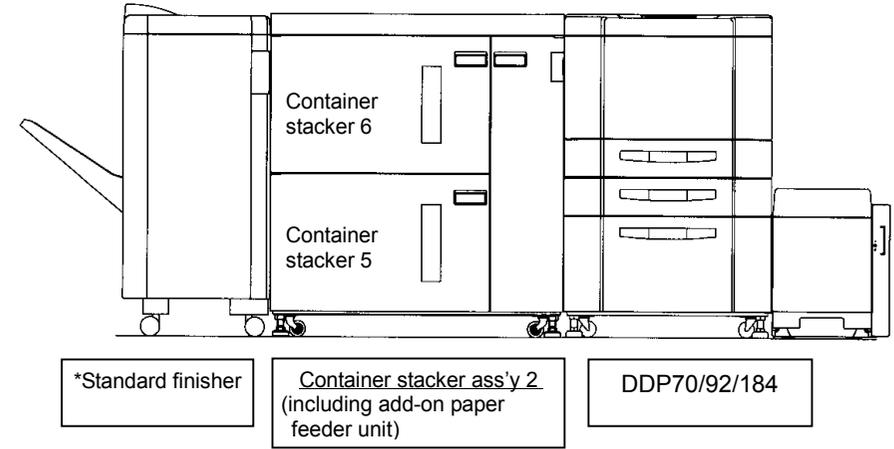
(2) DDP70/92/184 + Container stacker ass'y 1 (including sample tray) + Container stacker ass'y 2 (including add-on paper feeder unit)
