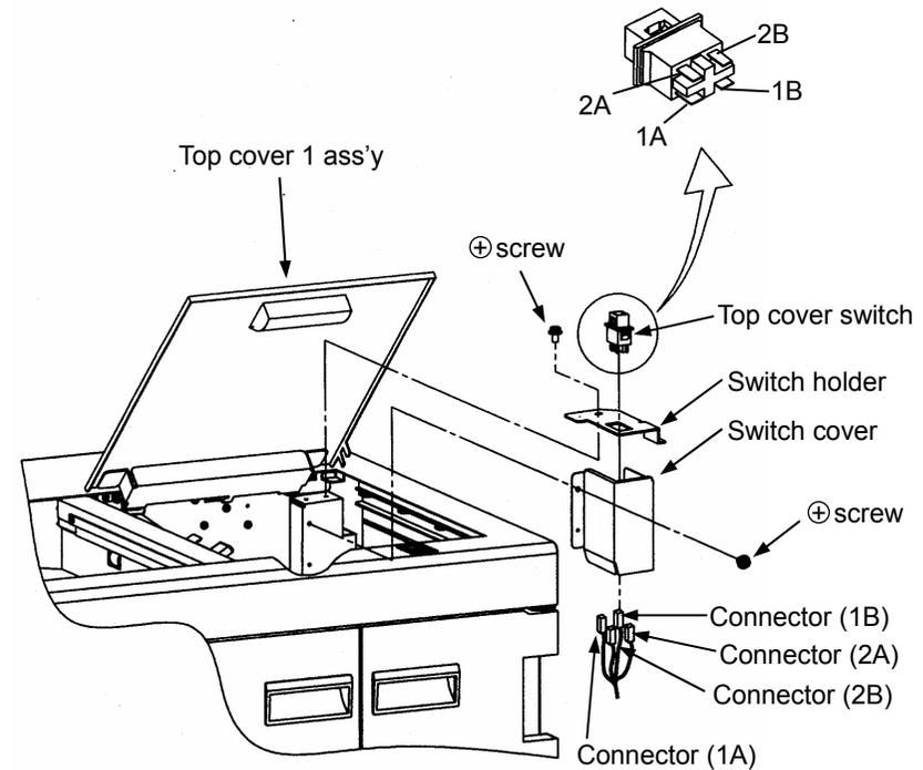
Fig. 6-122. Removal of the top cover switch
