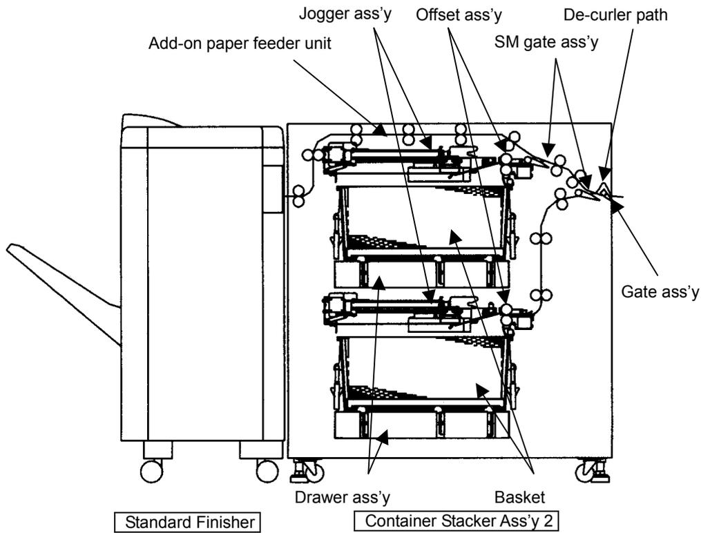
Fig 8-3 View of the Center Cross Section of Container Stacker Ass'y 2 + Standard Finisher
