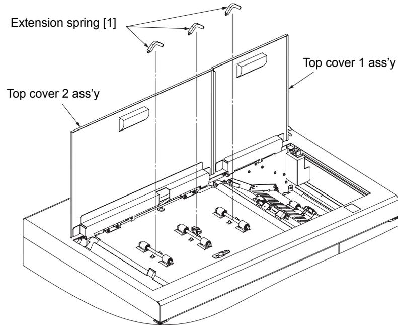
Fig. 6-101. Removal of the extension spring [1] (upper)
