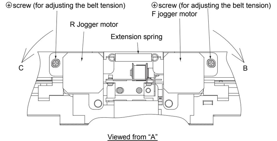
Fig. 6-12. Removal of the timing belt (front/rear) U/L
