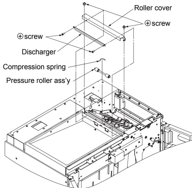
Fig. 6-90. Removal of the pressure roller ass'y and the compression spring
