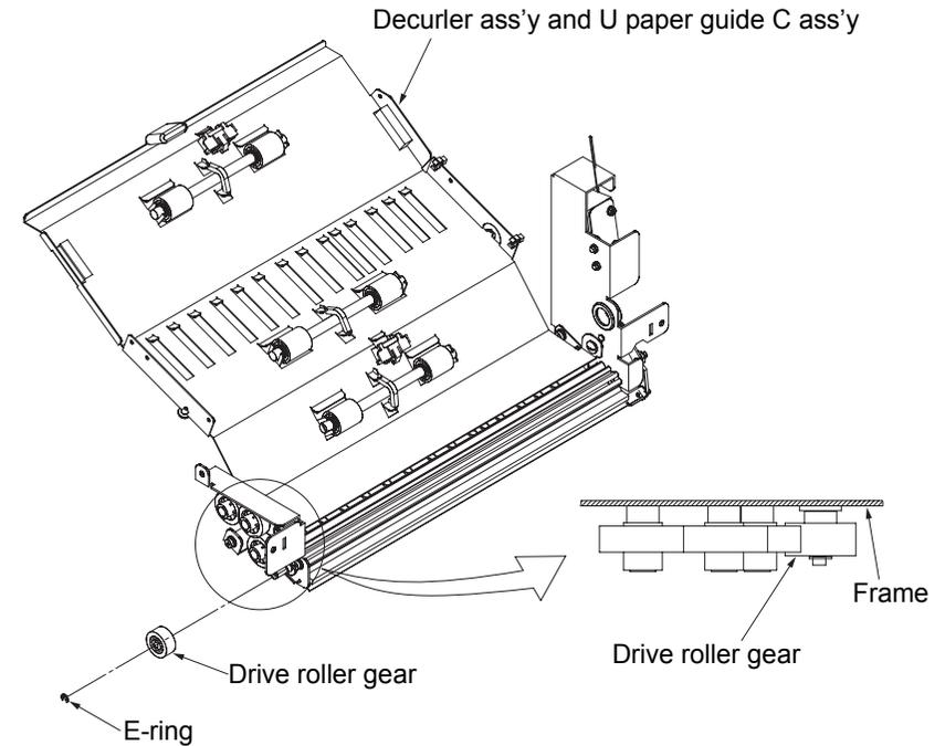
Fig. 6-58 Removal of the drive roller gear
