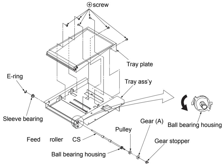
Fig. 6-96. Removal of the feed roller CS ass'y
