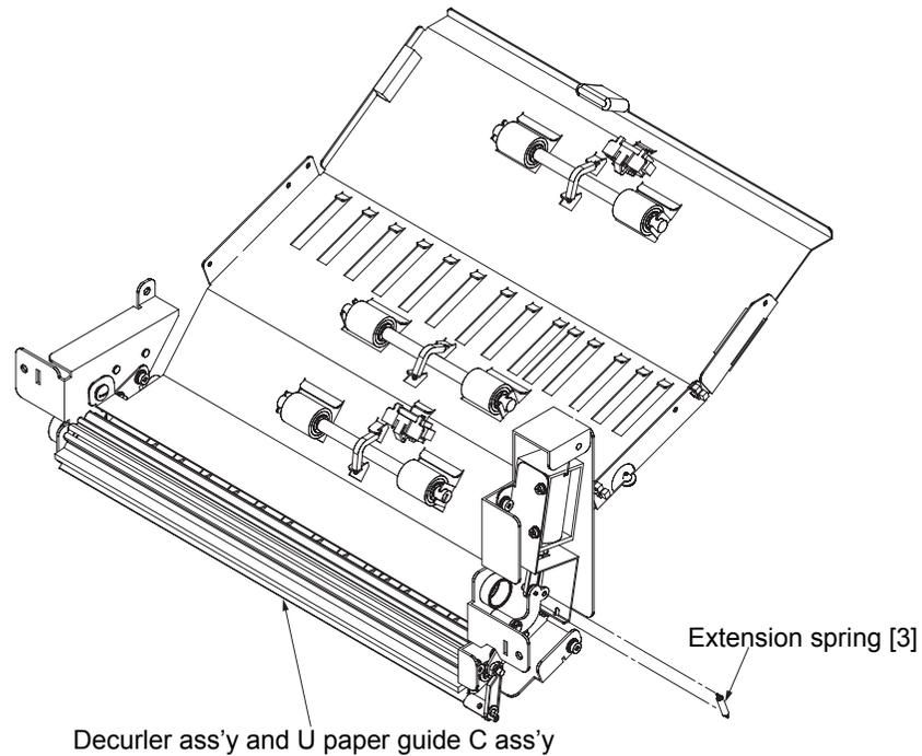
Fig. 6-59 Removal of the extension spring [3]
