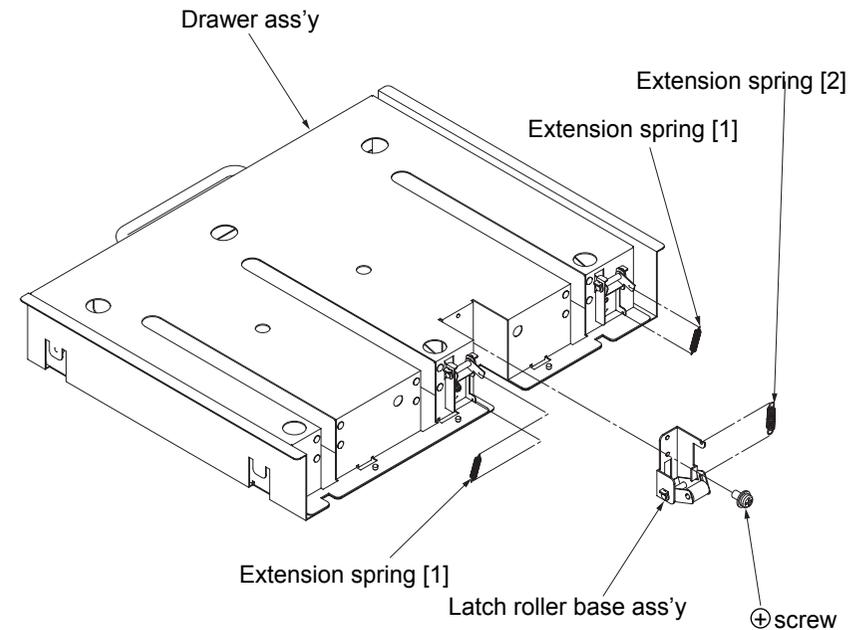
Fig. 6-118. Removal of the extension springs [1] and [2] U/L
