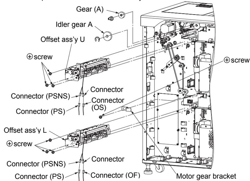
Fig. 6-74. Removal of the offset ass'y U/L
