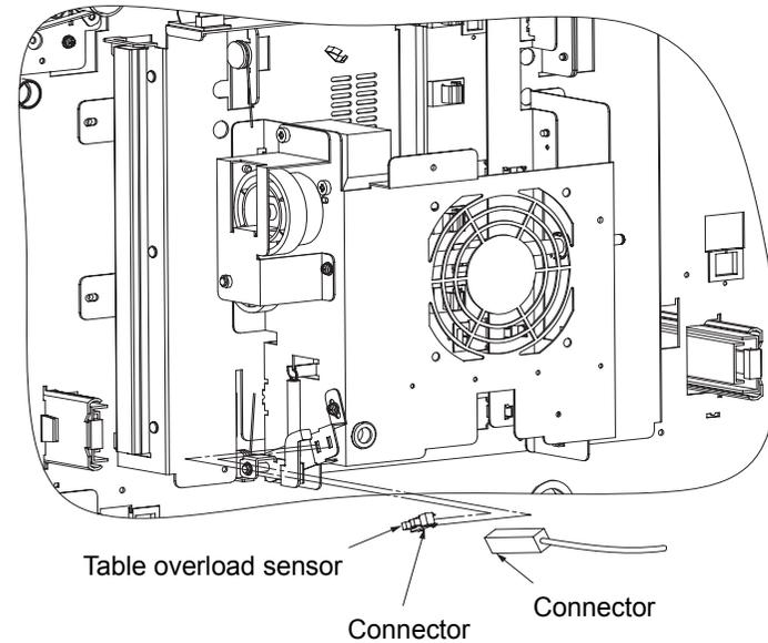
Fig. 6-26. Removal of the table overload sensor U/L
