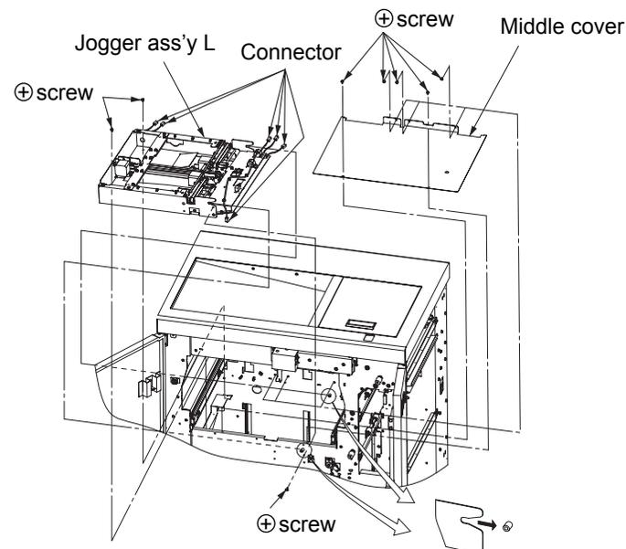
Fig.6-2. Removal of the jogger ass'y L
