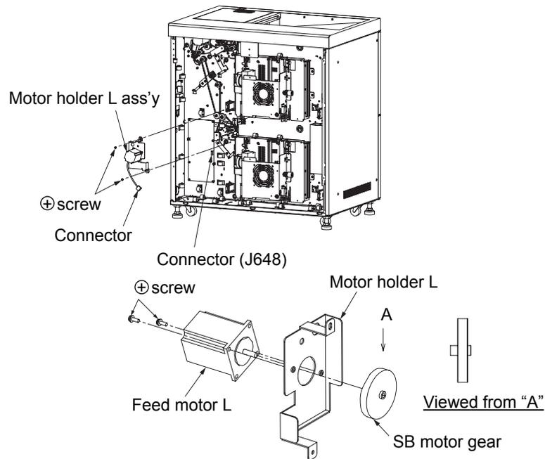
Fig. 6-49. Removal of the feed motor L and the SB motor gear
