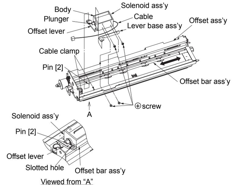
Fig. 6-87. Removal of the solenoid ass'y U/L
