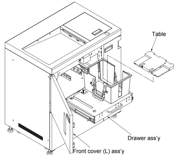
Fig. 6-132. Removal of the table U/L
