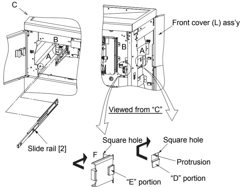
Fig. 6-137. Removal of the slide rail [2] U/L
