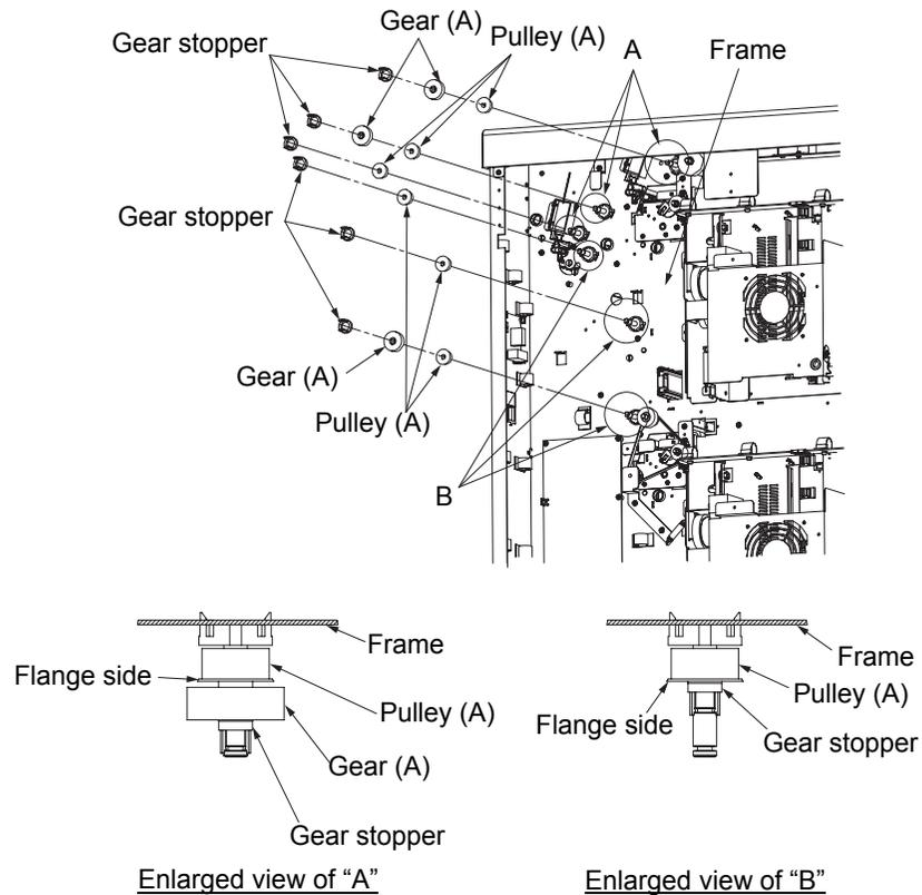
Fig. 6-55. Removal of the pulley (A)
