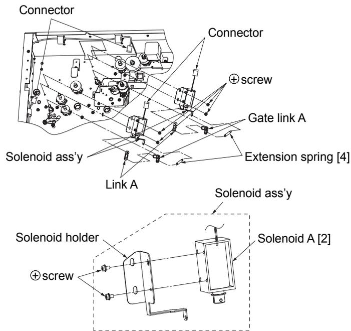
Fig. 6-69. Removal of the solenoid A [2]
