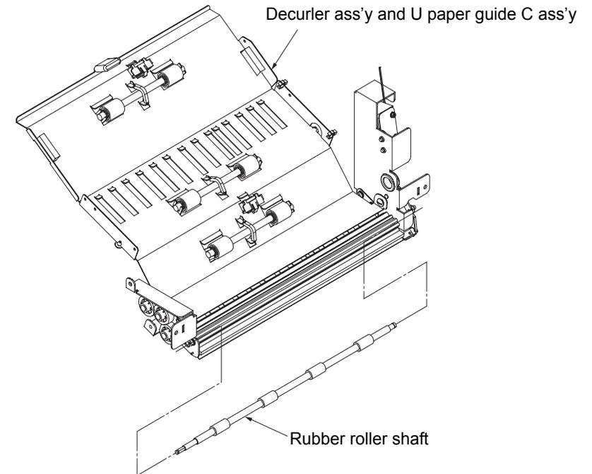
Fig. 6-64. Removal of the rubber roller shaft
