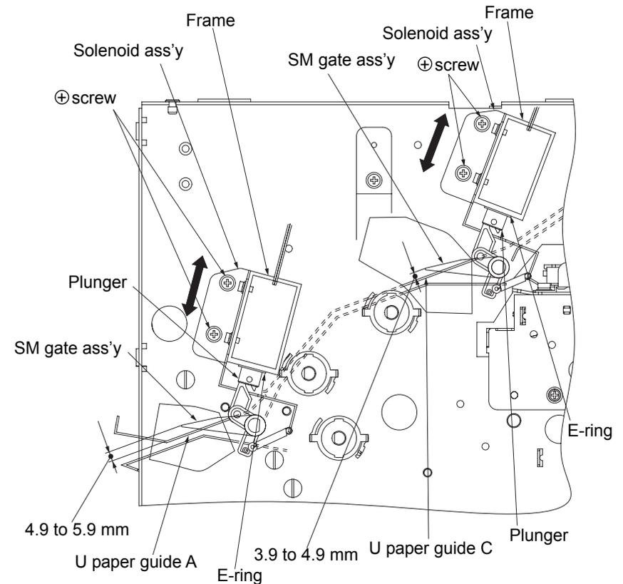
Fig. 6-70. Installation of the solenoid A [2]
