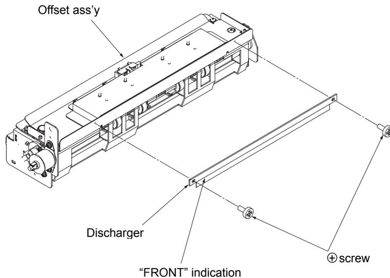
Fig. 6-78. Removal of the discharger U/L
