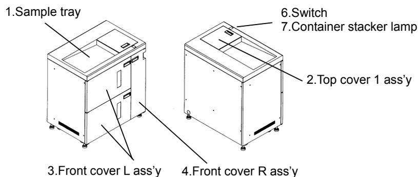
Fig. 3-1. External view of Container Stacker Ass'y 1
