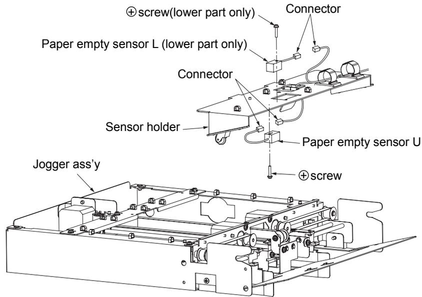
Fig. 6-9. Removal of the paper empty sensor U/L
