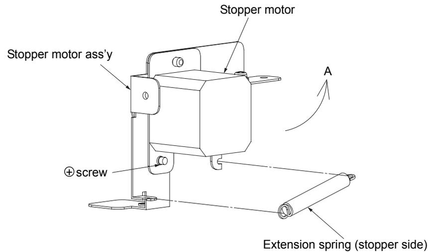
Fig. 6-23. Removal of the extension spring (stopper side) U/L
