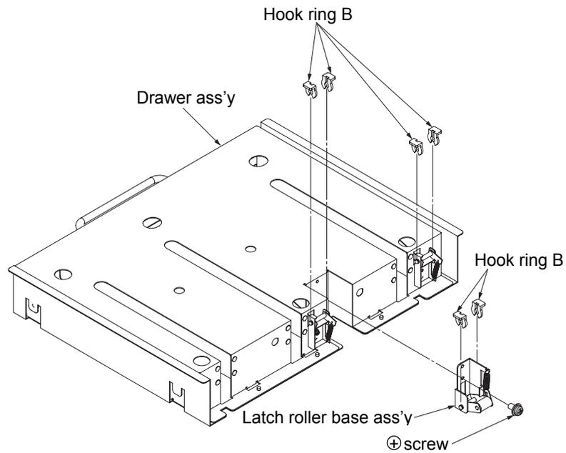
Fig. 6-117. Removal of the hook ring B U/L
