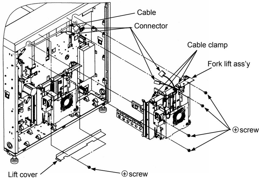
Fig. 6-25. Removal of the fork lift ass'y U/L
