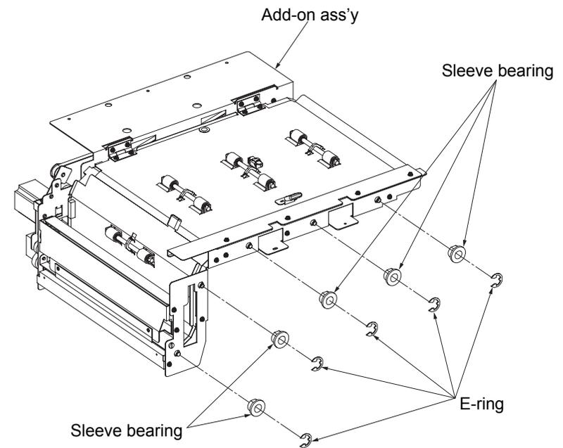
Fig. 6-106. Removal of the sleeve bearing
