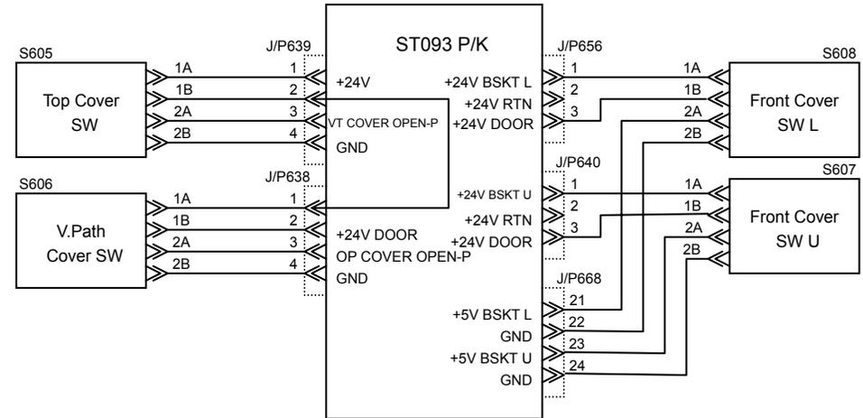
Fig. 5-3 Error codes E02D, E03B, E02E, E03A, E03C, E03D, E038 and E039
