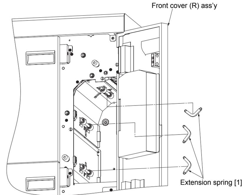
Fig. 6-40. Removal of the extension spring [1] (lower)
