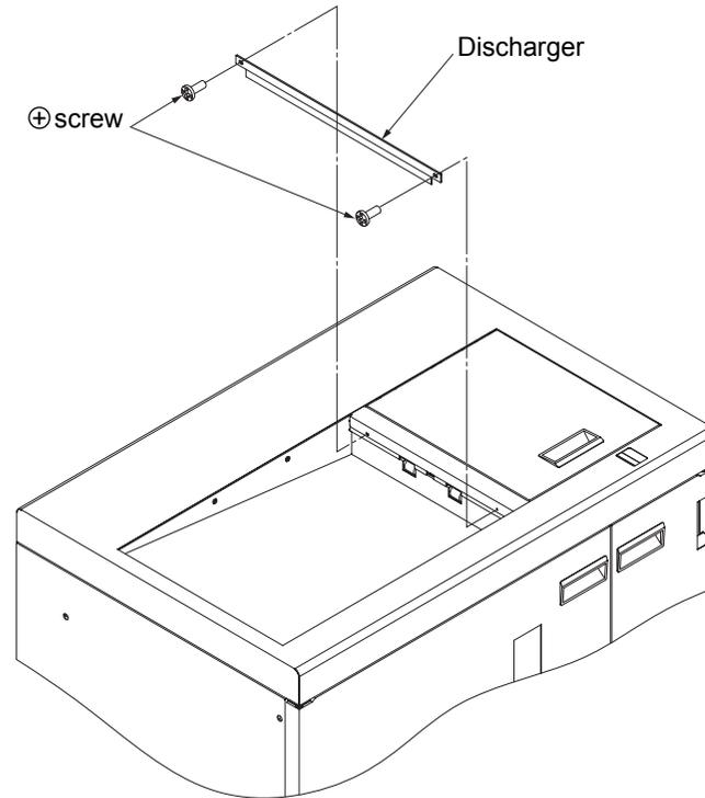
Fig. 6-89. Removal of the discharger
