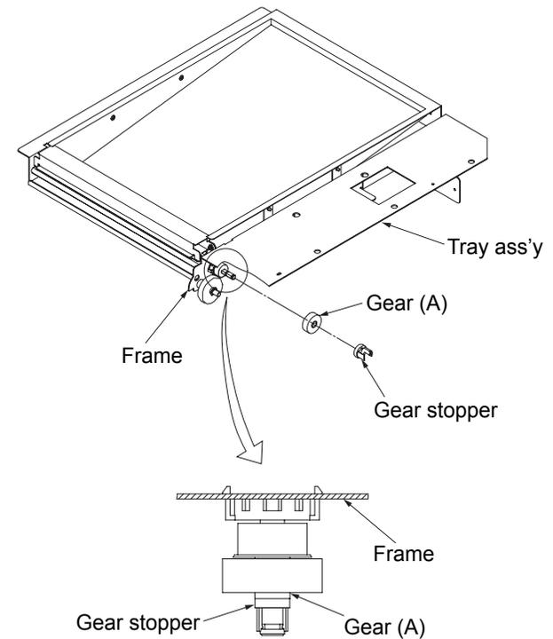
Fig. 6-93. Removal of the gear (A)
