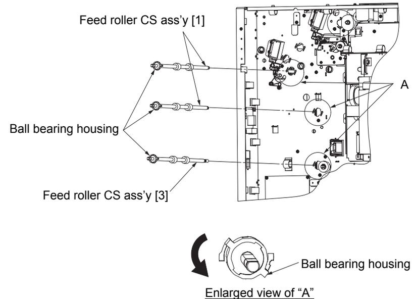
Fig. 6-68. Removal of the feed roller CS assemblies [1] (lower side) and [3]
