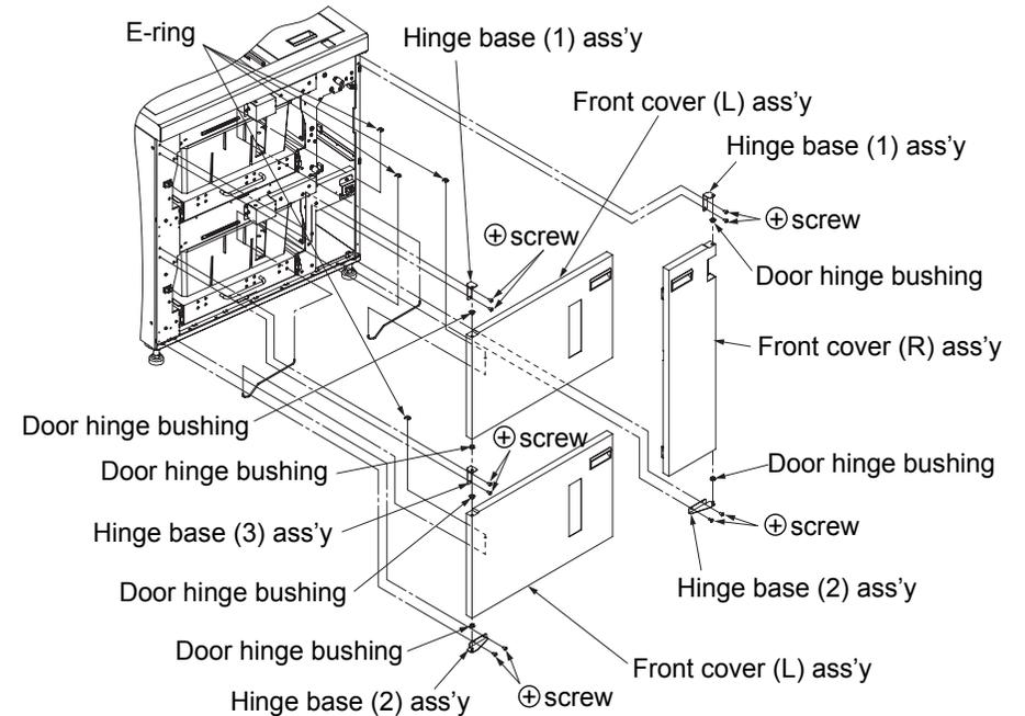
Fig. 6-130. Removal of the door hinge bushing
