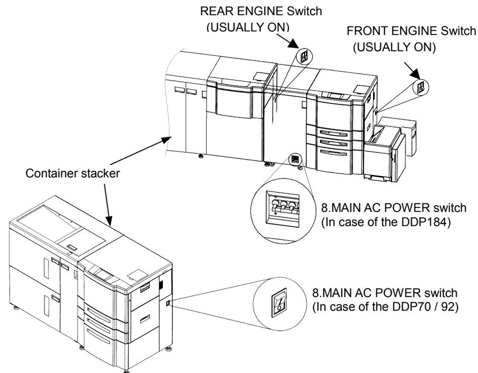
Fig. 3-3. Location of the MAIN AC POWER switch
