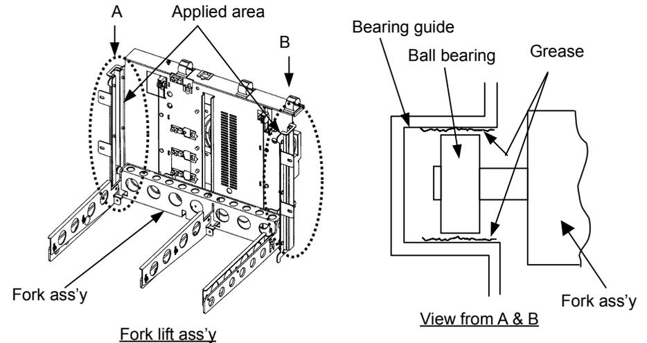
Fig. 4-1. Cleaning of bearing guide
