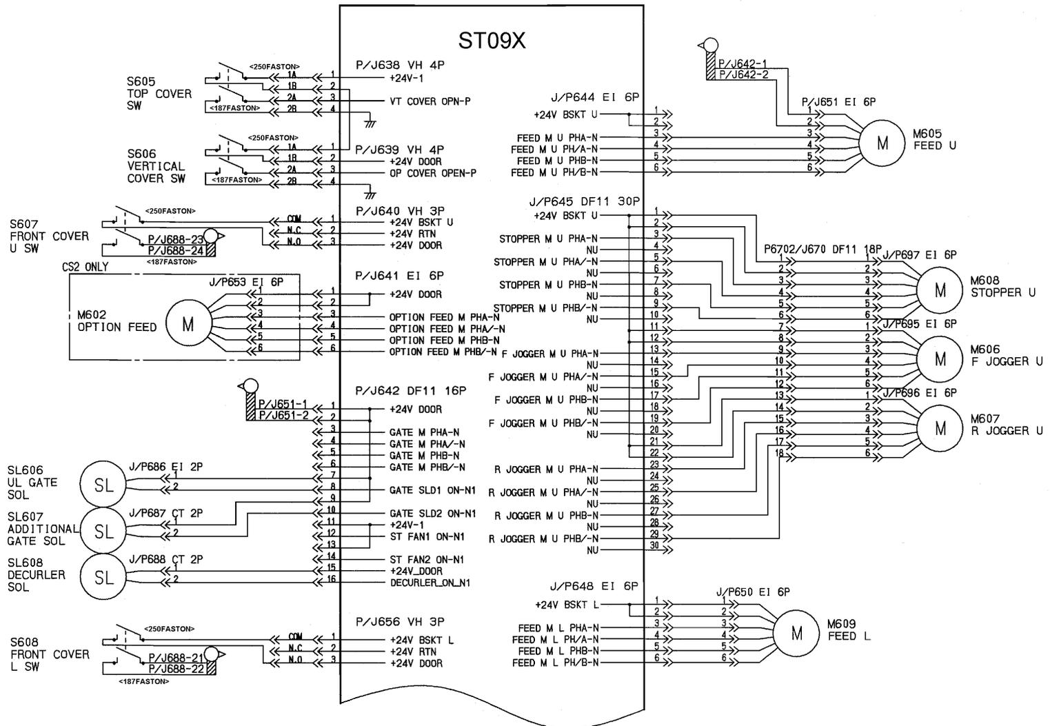
Figure 3-13 Block Wiring
