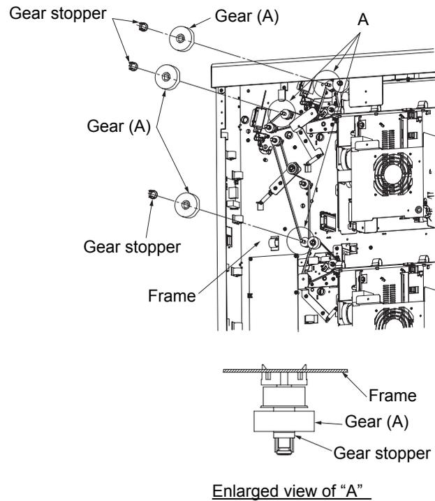
Fig. 6-51. Removal of the gear (A)
