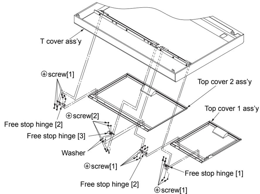
Fig. 6-131. Removal of the free stop hinges [1], [2] and [3]
