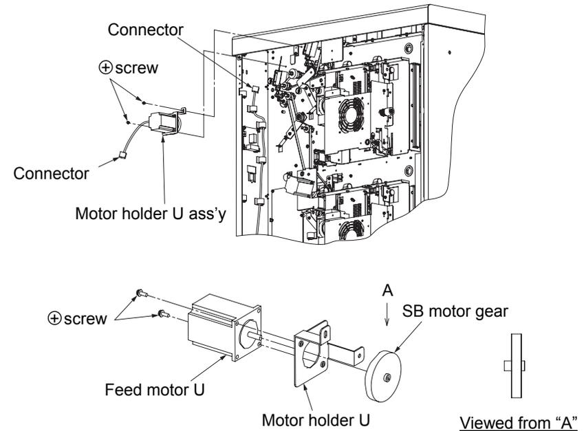
Fig. 6-48. Removal of the feed motor U and the SB motor gear
