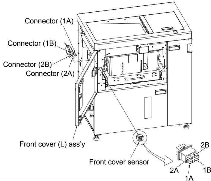
Fig. 6-127. Removal of the front cover sensor U/L
