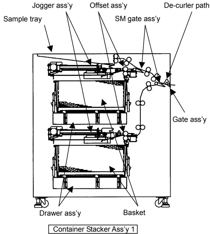
Fig 8-1 View of the Center Cross Section of Container Stacker Ass'y 1
