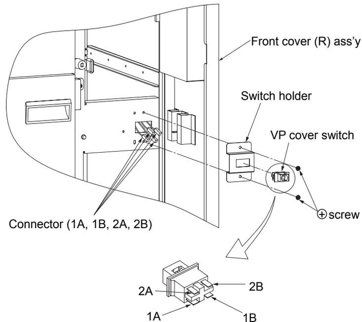
Fig. 6-125. Removal of the VP cover switch
