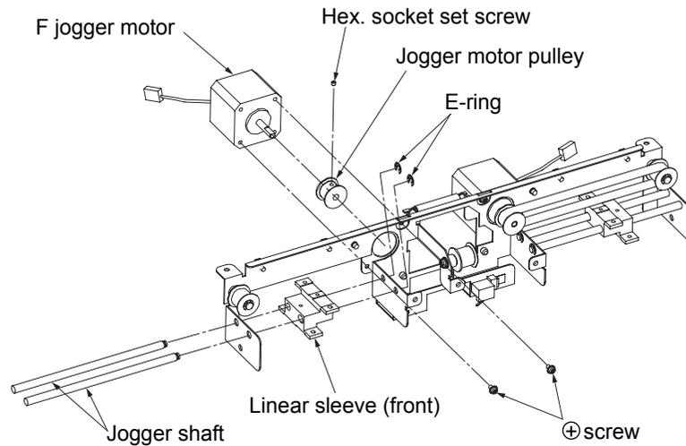
Fig. 6-21. Removal of the F jogger motor U/L
