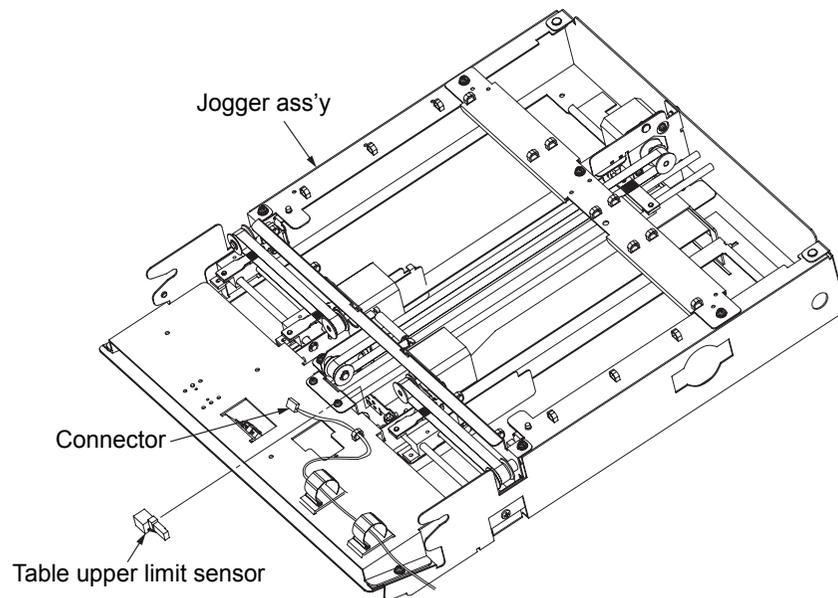
Fig. 6-7. Removal of the table upper limit sensor U/L
