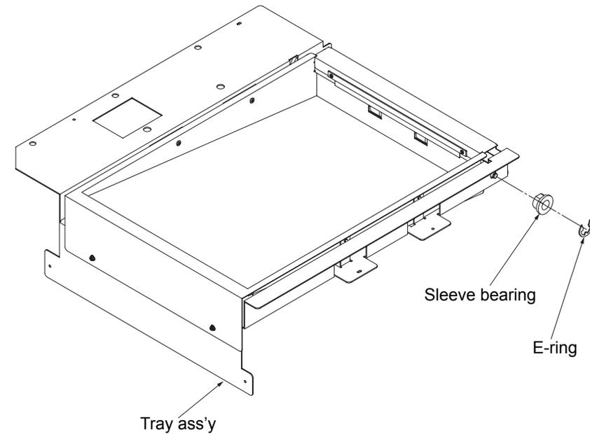
Fig. 6-95. Removal of the sleeve bearing
