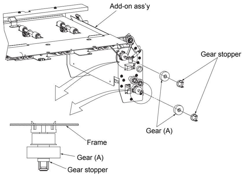
Fig. 6-109. Removal of the gear (A)
