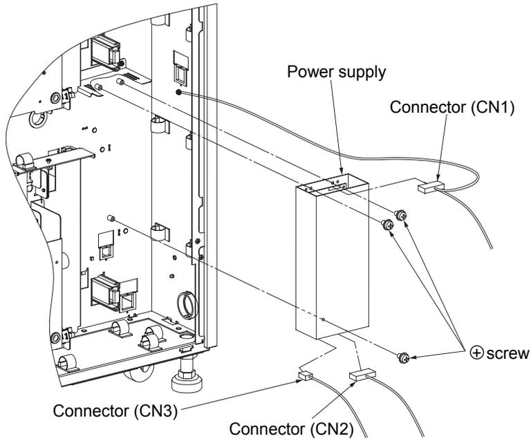
Fig. 6-119. Replacement of the power supply
