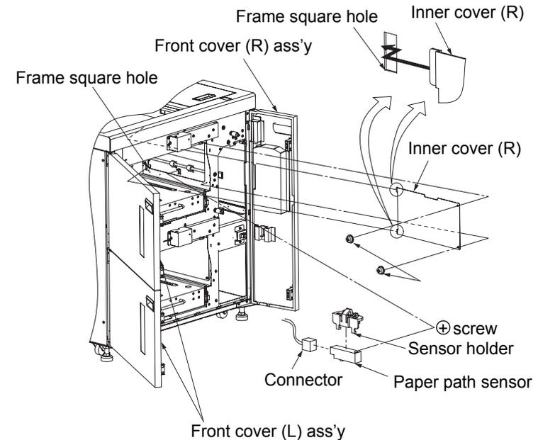
Fig. 6-44. Removal of the paper path sensor (lower) and the sensor holder
