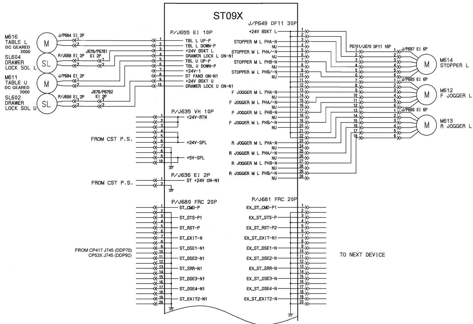
Figure 3-14 Block Wiring
