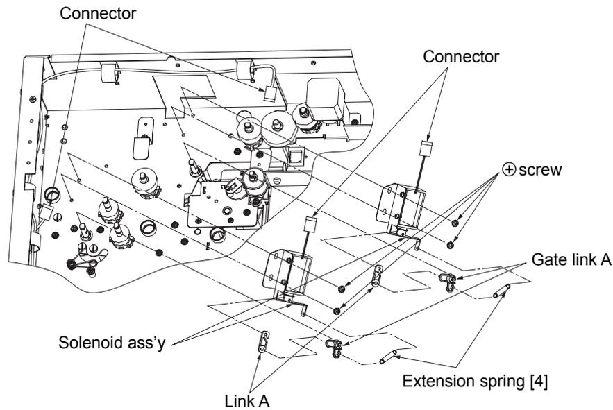
Fig. 6-71. Removal of the extension spring [4]
