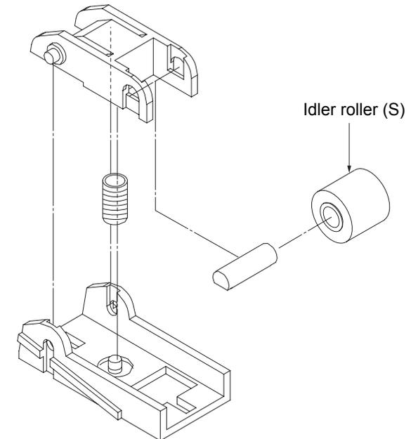
Fig. 6-83. Removal of the idler roller (S) U/L
