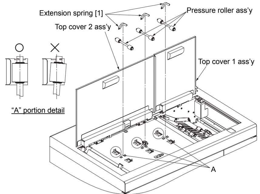
Fig. 6-102. Removal of the pressure roller ass'y (upper)
