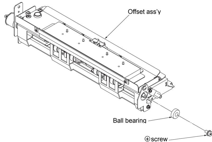
Fig. 6-81. Removal of the ball bearing U/L
