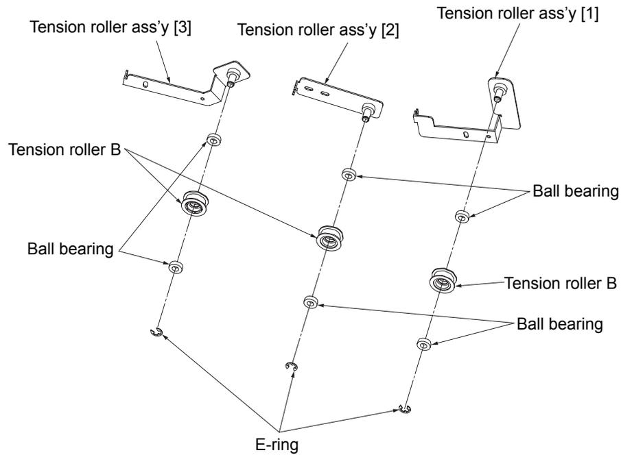
Fig. 6-53. Removal of the tension roller B and the ball bearing
