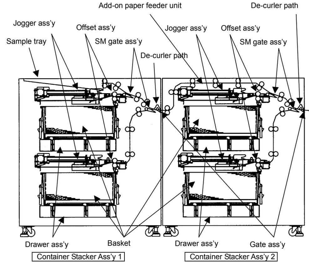
Fig 8-2 View of the Center Cross Section of Container Stacker Ass'y 1 + 2
