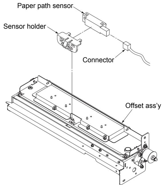
Fig. 6-80. Removal of the paper path sensor and sensor holder U/L
