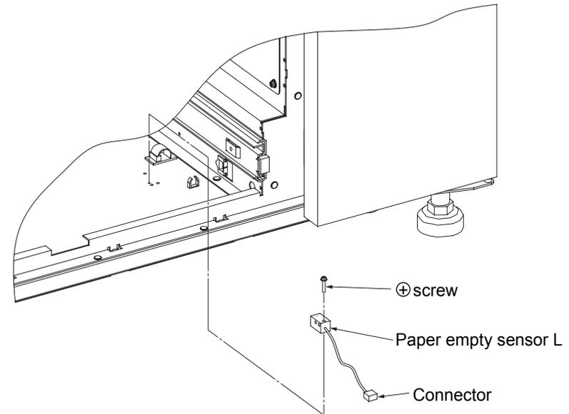
Fig. 6-124. Removal of the paper empty sensor L
