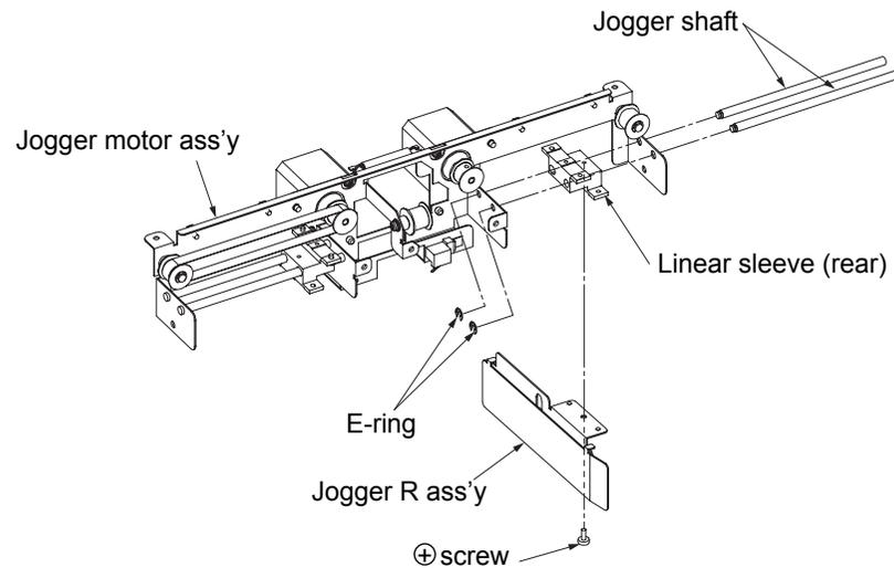
Fig. 6-19. Removal of the linear sleeve (rear) U/L
