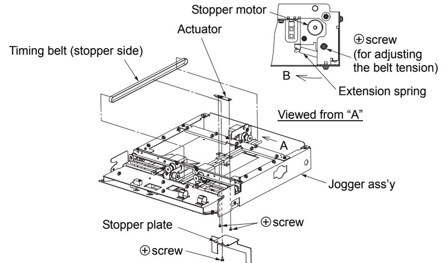
Fig. 6-10. Removal of the timing belt (stopper side) U/L
