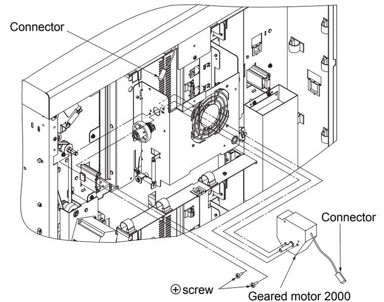
Fig. 6-30. Removal of the geared motor 2000 U/L
