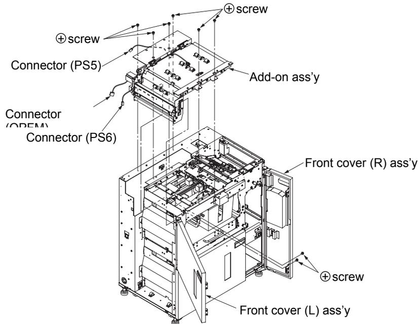
Fig. 6-97. Removal of the add-on ass'y
