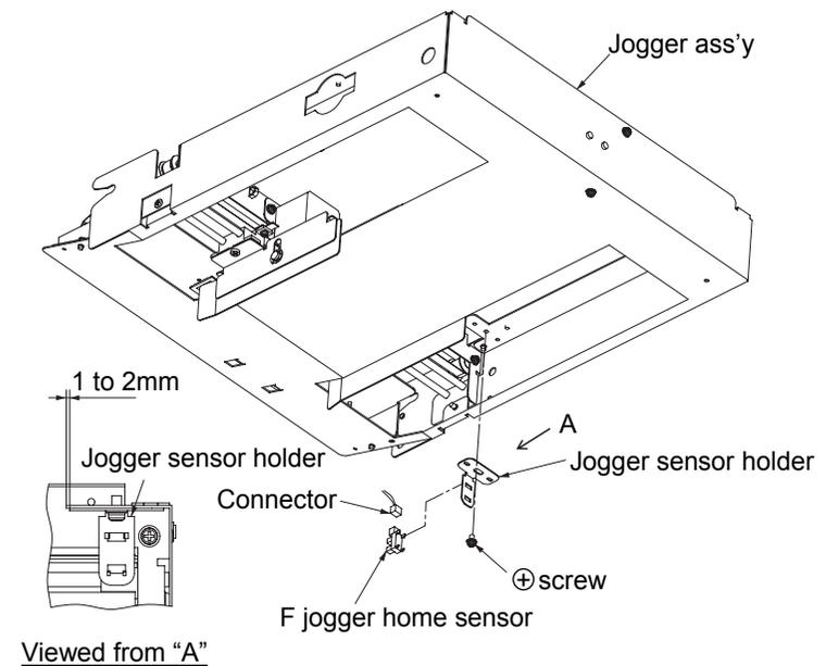
Fig. 6-4. Removal of the F jogger home sensor U/L
