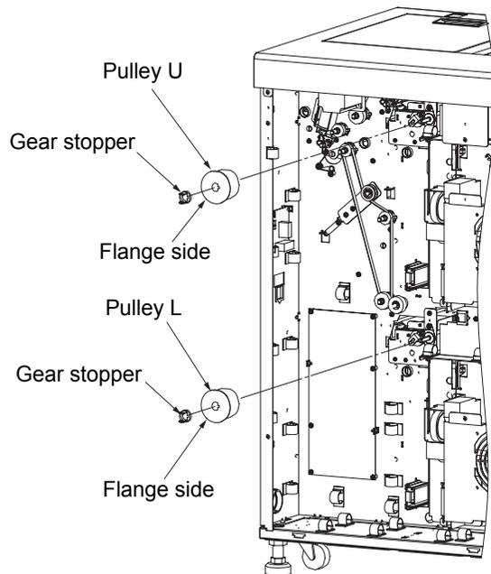
Fig. 6-76. Removal of the pulley U/L
