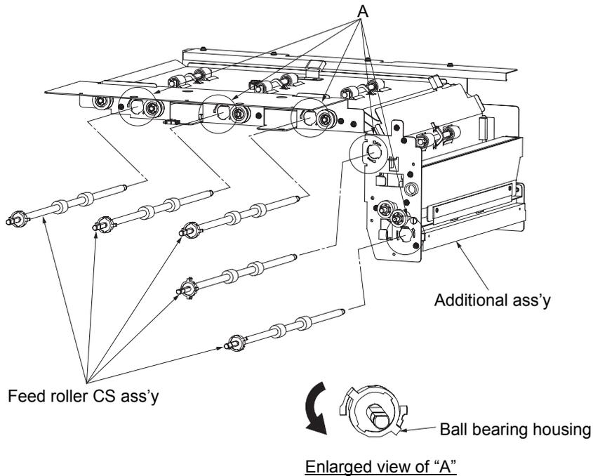
Fig. 6-115. Removal of the feed roller CS ass'y
