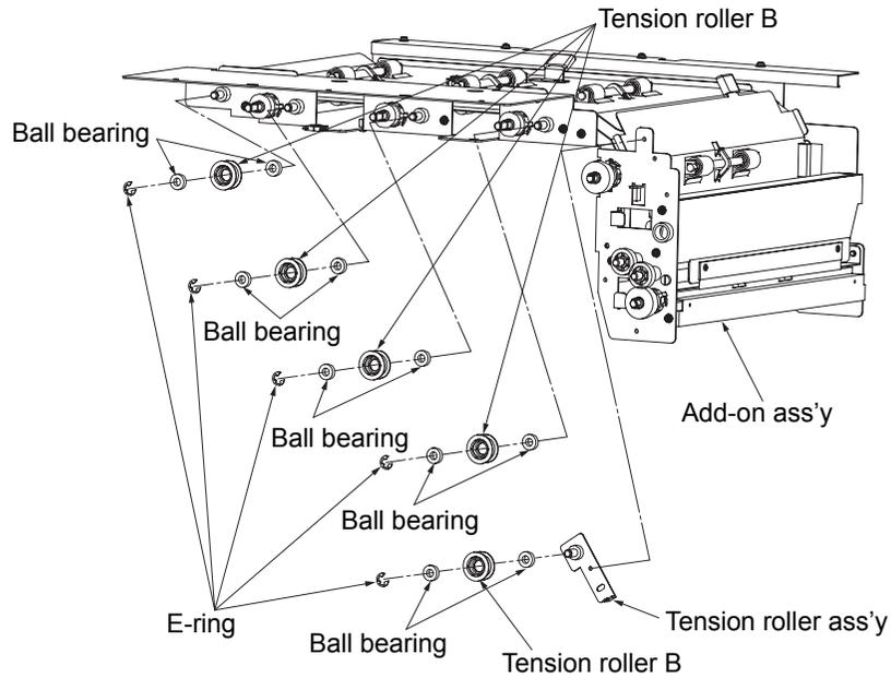
Fig. 6-113. Removal of the tension roller B and the ball bearing
