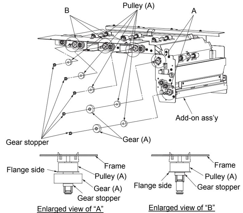
Fig. 6-114. Removal of the pulley (A)
