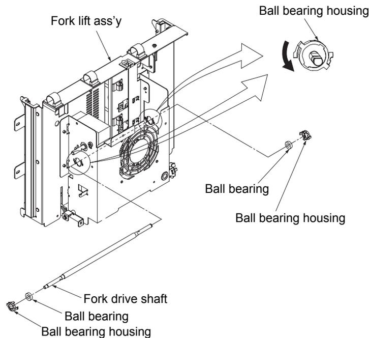
Fig. 6-37. Removal of the ball bearing housing and the ball bearing U/L
