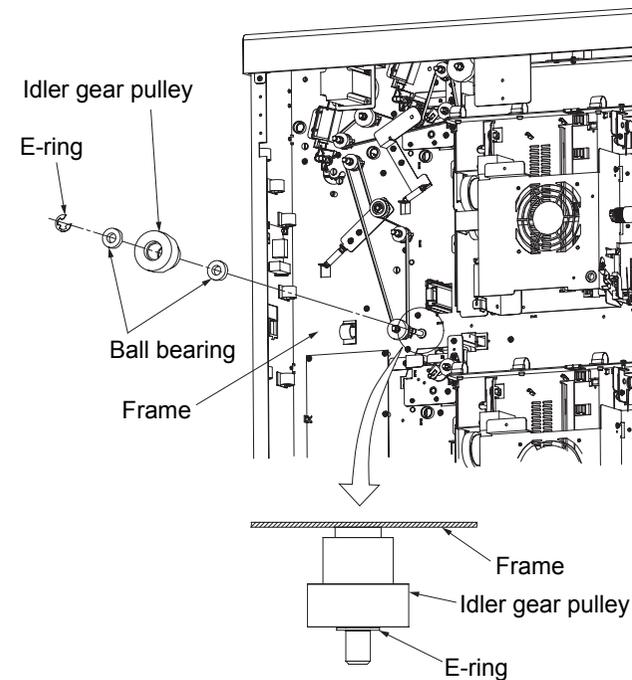
Fig. 6-56. Removal of the idler gear pulley and the ball bearing
