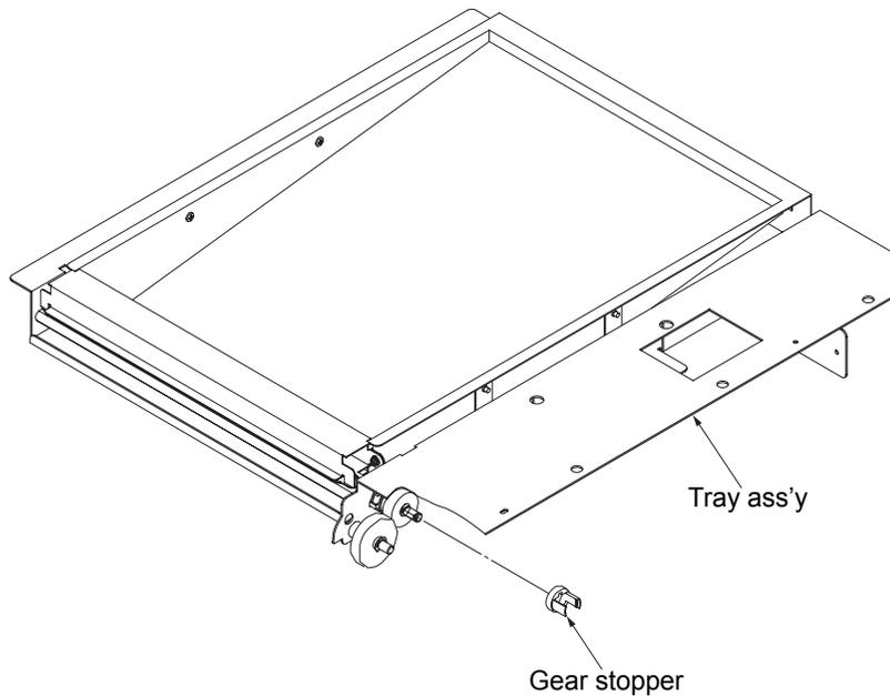
Fig. 6-92. Removal of the gear stopper
