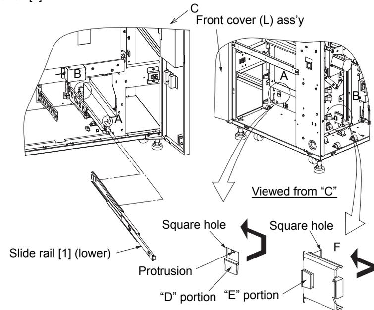
Fig. 6-134. Removal of the slide rail [1] (lower)
