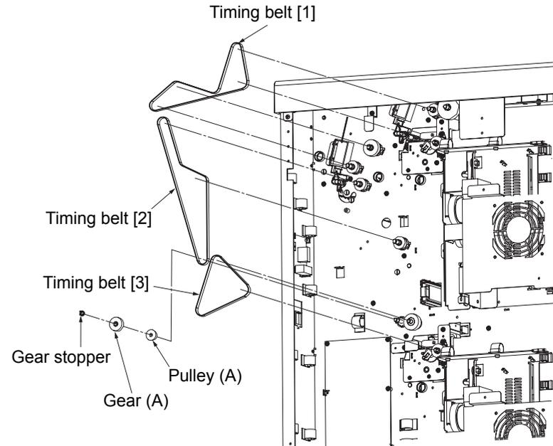
Fig. 6-54. Removal of the timing belts [1], [2] and [3]
