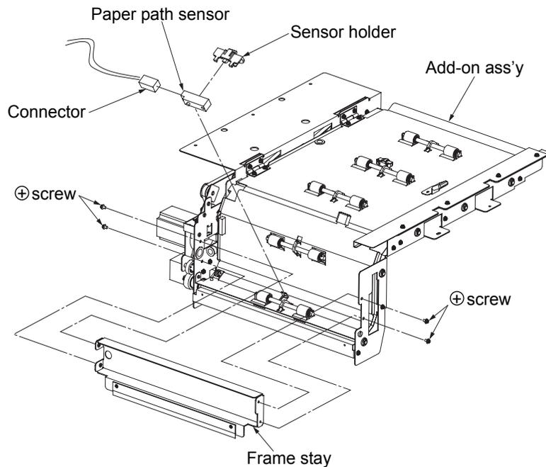
Fig. 6-99. Removal of the paper path sensor (discharging side) and the sensor holder
