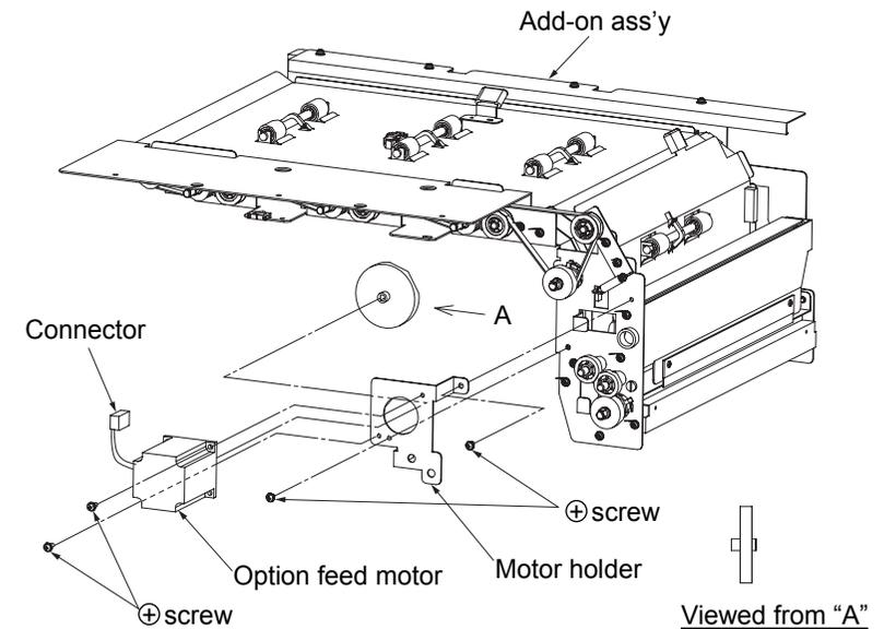
Fig. 6-108. Removal of the option feed motor and the SB motor gear
