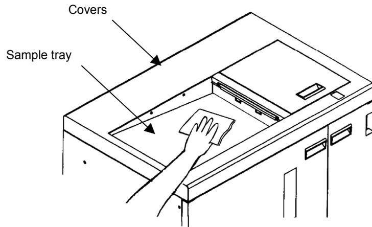
Fig. 4-2. Cleaning of covers and sample tray
