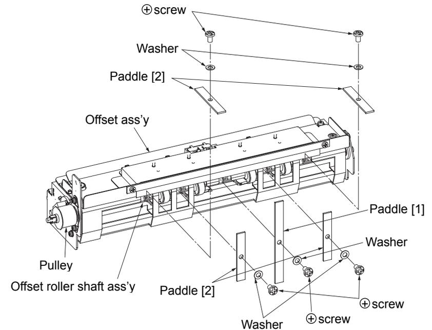
Fig. 6-79. Removal of the paddle [1] [2] U/L
