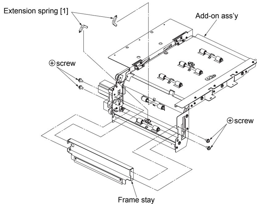
Fig. 6-103. Removal of the extension spring [1] (discharging side)
