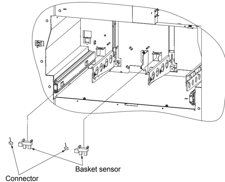
Fig. 6-126. Removal of the basket sensor U/L
