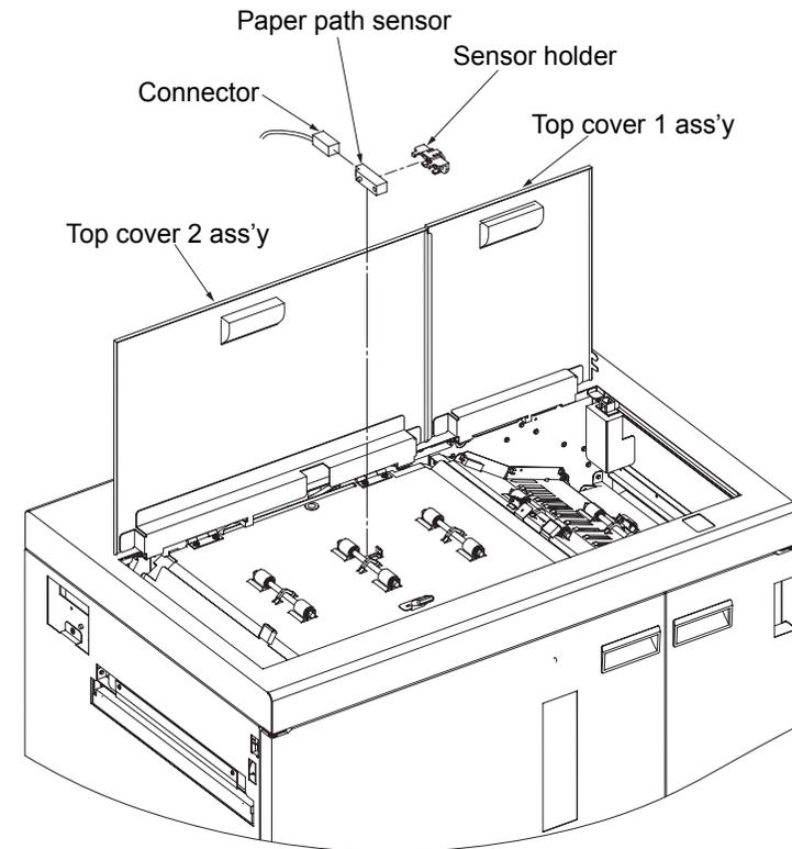
Fig. 6-98. Removal of the paper path sensor (upper) and the sensor holder
