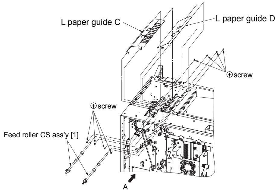
Fig. 6-65. Removal of the feed roller CS ass'y [1] (upper)
