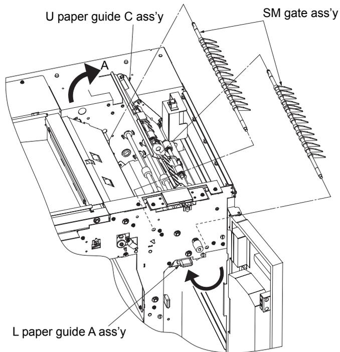
Fig. 6-73. Removal of the SM gate ass'y
