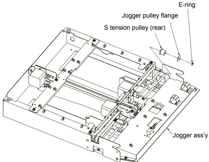
Fig. 6-15. Removal of the S tension pulley (rear) U/L
