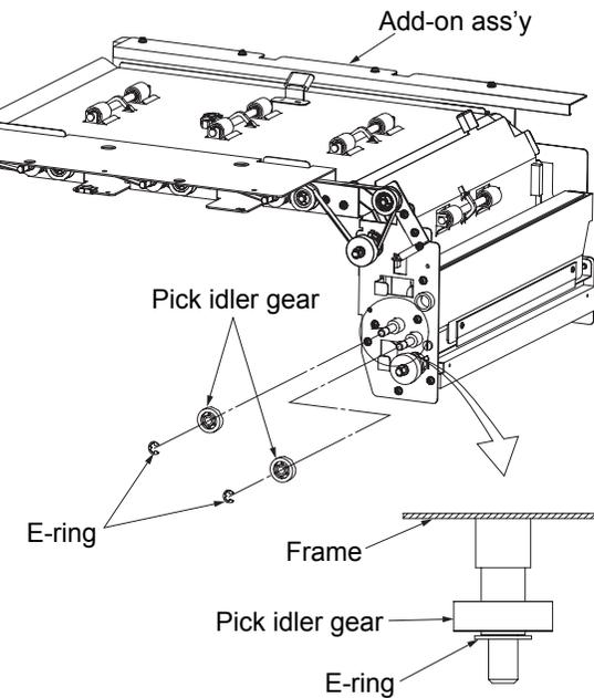
Fig. 6-110. Removal of the pick idler gear
