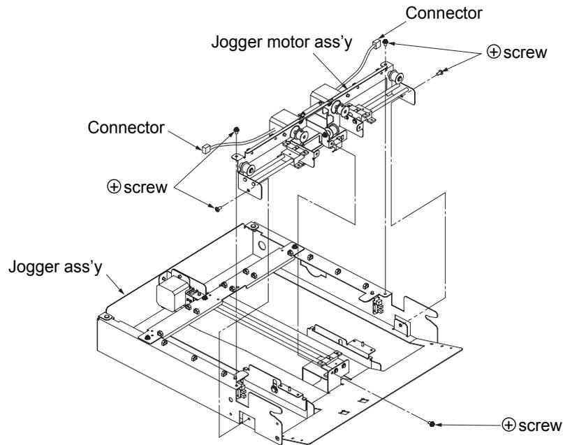
Fig. 6-17. Removal of the linear sleeve (front) U/L
