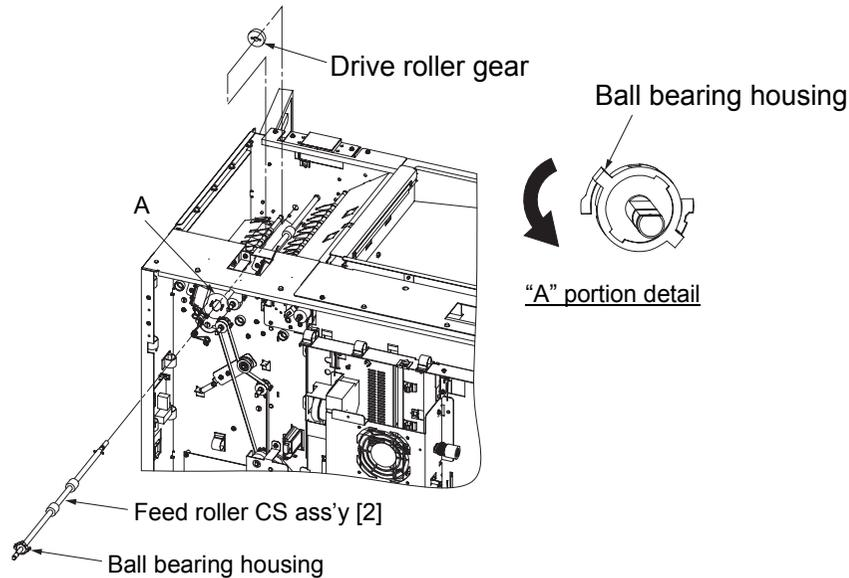
Fig. 6-67. Removal of the feed roller CS ass'y [2] and the drive roller gear
