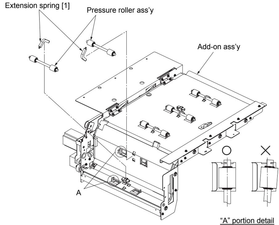
Fig. 6-104. Removal of the pressure roller ass'y (discharging side)
