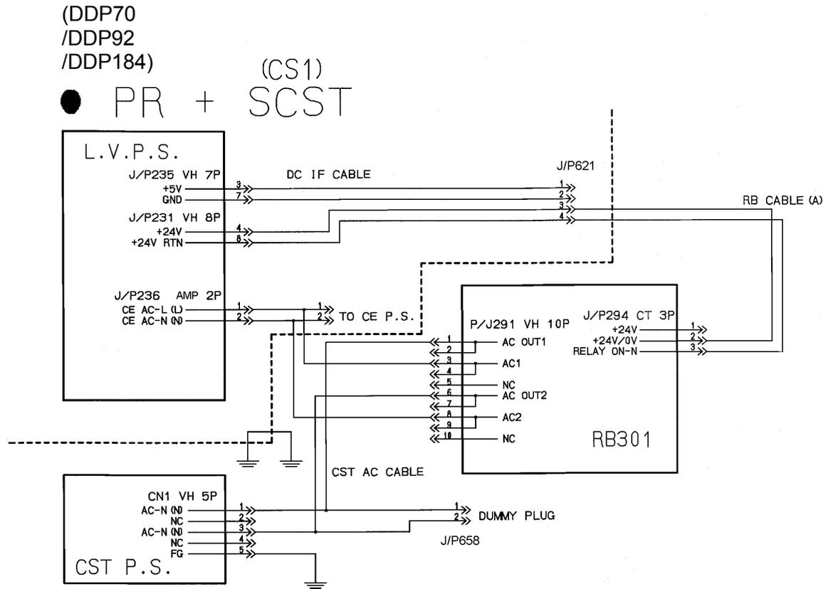
Figure 3-10 Block Wiring
