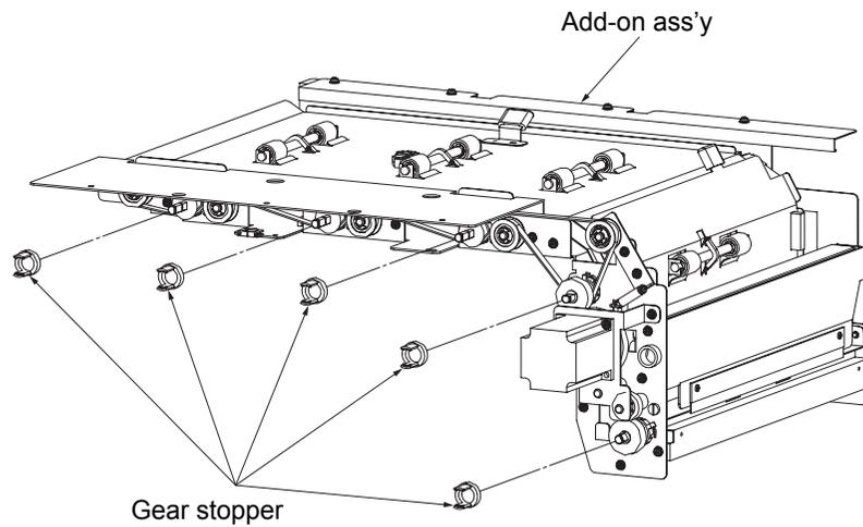
Fig. 6-107. Removal of the gear stopper
