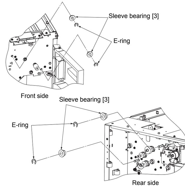
Fig. 6-72. Removal of the sleeve bearing [3]
