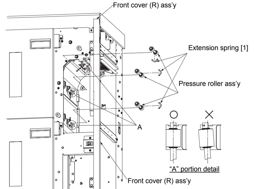
Fig. 6-42. Removal of the pressure roller ass'y (lower)
