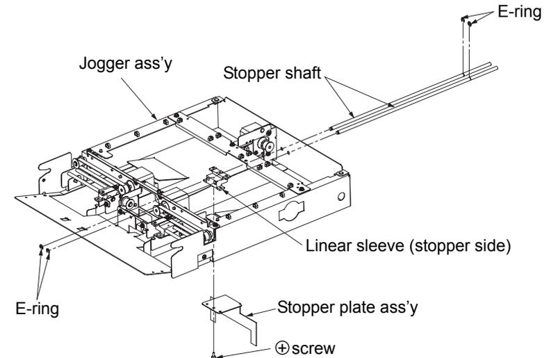
Fig. 6-16. Removal of the linear sleeve (stopper side) U/L
