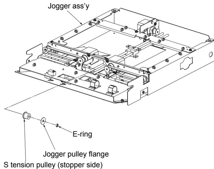
Fig. 6-13. Removal of the S tension pulley (stopper side) U/L
