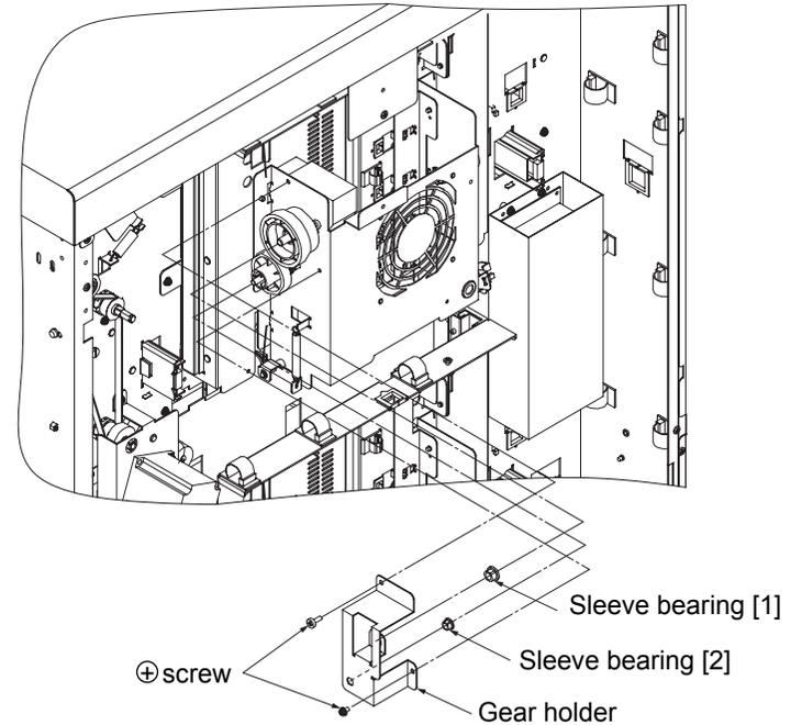
Fig. 6-28. Removal of the sleeve bearings [1] and [2] U/L
