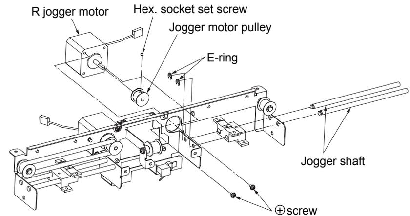
Fig. 6-22. Removal of the R jogger motor U/L
