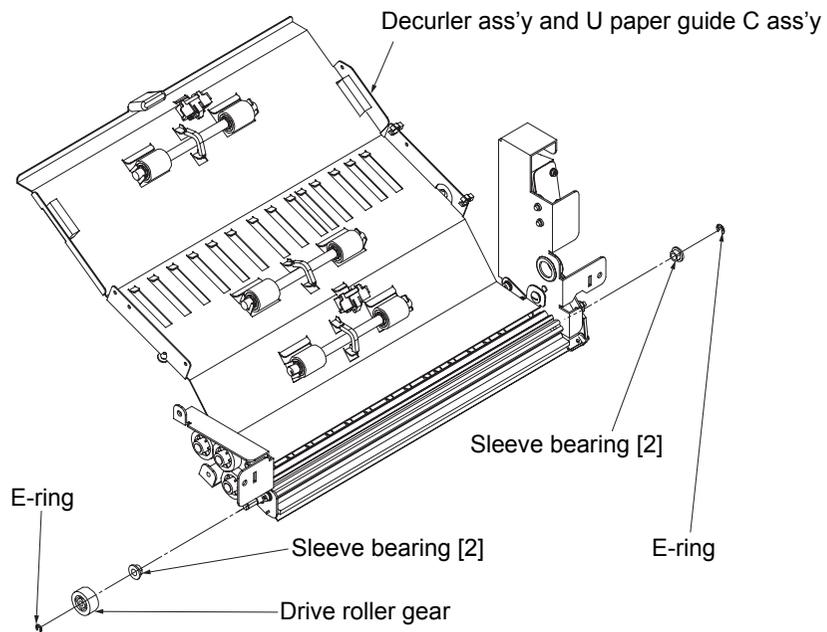
Fig. 6-63. Removal of the sleeve bearing [2]
