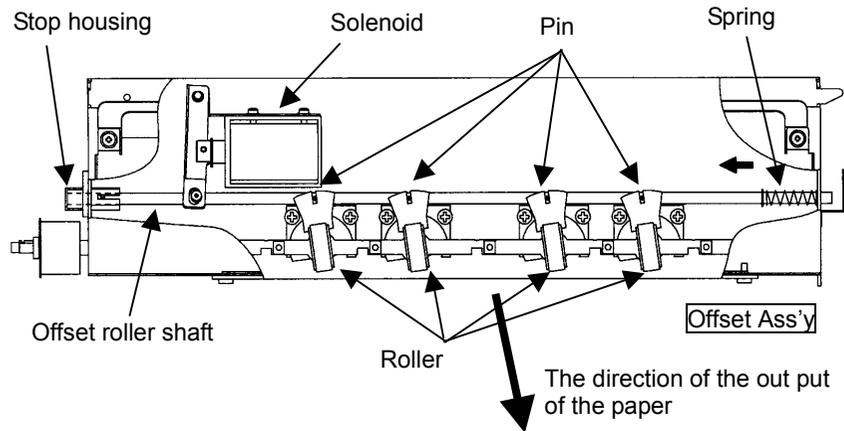
Fig 8-14 Out put a paper to the OP side
