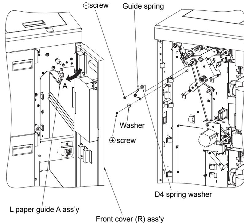
Fig. 6-138. Removal of the guide spring
