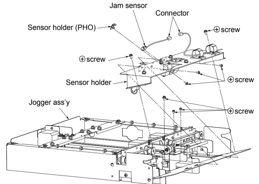
Fig. 6-8. Removal of the jam sensor U/L
