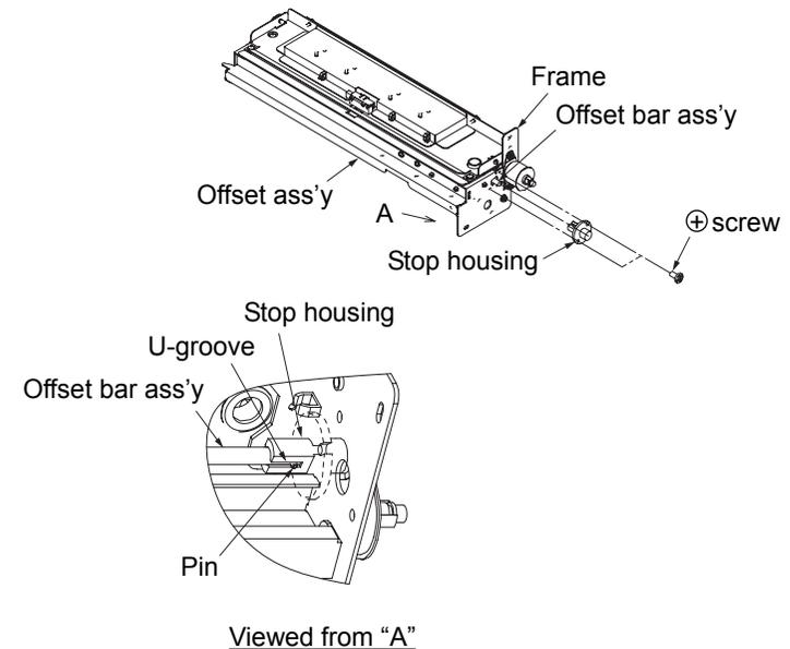
Fig. 6-77. Removal of the stop housing U/L
