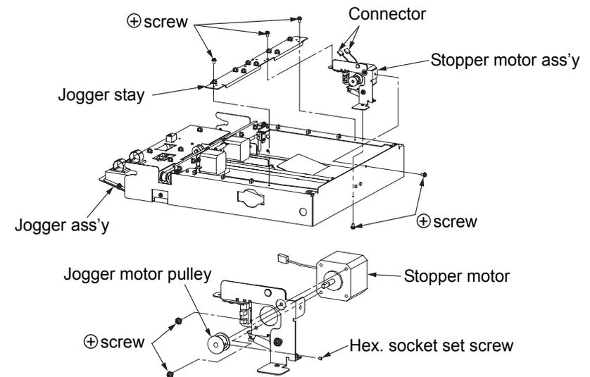
Fig. 6-20. Removal of the stopper motor U/L
