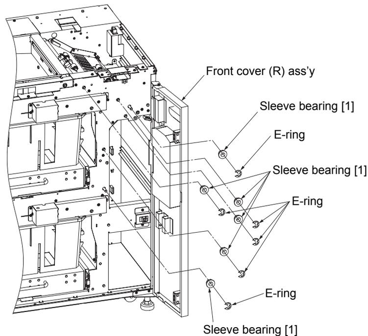
Fig. 6-47. Removal of the sleeve bearing [1]
