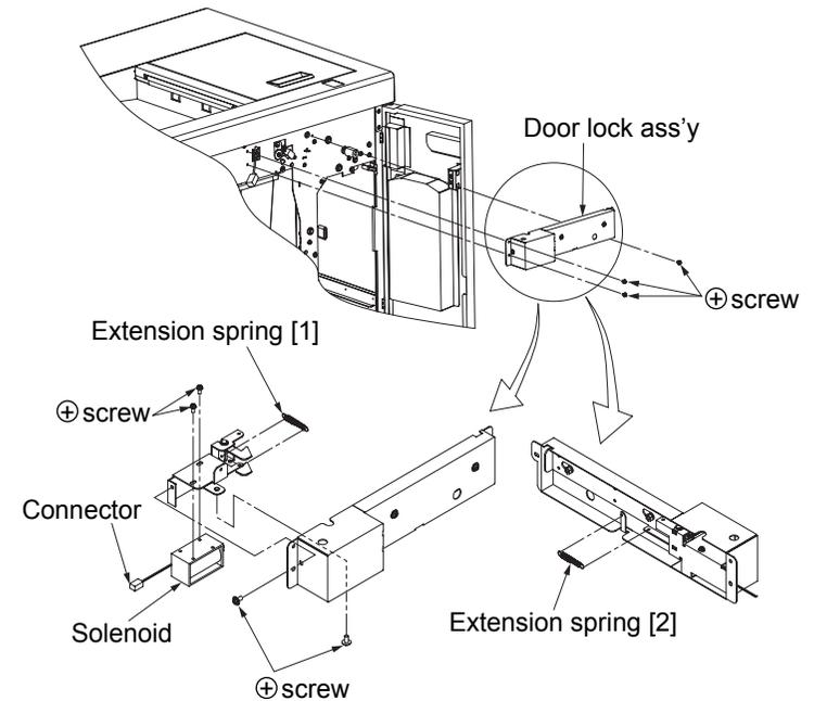
Fig. 6-128. Removal of the solenoid and the extension springs [1] and [2]
