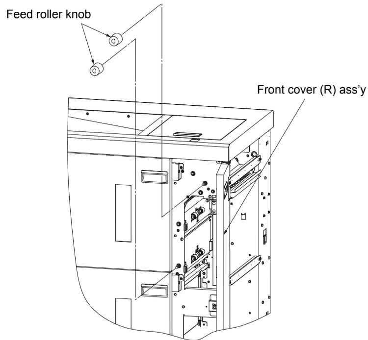
Fig. 6-45. Removal of the feed roller knob
