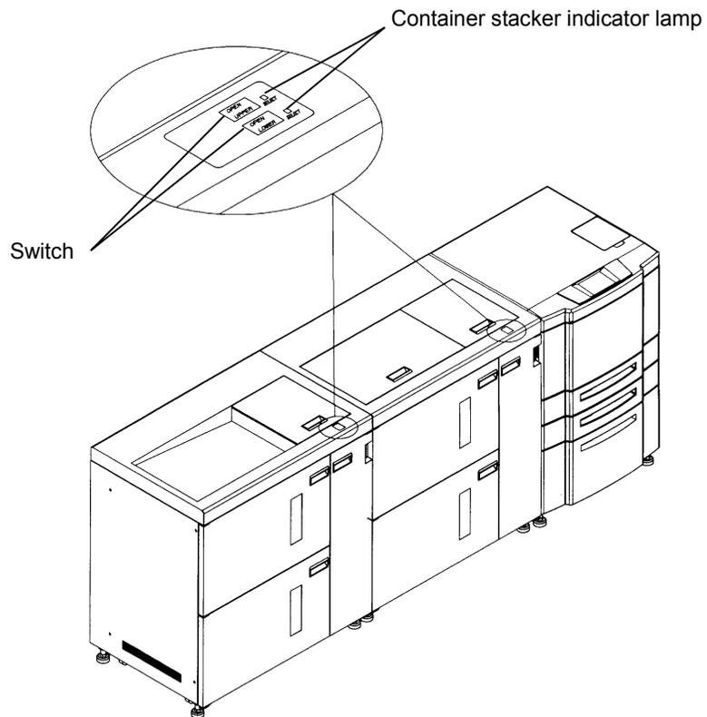
Fig. 3-4. Switch and indicator lamp locations
