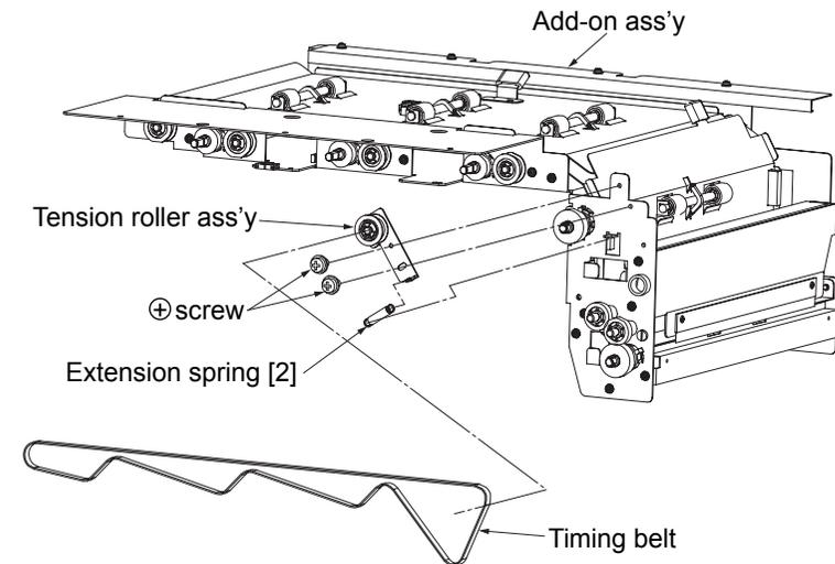
Fig. 6-112. Removal of the timing belt
