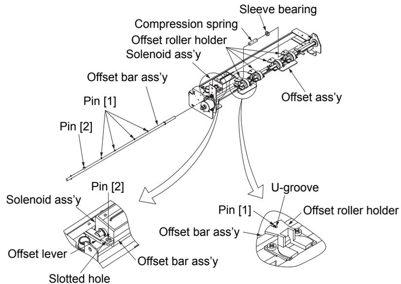
Fig. 6-86. Removal of the sleeve bearing and the compression spring [2] U/L
