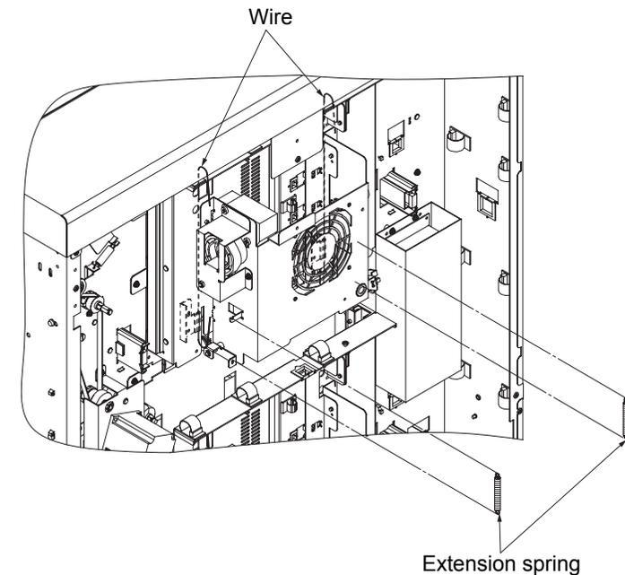
Fig. 6-38. Removal of the extension spring U/L
