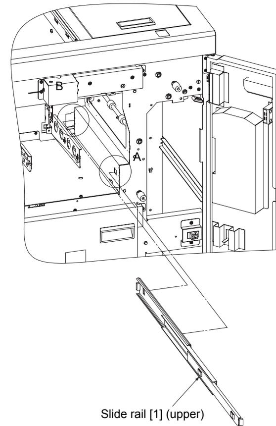
Fig. 6-136. Removal of the slide rail [1] (upper)
