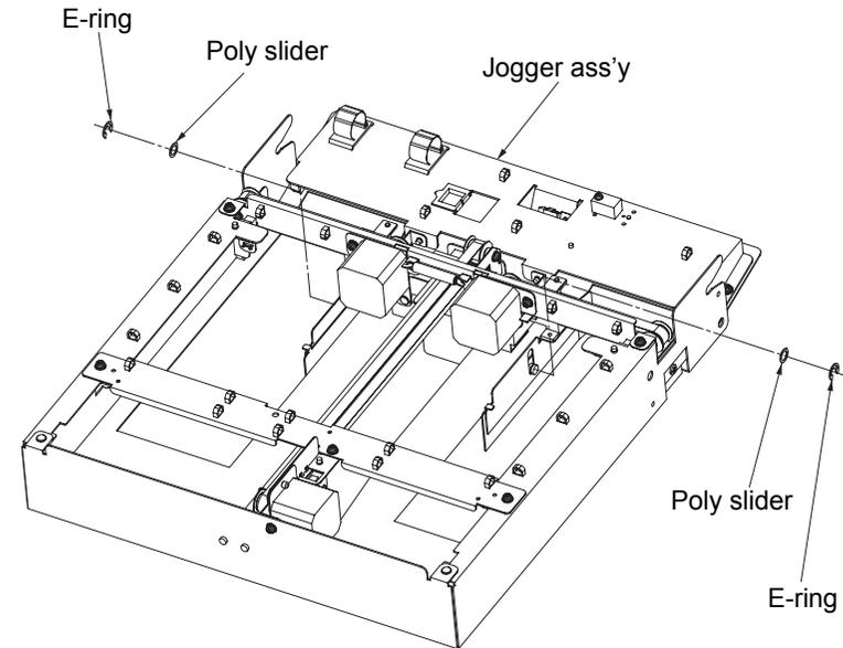
Fig. 6-6. Removal of the poly slider U/L
