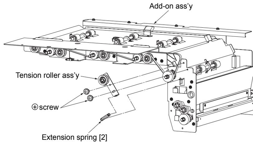
Fig. 6-111. Removal of the extension spring [2]
