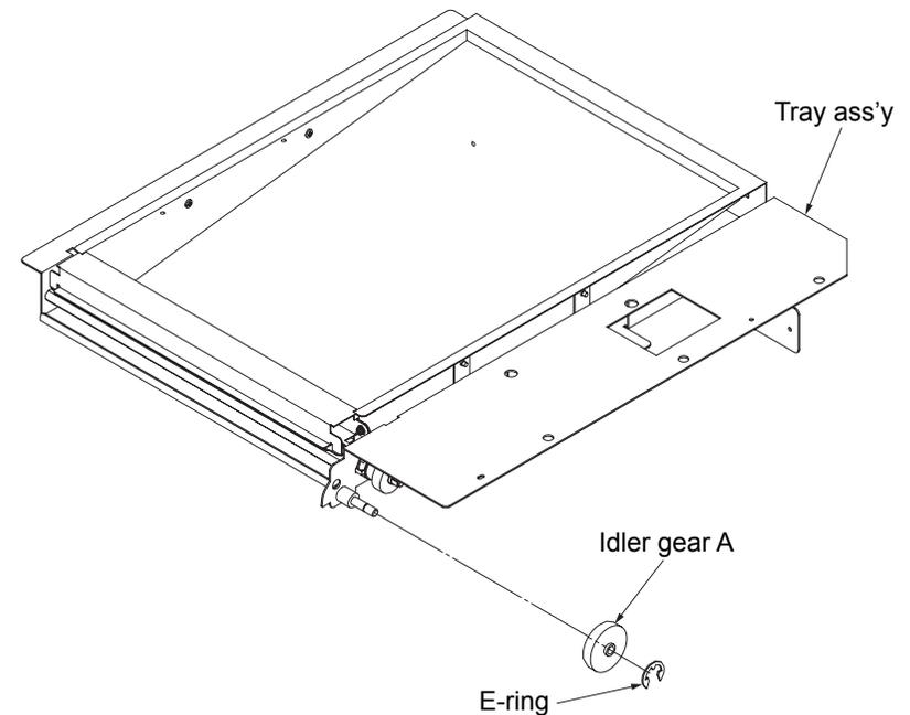
Fig. 6-91. Removal of the idler gear A
