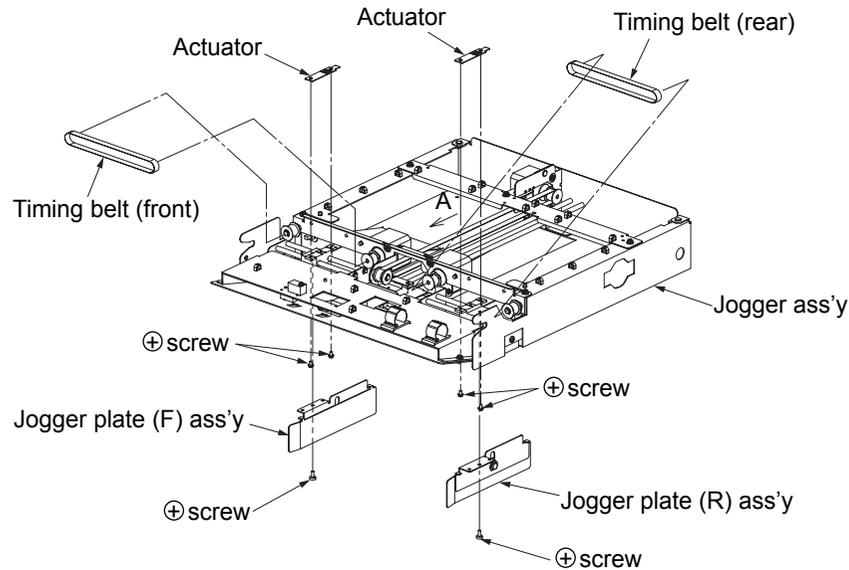
Fig. 6-11. Removal of the timing belt (front/rear) U/L
