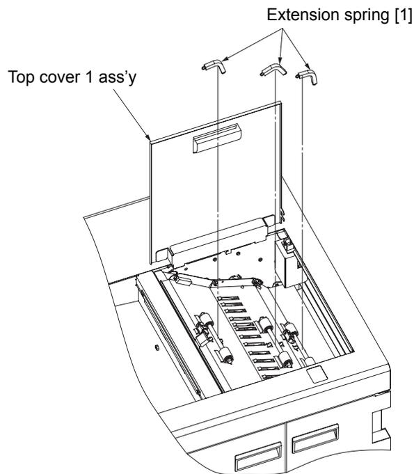
Fig. 6-39. Removal of the extension spring [1] (upper)
