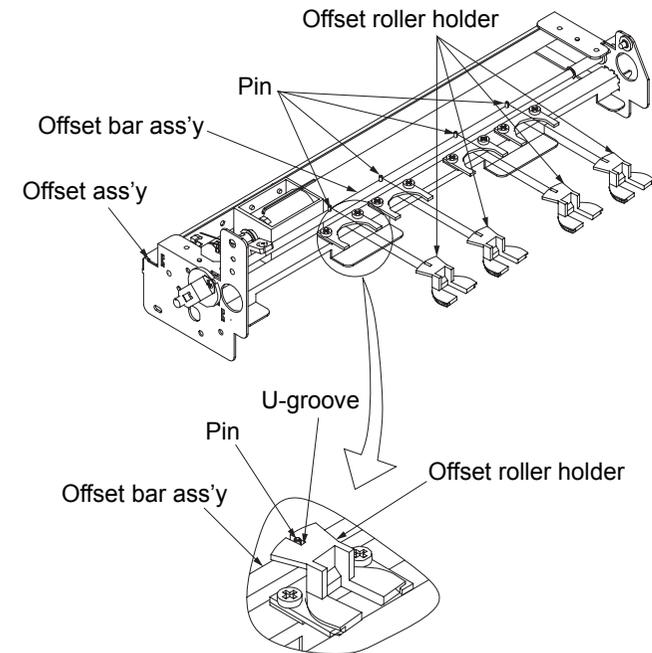
Fig. 6-85. Removal of the offset roller holder U/L
