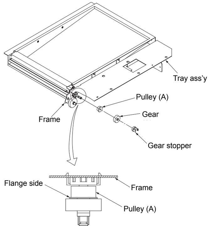
Fig. 6-94. Removal of the pulley (A)
