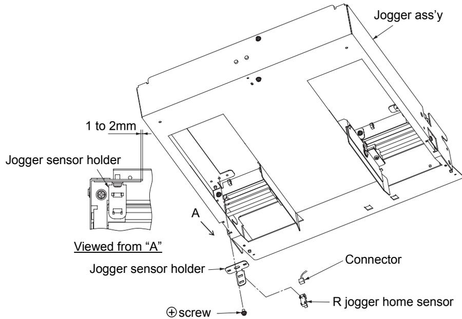
Fig. 6-5. Removal of the R jogger home sensor U/L
