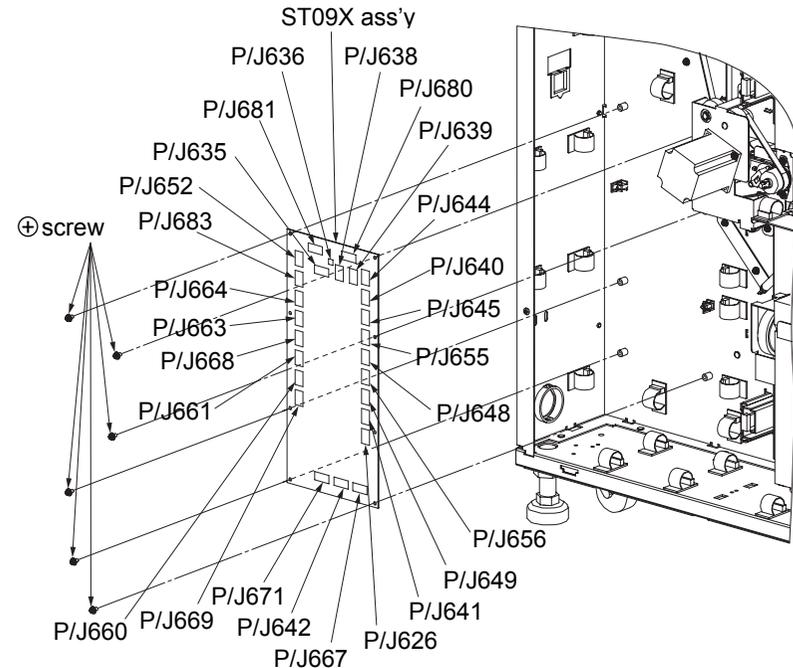
Fig. 6-120. Removal of the ST09X ass'y
