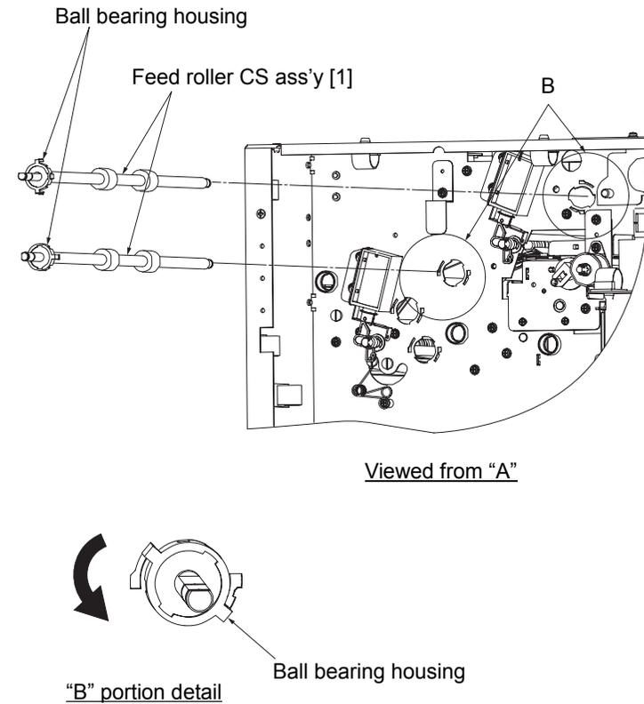
Fig. 6-66. Removal of the feed roller CS ass'y [1] (upper)
