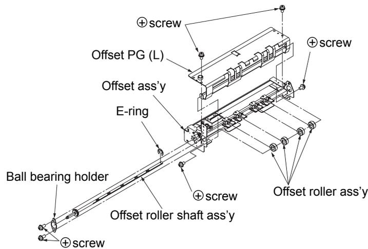
Fig. 6-84. Removal of the offset roller ass'y and offset roller shaft ass'y U/L
