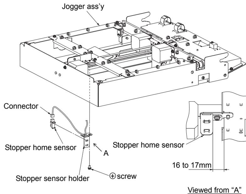
Fig. 6-3. Removal of the stopper home sensor U/L
