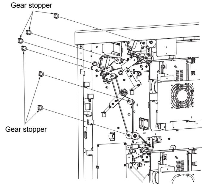
Fig. 6-50. Removal of the gear stopper
