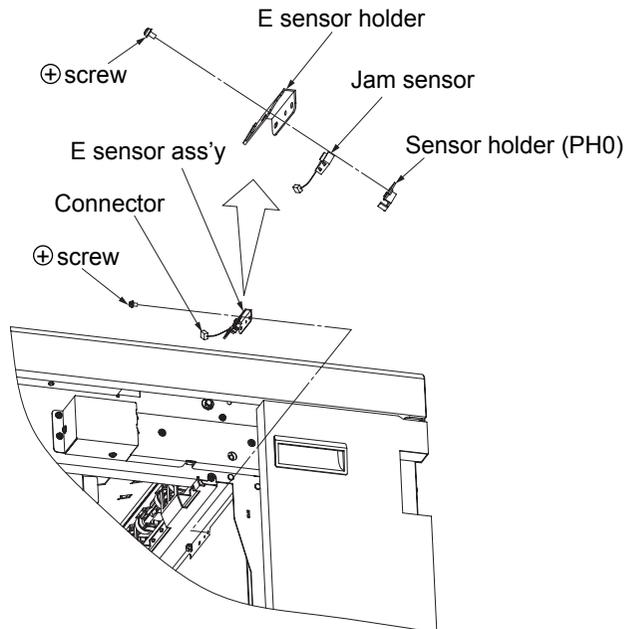
Fig. 6-123. Removal of the jam sensor U/L
