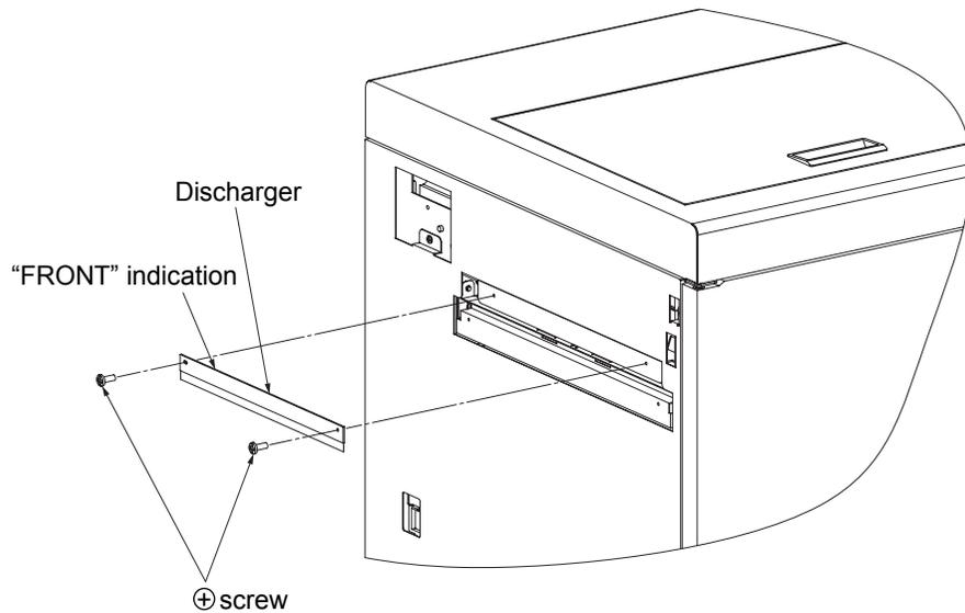
Fig. 6-105. Removal of the discharger
