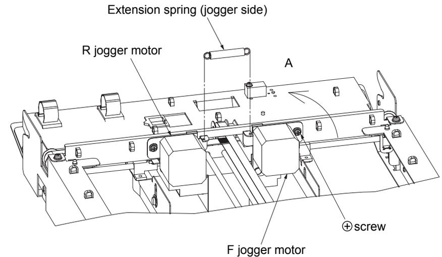
Fig. 6-24. Removal of the extension spring (jogger side) U/L
