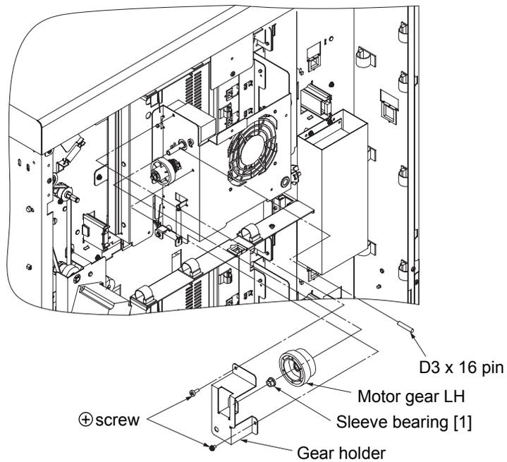
Fig. 6-29. Removal of the motor gear LH U/L
