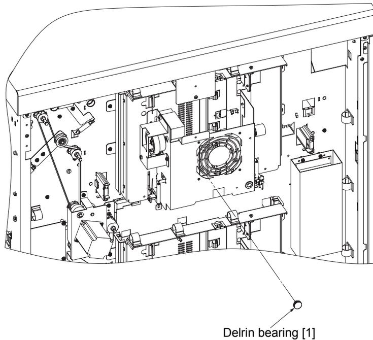
Fig. 6-27. Removal of the Delrin bearing [1] U/L
