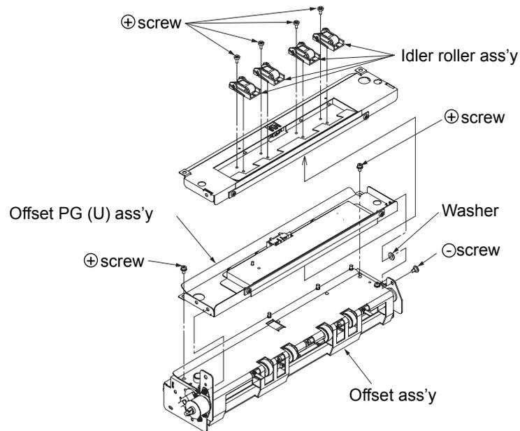
Fig. 6-82. Removal of the idler roller ass'y U/L
