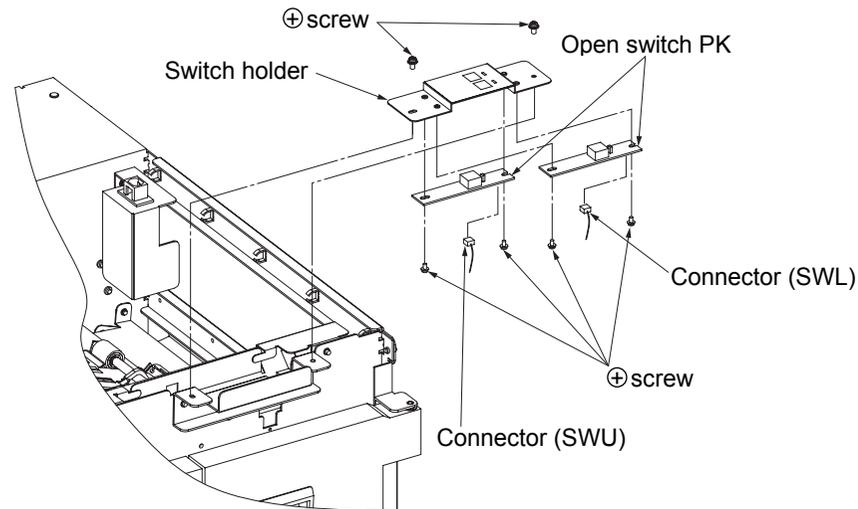
Fig. 6-121. Removal of the open switch PK (SW96X ass'y)
