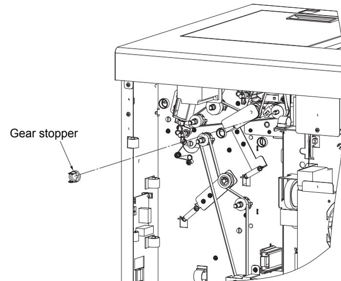
Fig. 6-75. Removal of the gear stopper U/L
