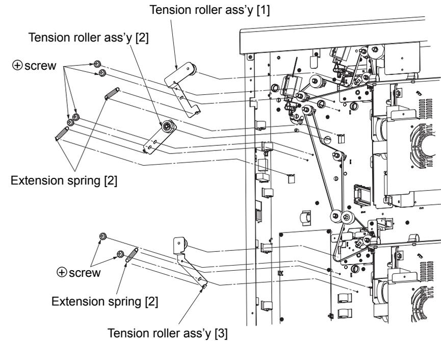
Fig. 6-52. Removal of the extension spring [2]
