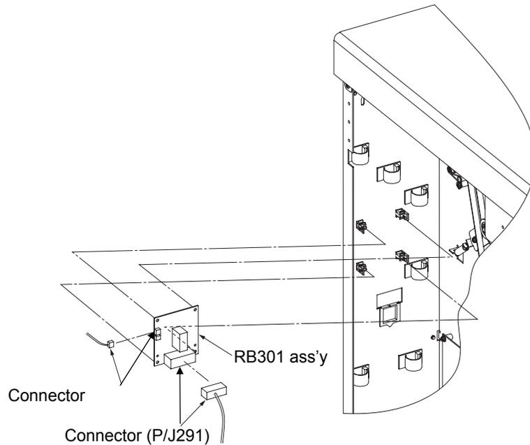
Fig. 6-129. Removal of the RB301 ass'y
