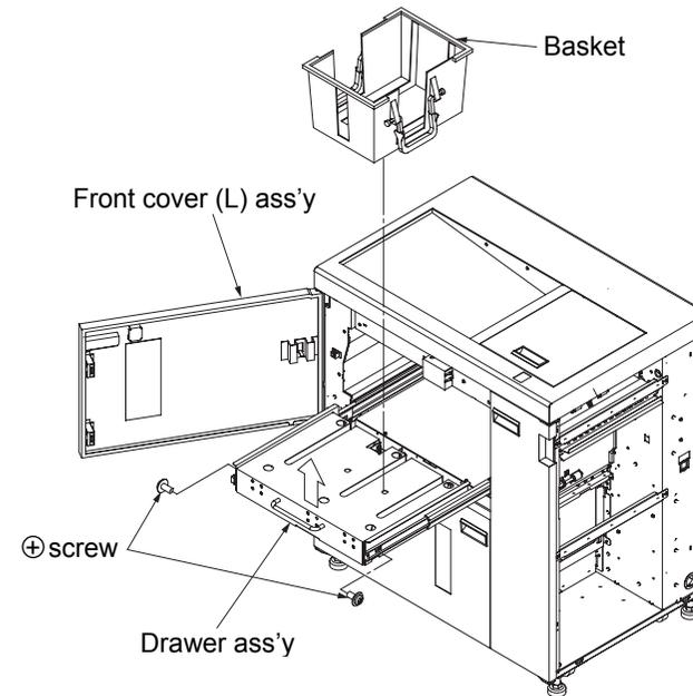
Fig. 6-116. Removal of the drawer ass'y U/L
