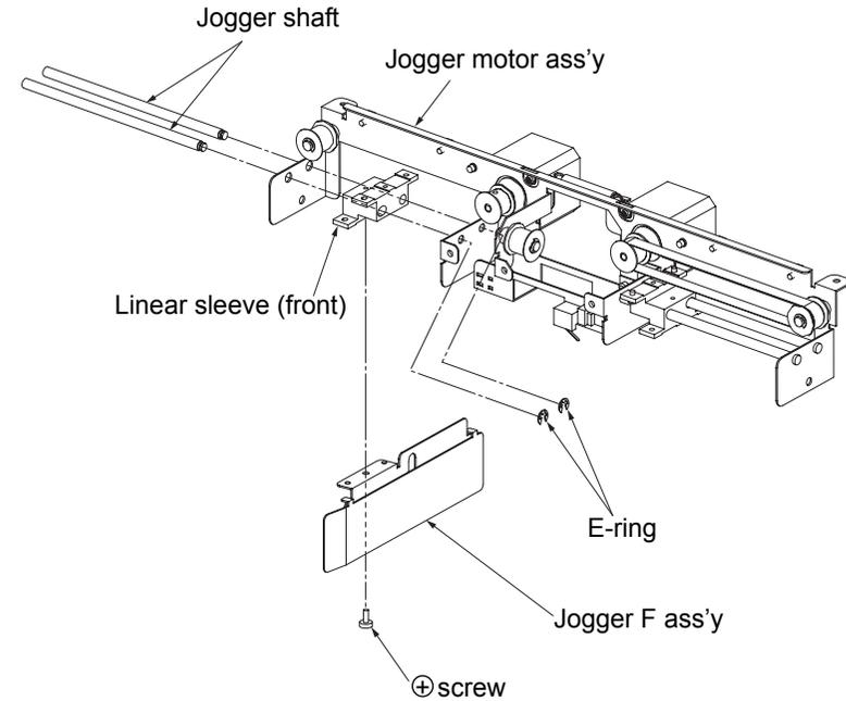
Fig. 6-18. Removal of the linear sleeve (front) U/L
