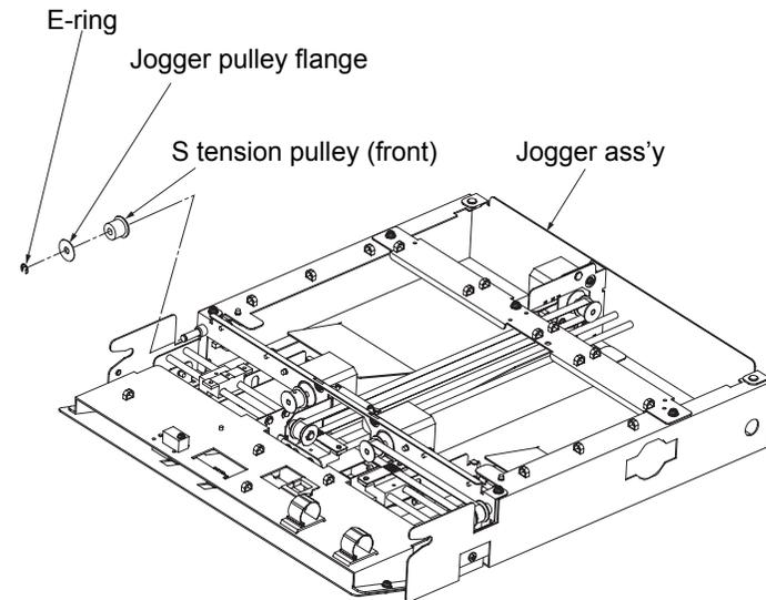
Fig. 6-14. Removal of the S tension pulley (front) U/L
