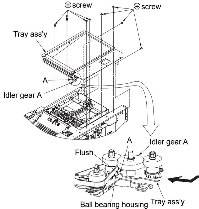
Fig. 6-88. Removal of the tray ass'y
