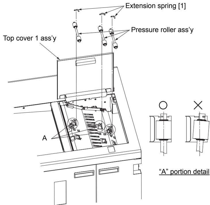
Fig. 6-41. Removal of the pressure roller ass'y (upper)
