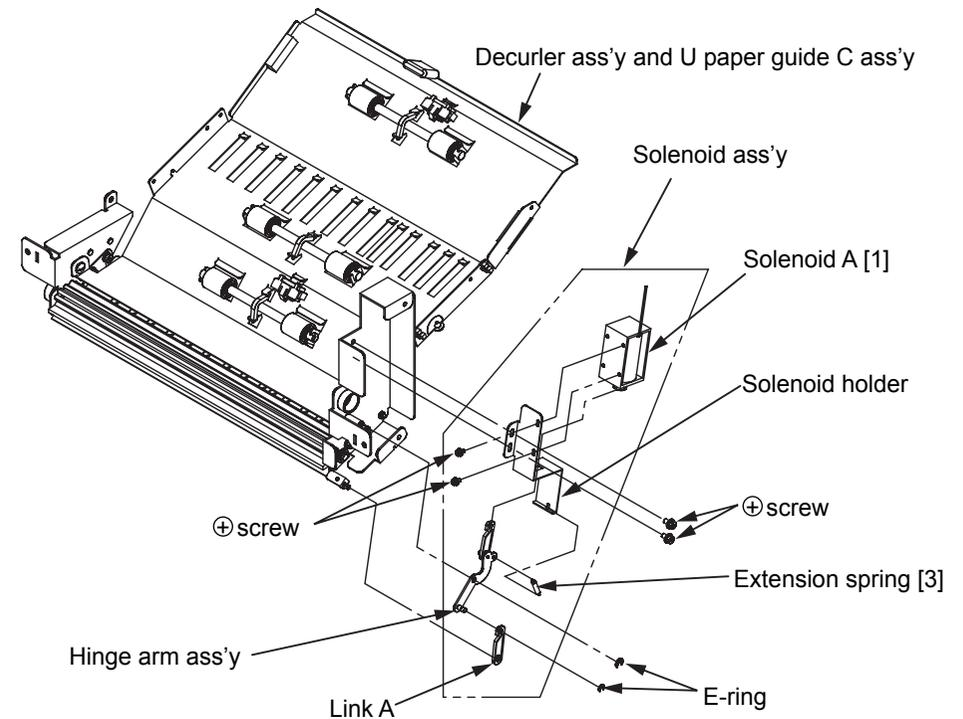
Fig. 6-60 Removal of the solenoid A [1]
