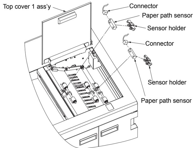
Fig. 6-43. Removal of the paper path sensor (upper) and the sensor holder
