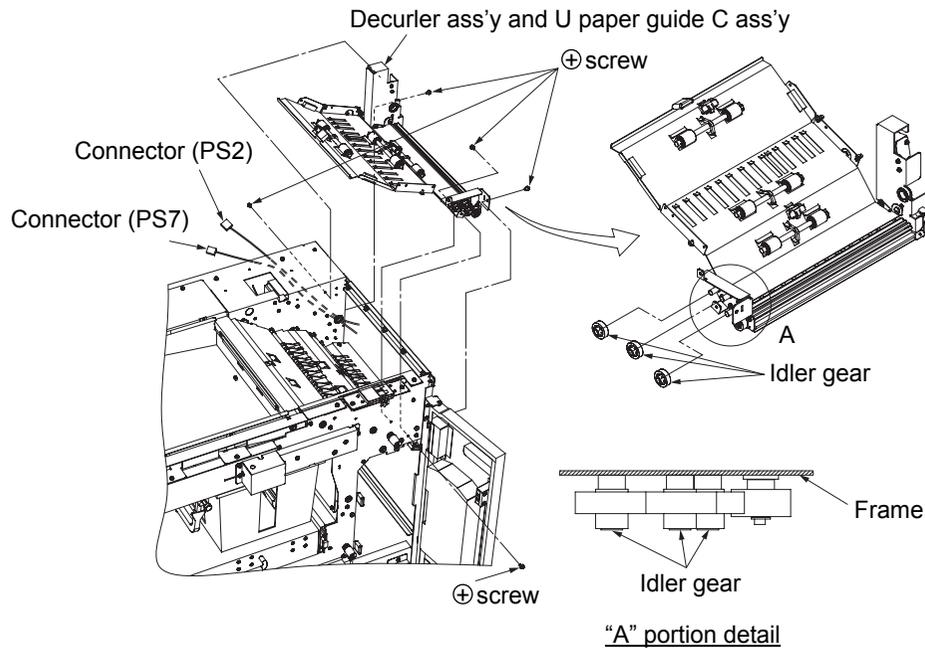
Fig. 6-57 Removal of the idler gear
