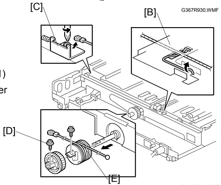
**Reassembling the Rear Scanner Wire**
