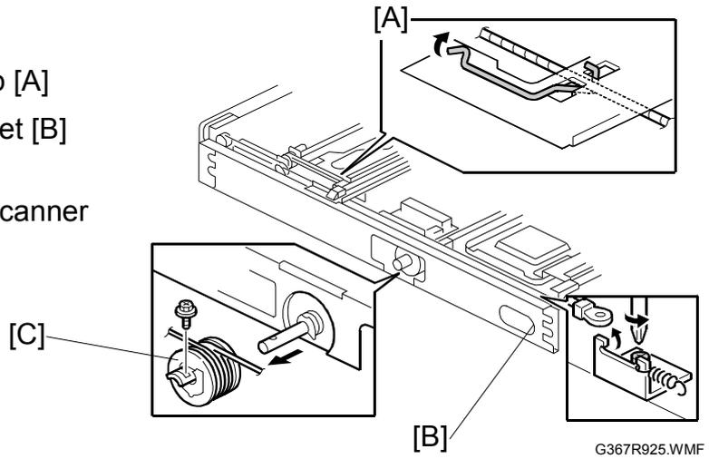
**Reassembling the Front Scanner Wire**
