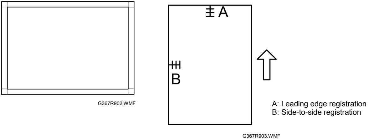
Make a temporary test chart as shown above using A3/DLT paper.
