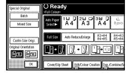
Enter the horizontal size of the original with the Number keys, and then press [#].
